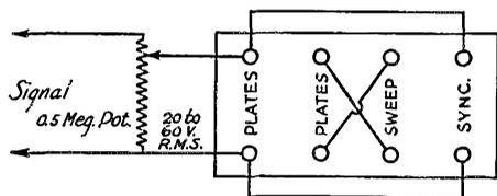
FIG. 4—CONNECTIONS FOR OBSERVING AN AUDIO-FREQUENCY SIGNAL VOLTAGE
