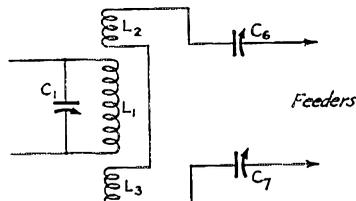
FIG. 2—ANTENNA COUPLING FOR ZEPPE FEEDERS
