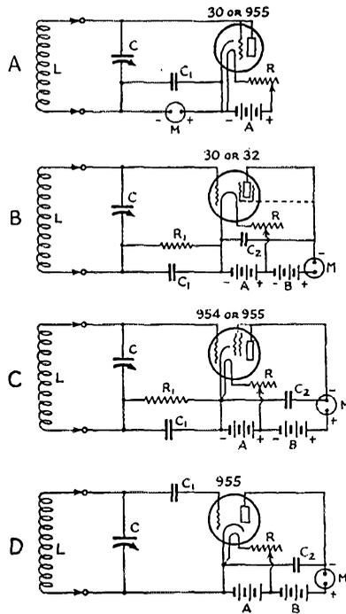
deflection to 50 microamperes from initial value. This holds the grid condenser discharge time within reasonable limits. The detector thus arranged is so sensitive that it may be necessary to keep one or two hundred feet from the transmitter and antenna when tuning to resonance with the fundamental frequency. A 30-microampere deflection occurred, for instance, 15 feet from the oscillator alone at WIES.
