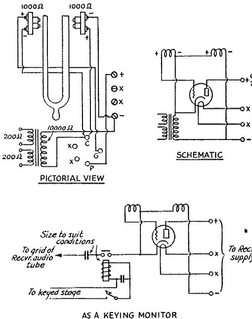
FIG. 1—CIRCUIT DETAILS OF THE TONE GENERATOR
