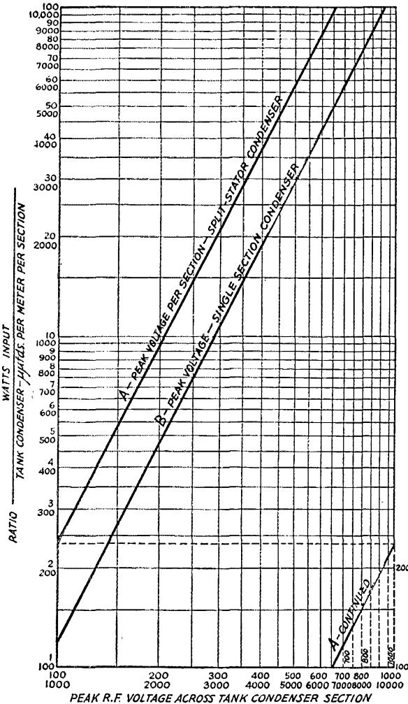
DETERMINING CONDENSER PEAK VOLTAGE
