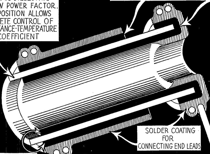
SOLDER COATING FOR CONNECTING END LEADS
