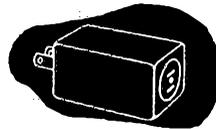
Manufacturers of low power lamp and electric razor equipment needed a step-down transformer to permit the operation of 110 V. units on 220 V. lines. Ordinary units were bulky. UTC developed an item with the transformer built into the line cord plug.
