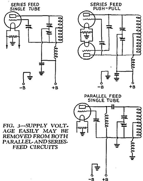
FIG. 3—SUPPLY VOLTAGE EASILY MAY BE REMOVED FROM BOTH PARALLEL AND SERIES FEED CIRCUITS
