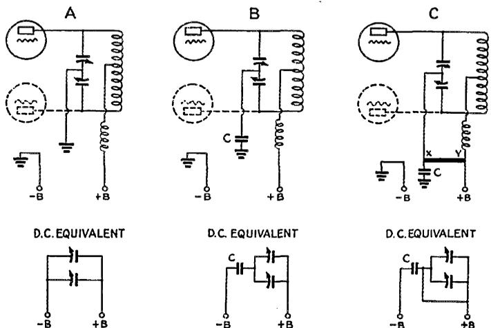
WITH TUNING CONDENSER CONNECTED AS IN A OR B OF FIG. 1
