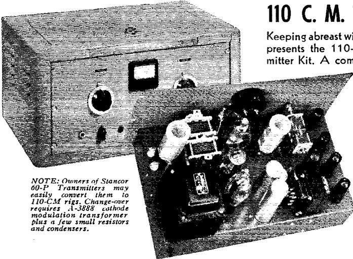
*NOTE: Owners of Stancor 60-P Transmitters may easily convert them to 110-CM rigs. Change-over requires A-3888 cathode modulation transformer plus a few small resistors and condensers.*
