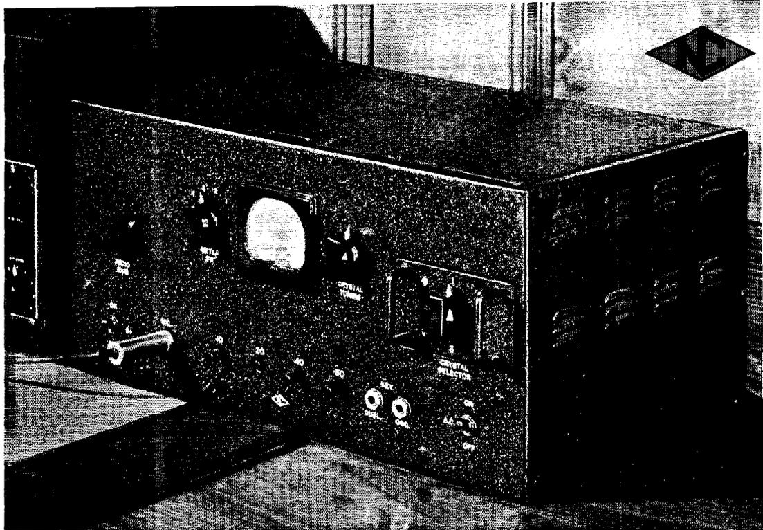
**E**ITHER of the fine units shown on this page contributes generously to the art of fine operating. The NTE Exciter-Speech Amplifier shown above is the heart of a fine transmitter, combining a crystal controlled multi-band exciter with a high fidelity 10-watt speech amplifier. The NTX-30 below is a complete CW transmitter in itself, with 30 watts output, conservatively rated. Terminals are provided for connecting an external amplifier for phone operation.
