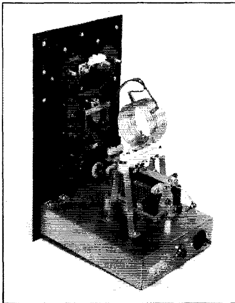
Rear view of the antenna coupler. Connections to the coax link, to the receiver antenna posts, and to the 115-volt supply for the relay are through sockets on the rear edge of the chassis.
