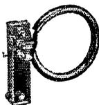
These links are made to fit RLS, VLS, and MLS series of coils. This link will prevent capacity coupling between the tank coil and the link and would reduce TVI by greatly attenuating harmonics. The links can be used on co-ax or balanced lines.
