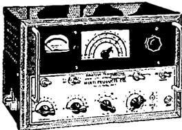
VFO or Crystal control. Direct-reading. VFO on all bands—75, 20, 11, 10. • Plate modulation • Completely band-switching, fone or CW. • 50 Watts max. input. Power required: 300-500 V.D.C. at 250 ma., 6.3 V AC or DC at 4.5A. • Uses 3-6AG5, 6AR5, 6C4, 12AU7, 2-6L6G, 807, (included). • Only 7 1/2" x 7 1/2" x 12", 14 1/2 lbs.
