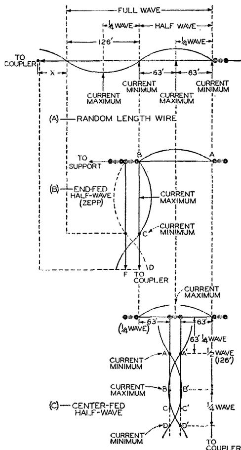
Fig. 1 — Current distribution in three different types of antenna. Note the way the current patterns repeat themselves, but in the opposite polarity, throughout alternate half waves. The dimensions shown are those computed for half-wave antennas operating at 3725 kc., the center of the present Novice assignment in the 3.5-Mc. amateur band.
