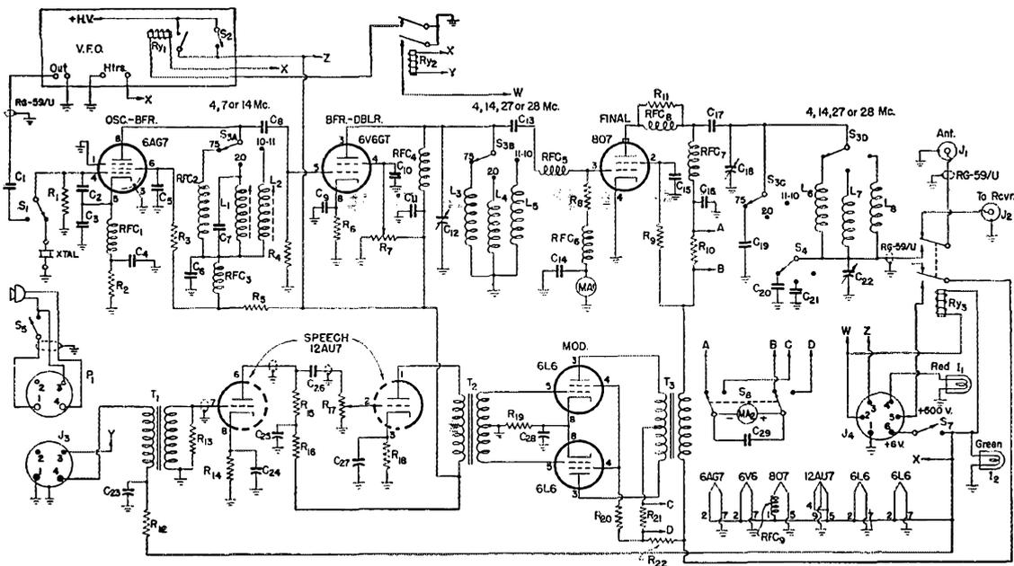
Fig. 1 — Circuit diagram of the quadriband mobile transmitter.
