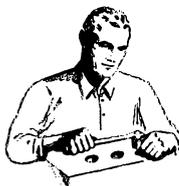
Save hours of hard, tedious work . . . cut accurate holes in chassis for sockets, plugs, controls, meters, panel lights, etc. with GREENLEE Punches. In 1-1/2 minutes or less make a smooth hole in metal, bakelite or hard rubber up to 1/16" thick. Easy to operate. Simply turn with
