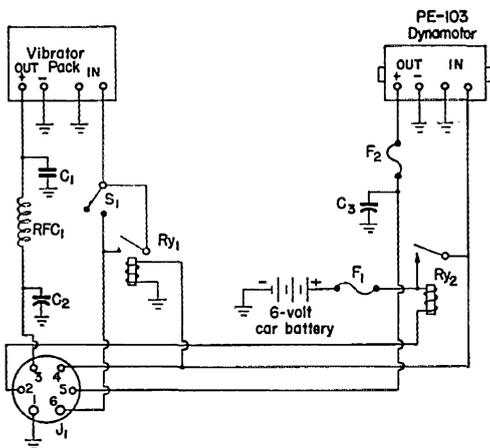
Fig. 2—Power circuits of the quadriband mobile transmitter.
