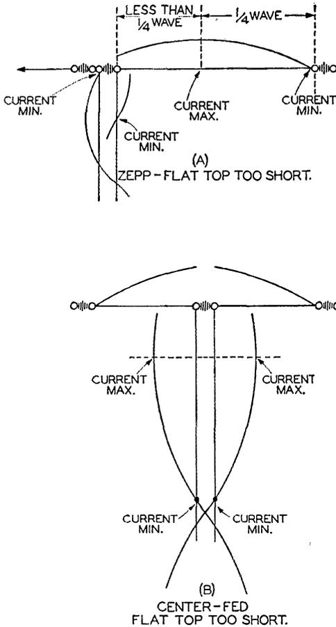
Fig. 2 — Current distribution in antennas having less than a half wavelength in the "flat-top." In the case of the Zepp, feeder unbalance results. This is not true of the center-fed antenna, making it the best bet for installation where space for a full half-wave is unobtainable.
