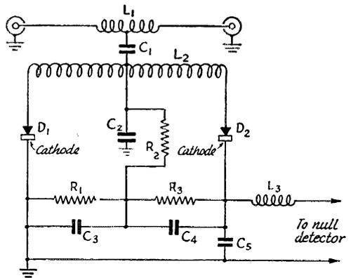
Fig. 5 — Circuit of the phase-angle detector.
