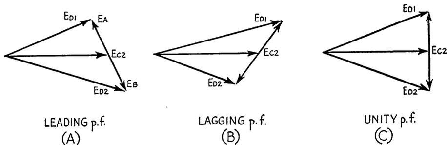
Fig. 3 — Relations among secondary voltages in phase-angle detector.
