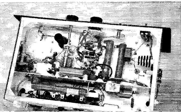
Bottom view of the 160-meter transmitter.  $R_4$  is to the left. The inverted 6AG7 oscillator tube is just to the left of the buffer tuning-condenser shaft. In front of the 813 socket are the meter-shunting resistors and the meter switch.  $R_8$  and  $R_9$  are to the right of the 813 socket. The final plate choke is mounted on the right drop of the chassis. All power wiring is done with shielded wire to suppress v.h.f. harmonics.
