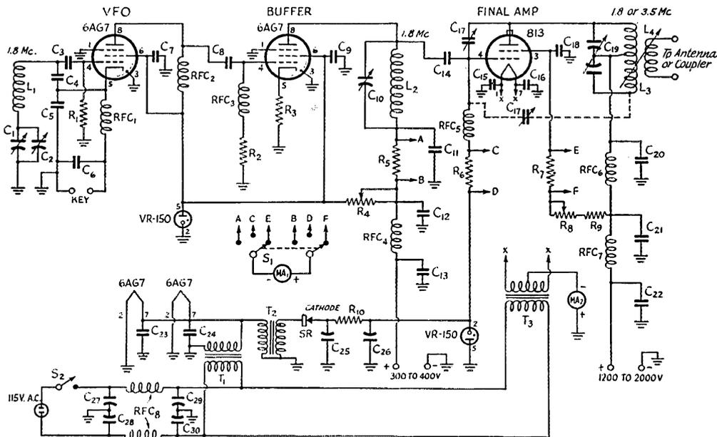
Fig. 1 — Circuit diagram of the 200-watt 160-meter transmitter.
