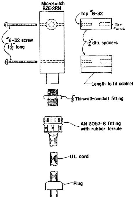
Fig. 1 — Microswitch mounting for service as rack-cabinet interlock.
