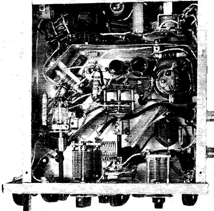
Bottom view of the quadri-band mobile rig showing the general arrangement of major components.
