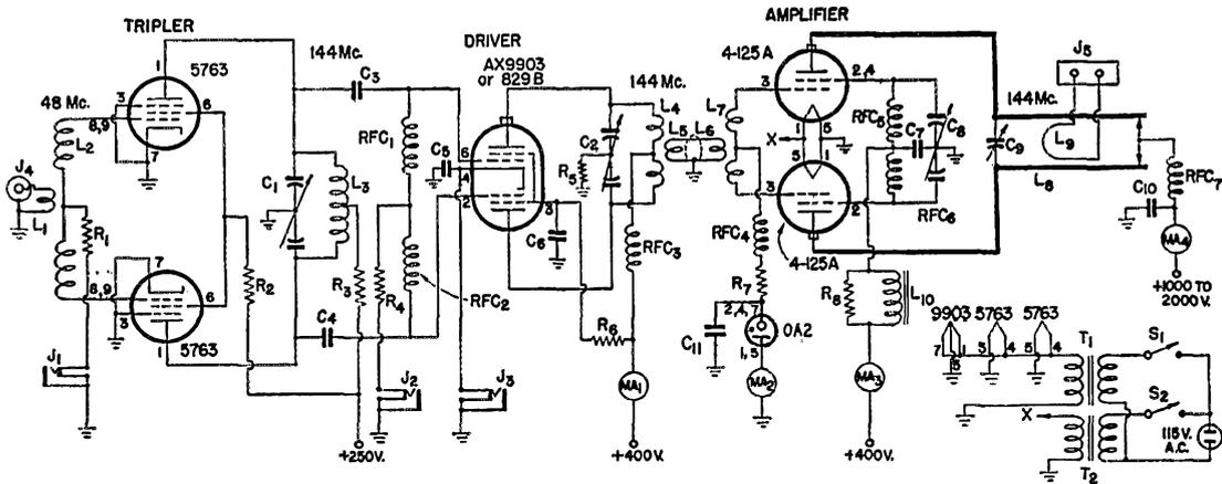
Fig. 1 — Wiring diagram and parts list for the high-powered 144-Mc. transmitter.
