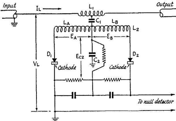
Fig. 1 — Basic circuit of the phase-angle detector.
