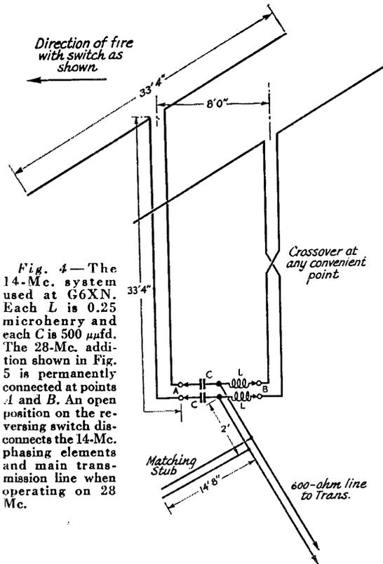
Fig. 4—The 14-Mc. system used at G6XN. Each  $L$  is 0.25 microhenry and each  $C$  is 500  $\mu\text{fd}$ . The 28-Mc. addition shown in Fig. 5 is permanently connected at points  $A$  and  $B$ . An open position on the reversing switch disconnects the 14-Mc. phasing elements and main transmission line when operating on 28 Mc.
