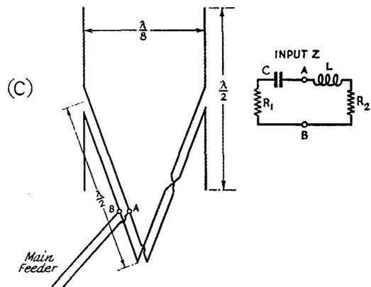
Fig. 3 — Development of the off-center feed method of phasing. The character of the input impedance seen by a transmission line connected to the terminals is shown at the right. As stated in the text, this is based on  $\lambda/8$ -wavelength spacing and exact resonance in each element plus its half-wave feeder.
