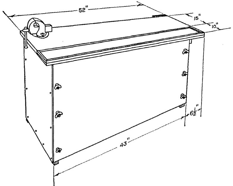
» Fig. 2— Rear view of the collapsible workbench showing essential dimensions. The hinged legs are firmly braced by a removable rear panel of plywood. Note that the top wing nut and bolt on the shorter leg must be placed lower than on the longer leg.
