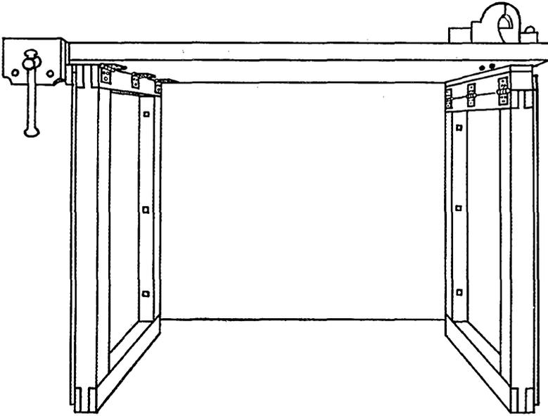
« Fig. 1— Front view of VE3PB's folding workbench. Leg room underneath is not obstructed by braces.
