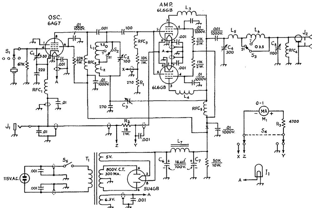
Fig. 1 — Circuit of the 6L6GB transmitter. All capacitances less than 0.001  $\mu\text{f.}$  are in  $\mu\text{mfd.}$  All 0.001- and 0.01- $\mu\text{f.}$  capacitors are disk ceramic. Capacitors marked with polarity are electrolytic. All other fixed capacitors are mica. All resistors are  $\frac{1}{2}$  watt unless otherwise specified. The 11K 6L6GB screen resistors are each made up of two 22K 1-watt units in parallel.
