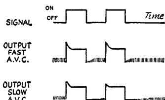
Fig. 1—Ordinary a.v.c. isn't too effective on s.s.b. or c.w. reception because it doesn't take hold fast enough to prevent overloading at the start of a strong syllable or character. Further, with a short time constant the gain jumps around too fast, as the a.v.c. tries to follow every change. With a long time constant this effect is abated, but there is still no protection at the start of a syllable or character.
