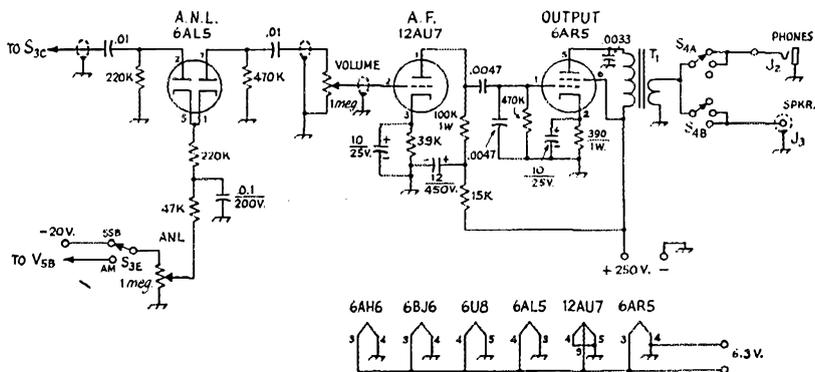
Fig. 3 — Schematic diagram of the audio portion of the amplifier. All capacitances in  $\mu$ . Fixed resistors are  $\frac{1}{2}$  watt unless specified otherwise.
