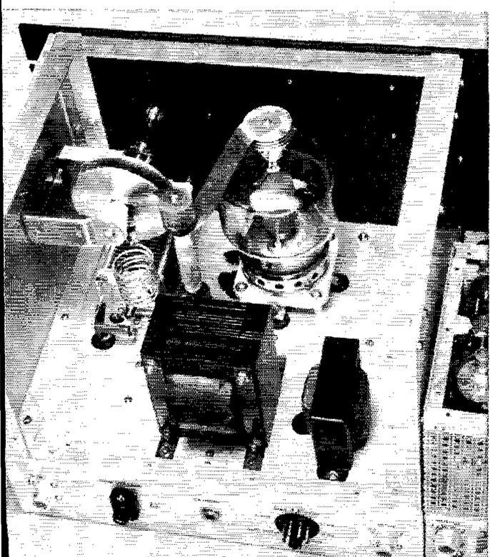
Bottom view of entire transmitter. Note that the exciter and final amplifier are built as completely separate units, though they are mounted on a single panel. Amplifier includes bias and filament supplies for both.
