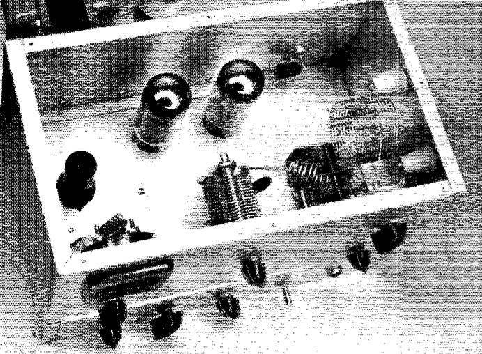
Looking down into the shielded box. Three of the crystals appear to the rear of the meter.  $C_3$  is at the center.  $C_5$  and  $L_6$  are to the right.  $L_5$  is connected between the switch and  $C_4$ .  $RFC_4$  and  $J_2$  are in the right rear corner. The holes along the bottom of the rear wall are for ventilation.  $L_7$  and the 5U4GB are behind.
