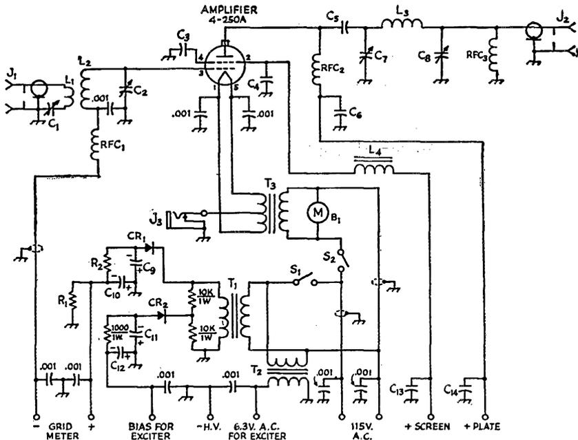
Fig. 2 — Schematic diagram and parts list for the 4-250A amplifier. All capacitors marked .001  $\mu$ f. are 600-volt disk ceramic.
