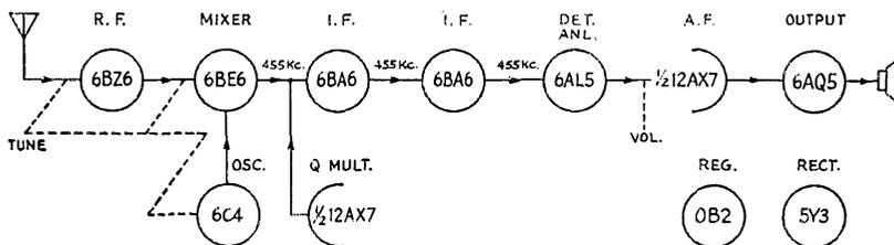
Fig. 1 — Block diagram of the HQ-100 receiver.
