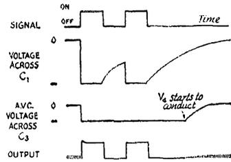
Fig. 3 — The effect of hang a.v.c. is readily understood by following the relative voltages at several points in the circuit of Fig. 2. The higher voltage developed at  $C_1$  maintains  $V_4$  cut off until some time after the signal has stopped, at which time  $C_3$  discharges through  $V_4$ .
