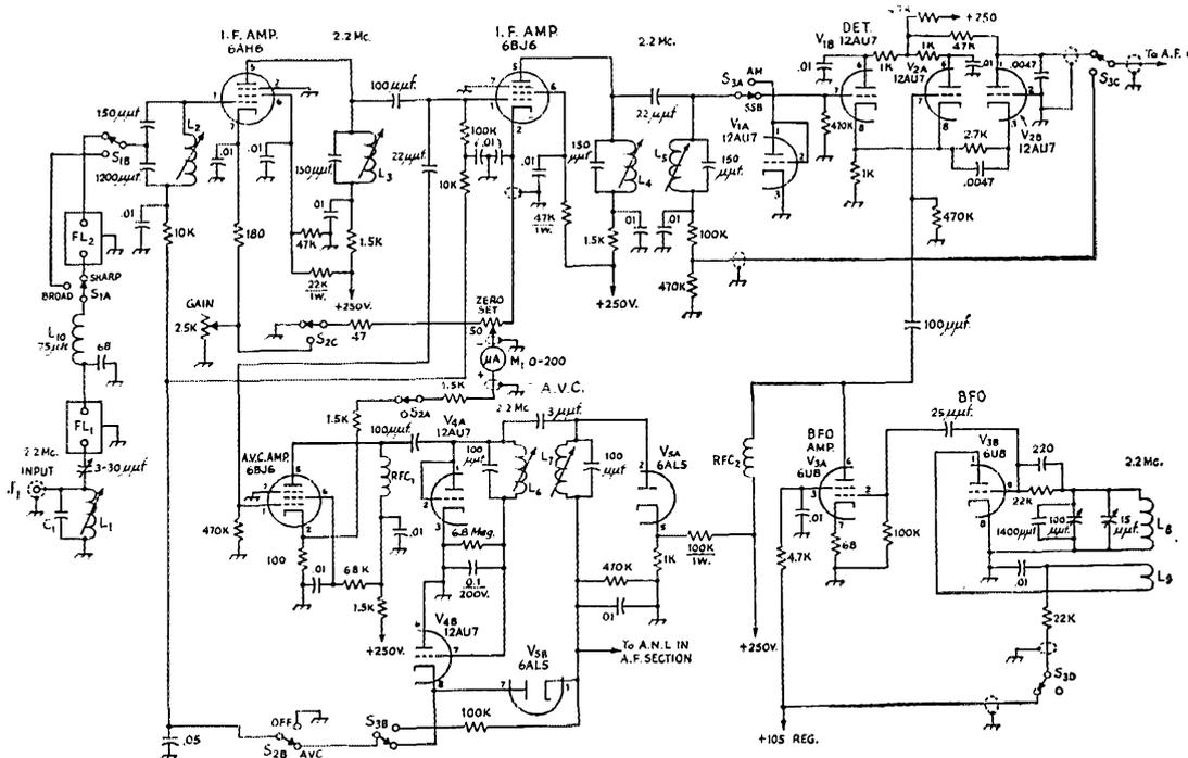
Fig. 2 — Schematic diagram of the i.f. amplifier up to and including the detector circuits.
