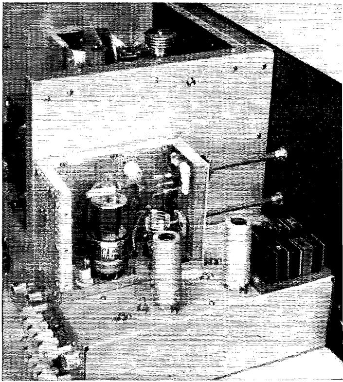
Exciter end of the 50-Mc. transmitter with shielding removed.
