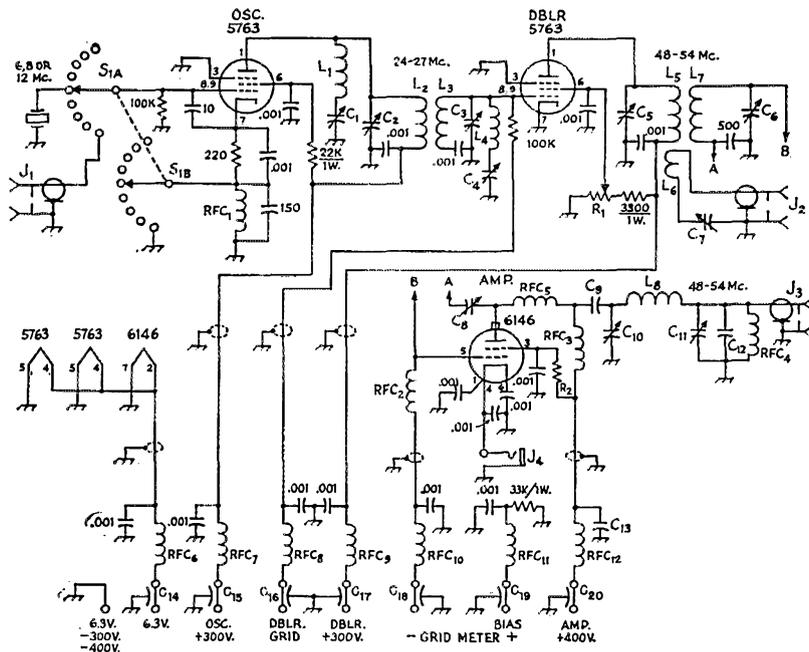
Fig. 1 — Schematic diagram of 48-54-Mc. exciter. All capacitances less than .001  $\mu\text{f}$ . are in  $\mu\text{f}$ . All .001- $\mu\text{f}$ . capacitors are disk ceramic. All resistors are  $\frac{1}{2}$ -watt unless otherwise specified.
