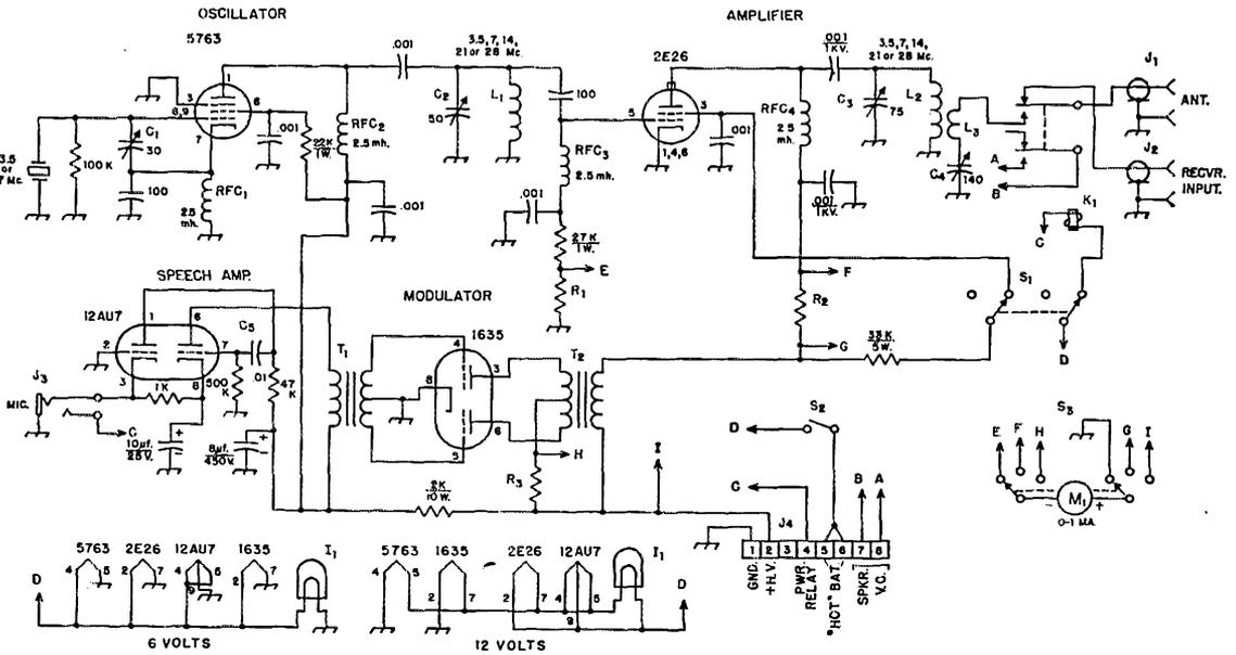
Fig. 1—Circuit of the single-band mobile transmitter. All resistors are  $\frac{1}{2}$  watt unless otherwise specified. All capacitances less than 0.001  $\mu$ f. are in  $\mu$ f. All 0.001- $\mu$ f. capacitors are disk ceramic. Fixed capacitors of smaller value may be mica or NP0 ceramic. Capacitors marked with polarity are electrolytic.
