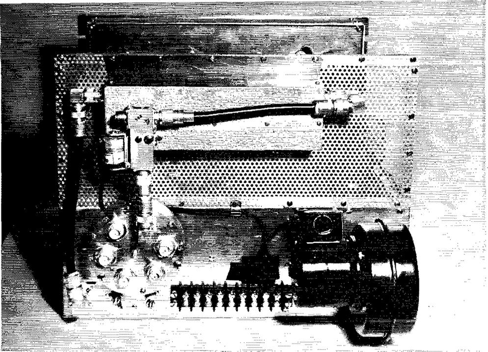
*Fig. 3* — The blower for cooling the tubes, the antenna selector switch, the antenna change-over relay and the low pass filter are all mounted on the back of the amplifier cabinet. Plate voltage is connected at the porcelain stand-off insulator under the antenna switch. Output voltage metering is obtained through the use of a high-resistance voltage divider across the output line and a 1N34A diode rectifier. The diode current is read by the output meter on the front panel.
