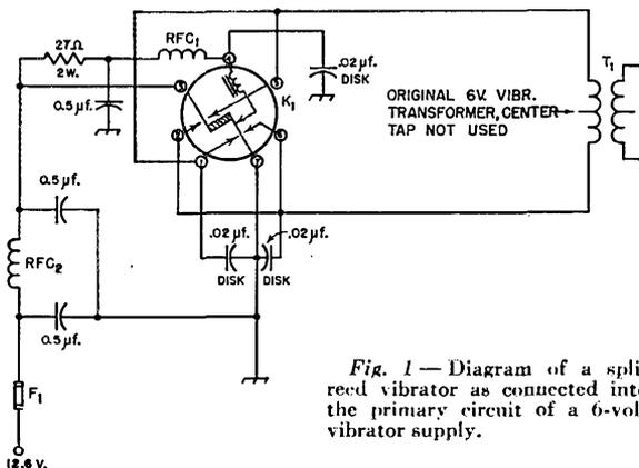
Fig. 1 — Diagram of a split reed vibrator as connected into the primary circuit of a 6-volt vibrator supply.
