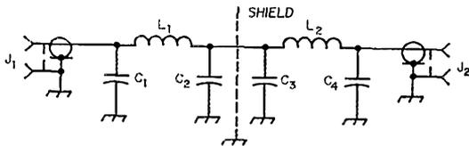
Fig. 1 — Schematic diagram of the band-pass filter.
