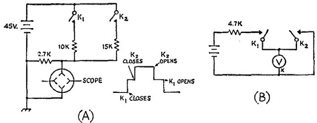
the pattern may show some "droop," but this can be ignored since the vertical lines are the important ones from which timing is measured. Of course if there is direct access to the vertical deflection plates, higher voltage and larger resistances may be used to eliminate this difficulty.
