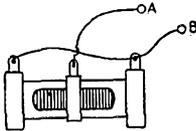
adjustable resistor. The slider is in the center of the resistor. When connected as shown, what value of total resistance must be purchased to get 25 ohms between points A and B?
