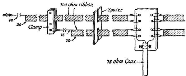
Fig. 1 — Sketch showing how ON4UF's multiple-dipole antenna system is assembled. The excess wire and insulation are stripped away.
