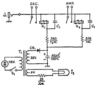
Fig. 3 — Test circuits for the keyer. These aren't essential, but they are very easy to utilize and furnish a method for comparing the delays on make and break. The make delay is about 2 milliseconds and the break delay about 4 milliseconds. Connections shown to vertical deflection plates mean connection to vertical amplifier under most conditions. See text.
