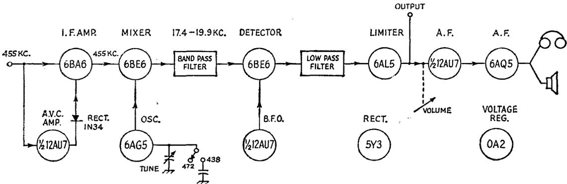
Fig. 1 — Block diagram of the GSB-1 single-side-band adapter.
