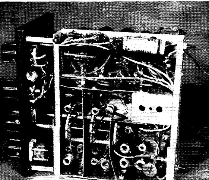
Considerable shielding is used in the mobile receiver. Three removable shield walls separate the oscillator, mixer and r.f. sections from each other and the rest of the receiver. The shield can covers the 1762-kc. oscillator circuit components.
