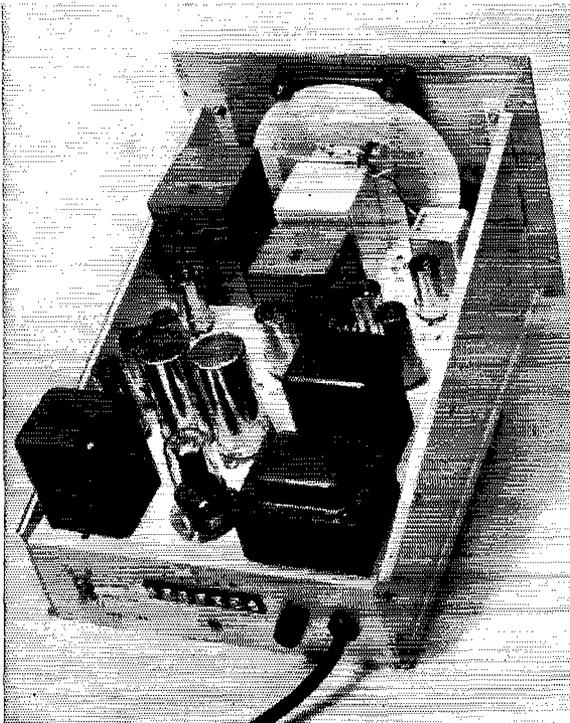
A top view of the GSB-1 removed from its case shows the clean and sturdy construction. The large tuning scale for the oscillator uses a rim drive. The band-pass filter, the heart of the adapter, is housed in the large can to the left of the tuning scale.
