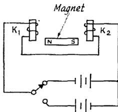
system will work even with sensitive relays in which the magnetic path is almost completely closed, although only over a small current range.
