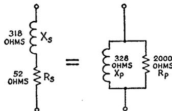
Fig. 2—An example of series and parallel circuits that are equivalent.
