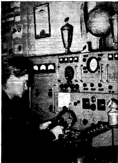
UR2KAA, multioperator-manned in Tallinn, has a rig line-up terminating in 813s, uses dipole antennae, and receives with 14- and 10-tube supers. Twenty phone and c.w. work is the station's specialty and QSLs are received direct or via the Moscow bureau. (Photo via W3VKD)
