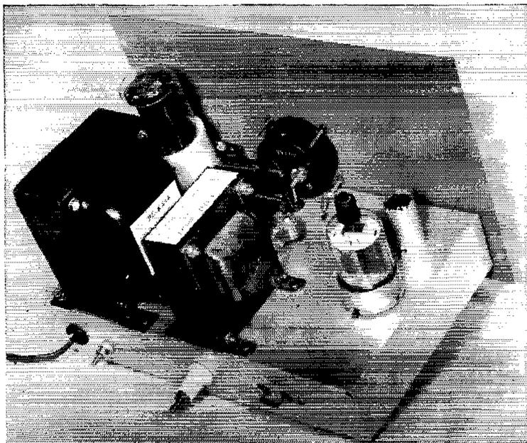
Rear view of the W3RMD transmitter. The power transformer and rectifier are to the left; the filter choke, plug-in coil and meter at the center; and the 6016 and 6AU6 to the right. The jumper in the jack on the rear wall of the chassis replaces modulator connections for c.w. operation.
