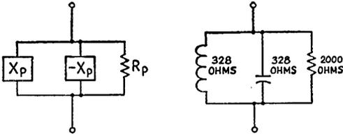
Fig. 4.—Reactance cancellation in the equivalent parallel circuit.
