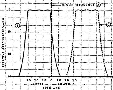
The scourge of Amateur reception is interference from neighboring signals. The most effective method of dodging this interference is passband tuning, and only Collins 75A-4 has it.
