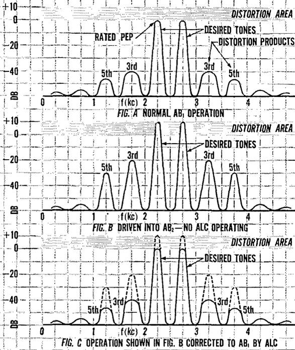
Over-driving of the power amplifier in a transmitter reduces the effective talk power of the unit by wasting power in distortion products. An important feature of Collins KWS-1 is an Automatic Load Control that automatically keeps the signal level adjusted to its rated Peak Envelope Power, and keeps distortion products at a negligible level.
