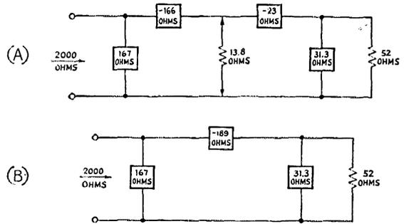
actually appear in the circuit, of course, so  $X_{R1}$  and  $X_{S2}$  can be added together and only one physical component is required. In this example it has a reactance of  $166 + 23 = 189$  ohms. The minus sign in Fig. 8A is used only to indicate that the reactance is of the opposite type to that chosen for  $X_{P1}$  and  $X_{P2}$ .<sup>8</sup>
