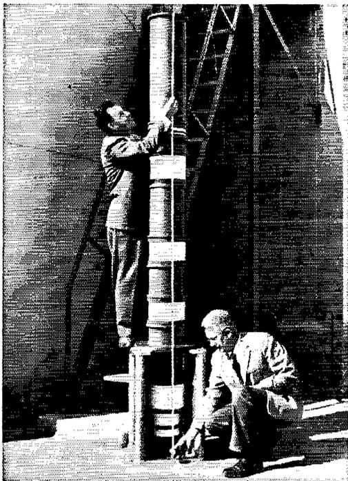
Bill Eitel, W6UF, and Jack McCullough, W6CHE, measure the world's largest electron tube, the Eimac X626 UHF klystron, which delivers 1,250,000 watts peak power and 100,000 watts average power.
