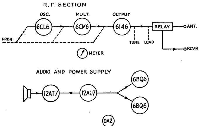
switching the antenna from receiver to transmitter. A second pole can be used to disable the receiver during transmit periods, and the third pole cuts in a low-resistance bleeder across the power supply when the plate power is turned off, to hasten the discharge of the power-supply filter and reduce the time the oscillator might "hang on."
