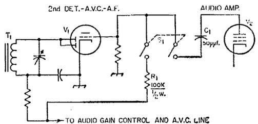
Fig. 2 — Circuit of the feed-back arrangement as applied to an a.c.-d.c. receiver by W3KKO.  $S_1$  is shown in the normal-operation position. Closing the switch completes the feed-back circuit for alarm operation.
