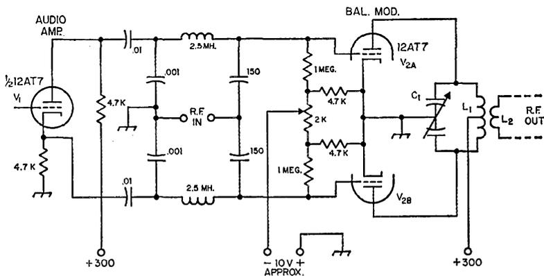
Fig. 2 — Balanced modulator circuit used in the "Pacemaker." The audio driver circuit also is shown.
