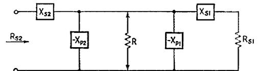
Fig. 10 — T network formed from two L sections.
