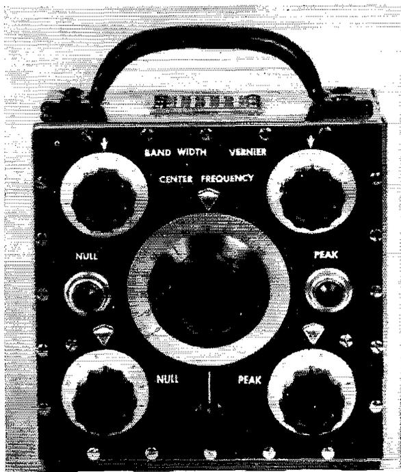
used, and to eliminate hum modulation resulting from heater-cathode leakage and diode action, the heater center tap is biased approximately +40 volts with respect to ground.<sup>2</sup> The *Q* multiplier will work excellently, however, with the heaters connected in any conventional fashion.
