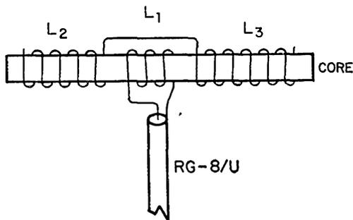
Fig. 1 — The compact all-band antenna uses a ferrite core measuring 3 inches in diameter and 3.6 feet long. L<sub>1</sub> — 5 turns No. 10 Formvar, close-wound. L<sub>2</sub>, L<sub>3</sub> — 40 turns 1/4-inch copper tubing, 1/4 inch between turns. Spacing between coils is 1/2 inch.
