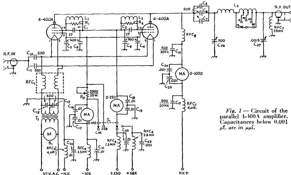
Fig. 1 — Circuit of the parallel 4-400A amplifier. Capacitances below 0.001 μf. are in μmf.
