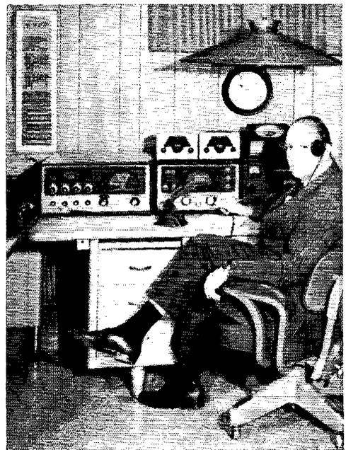
W9IOP, need more be said? Larry concentrated on 80-40-20 using an HT32A and SX115 indoors and a 100' tower outdoors supporting 15 over 20 over 40 rotary beams, using the insulated guys fed as an inverted Vee for 80. Results: tops for Indiana, leading Central Division c.w. score, third high code tally nationally. That youthful appearance (after years of S5ing as W2 W8 and W9IOP) is attributed by Larry to ham radio keeping him too busy for other normal "vices."
