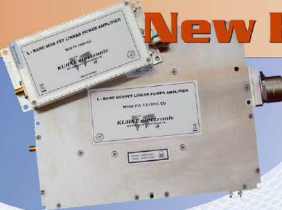
The brand new power amplifiers MKU PA 131000 CU and MKU PA 13250 CU provide excellent efficiency together with brilliant linearity and are ideally suited for huge EME- and contest-operations. The used LDMOS technology represents the current state of the art and allows the development of compact amplifier modules with high output power.
