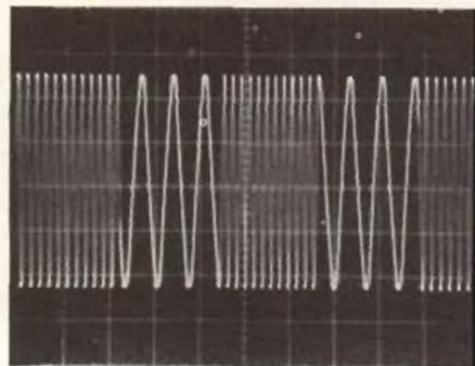
Fig. 28 - Uscita FSK (frequency-shift-keyed) con  $F1 = 4F2$ .
