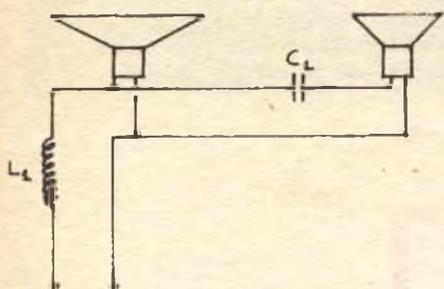
$C_L = \text{cond. } 2 \text{ mf } 50 \text{ V lav.}$
