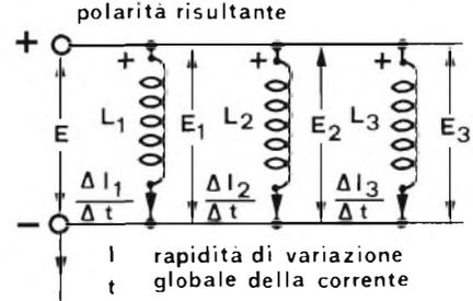
$$E = L_1 \frac{\Delta I_1}{\Delta t} \quad E_2 = L_2 \frac{\Delta I_2}{\Delta t} \quad E_3 = L_3 \frac{\Delta I_3}{\Delta t} \quad E = L \frac{\Delta I}{\Delta t}$$
