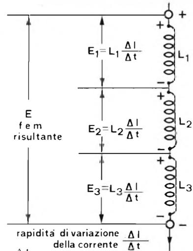
$$E_1 = L_1 \frac{\Delta I}{\Delta t} \quad E_2 = L_2 \frac{\Delta I}{\Delta t} \quad E_3 = L_3 \frac{\Delta I}{\Delta t} \quad E = L \frac{\Delta I}{\Delta t}$$
