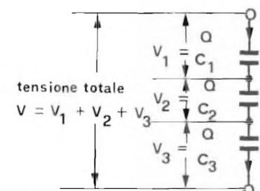
$$V_1 = \frac{Q}{C_1} \quad V_2 = \frac{Q}{C_2} \quad V_3 = \frac{Q}{C_3}$$
