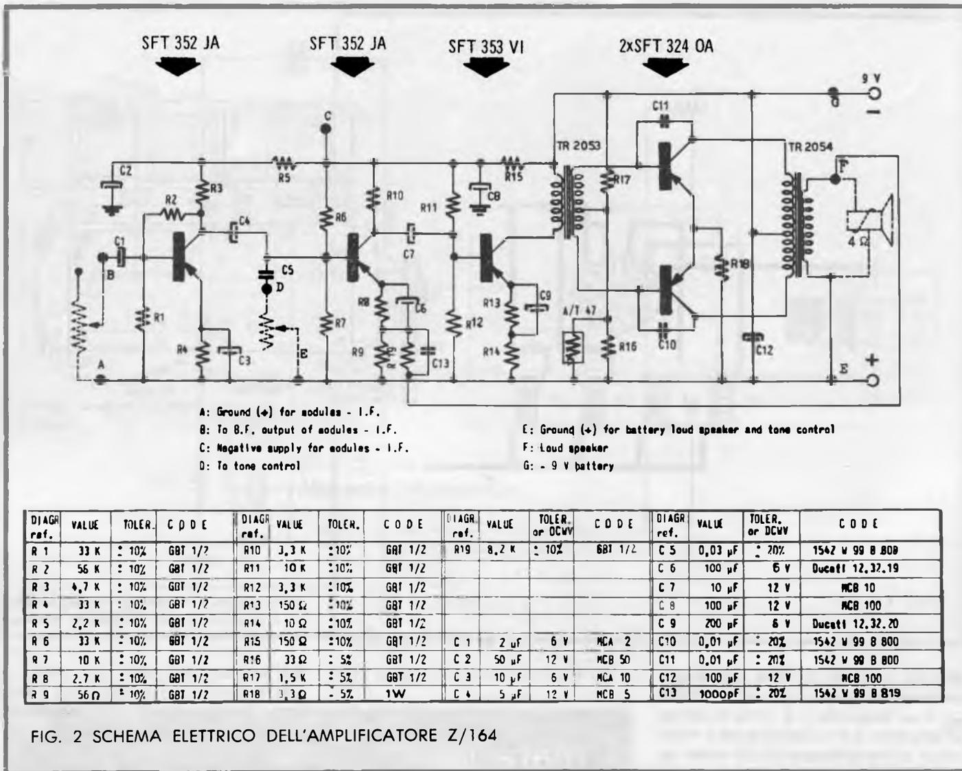
FIG. 2 SCHEMA ELETTRICO DELL'AMPLIFICATORE Z/164
