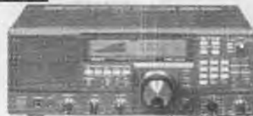
YAESU FRG-8800 SHORTWAVE MW AND SHORTWAVE GENERAL COVERAGE RECEIVER
