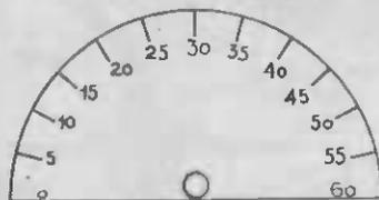
Removable plates of an old condenser may be used as a dial plate by carefully engraving them. With the aid of a sharp tool professional appearance is obtained. A pointer knob may be used to provide an excellent dial.
