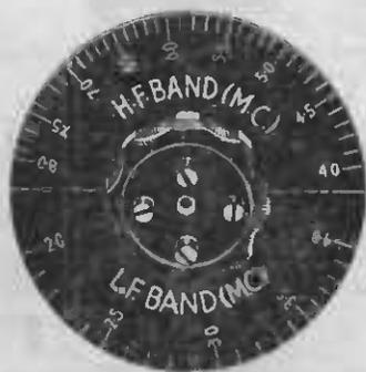
Dials as used in the sender and receiver sections of Z.C.1's. Can be set for two preset frequencies, with flick tuning mechanism. Diameter of dial, 4in.; diameter of hand-grip instrument knob, 2 1/2in.—Cat. No. TX1090/4 **4/-** each
