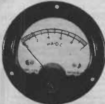
0-1 M.A. Moving Coil D.C. Meters. 1000 ohms per volt. Internal resistance 60 ohms.
