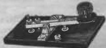
Heavy brass arm and bridge. Fine adjustment of spacing and tension provided. Wooden knob, and finger rest flange, ensuring comfortable operation grip. Mounted on wooden base, finished in varnish. Measures 6in. long, 3in. wide, 3in. high (overall).
