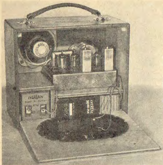
Back view of the receiver, showing the physical layout of the chassis, speaker, and batteries. Although the set is quite small, there is plenty of space available.
