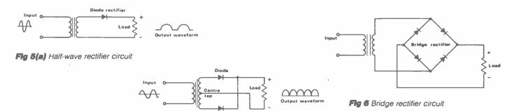
Flg 5(b) Full-wave rectifier circuit
