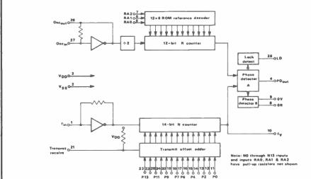
Fig 7 Motorola MC145151 PLL chip
