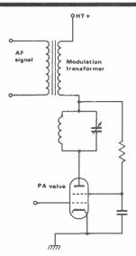
Fig 1b Amplitude modulation of a valve PA stage using a modulation transformer
