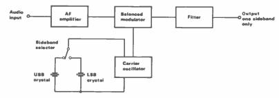
Fig 3 SSB generator block diagram
