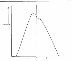
Effect of IF transformer response if the tuned circuits are not on the same frequency
