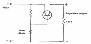
Flg 8 A simple voltage regulator circuit
