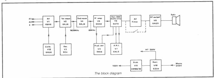
produce an intermediate frequency of 1620KHz
