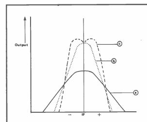
Effect of under (a), critical (b) and over (c) coupling of IF transformers
