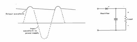
Fig 7 Waveforms for a rectifier circuit using a reservoir capacitor C
