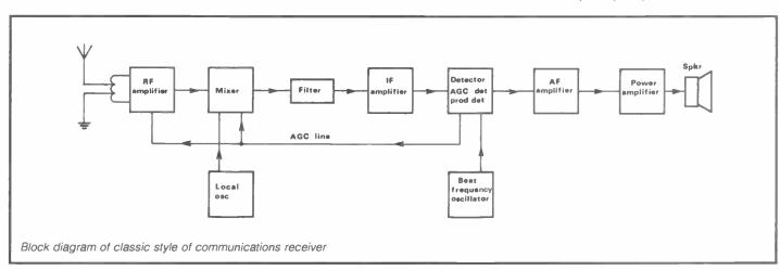
The IF amplifier is situated between the anode (in valve equipment), collector or drain (in solid-state receivers) of the mixer and the detector stage. It comprises a selective filter, either mechanical or crystal, followed by two or three stage or amplification-coupled IF transformers.
