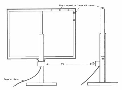
Fig 4 Details of the frame/co-ax arrangement
