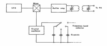
Fig 4 Mixer-type exciter block diagram
