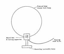
A possible refined version of the loop antenna
