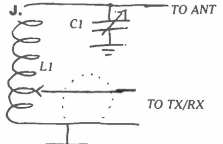
L1 35 turns 16 SUG 2" former 4" long tapped 5 turns up C1 500pf broadcast type variable.
