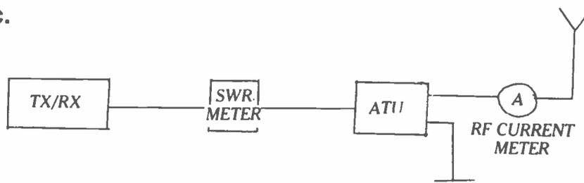
A method of connecting rig to end fed, current fed or other low impedance fed aerial. The SWR meter ensures a good match between rig and ATV. With such aerials (e.g. 132' wire) the object is to get as much RF current as possible indicated in the RF ammeter. The reading on the ammeter will depend upon aerial length and earth efficiency. Add radials or earth spikes until a greater reading cannot be obtained.
