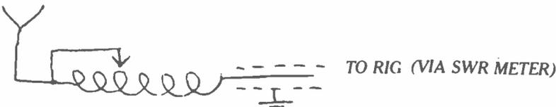
If a series inductor is used, the mobile whip should be adjusted to resonate on the highest frequency required. By increasing the number of turns in the series inductor (which can be in the shack) the frequency of the aerial system is lowered. Series Inductor can be ex government roller coaster type or made up of 16 SUG wire space wound 25 turns 1" to 2" diameter. Adjust for maximum aerial current and minimum SWR.
