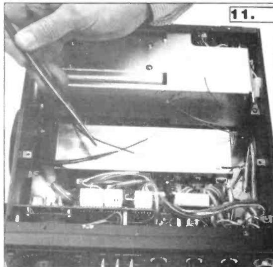
**11.** Replace both psu and synthesiser assemblies arranging RPCB251ub cables leading from slots on either side of synthesiser assembly.
