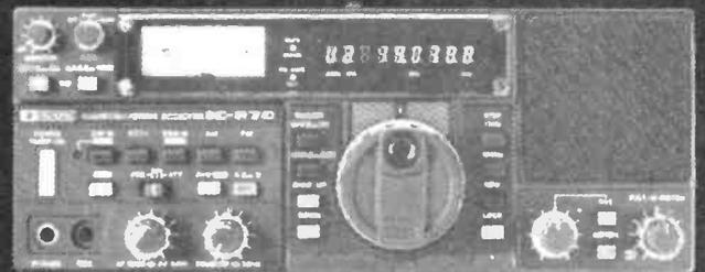
The R-70 covers all modes (when the FM option is included), and uses 2 CPU-driven VFO's for split frequency working, and has 3 IF frequencies: 70MHz, 9MHz and 455KHz, and a dynamic range of 100dB. It has a built-in mains supply.
