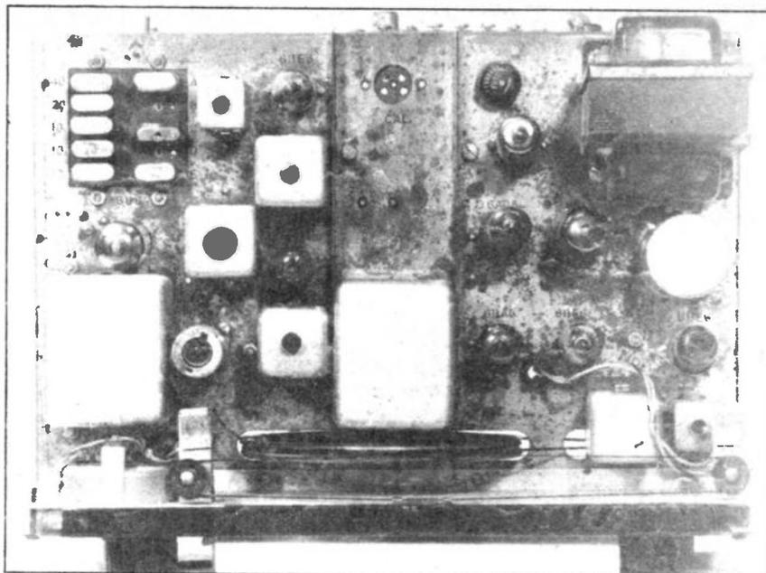
Top view of the Drake 2B. The discolouration of the chassis is due to the ravages of too many years in leaky garden shed shacks. The performance was not affected, however.
