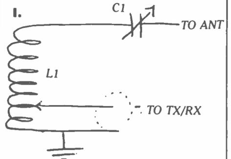
L1 35 turns 16 SUG 2" long tapped 5 turns up C1 500pf broadcast type variable (body & shaft must be insulated).
