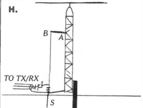
Gamma match feed of earthed tower. Correct impedance obtained by moving point A up and down tower, and by making A to B longer or shorter.
