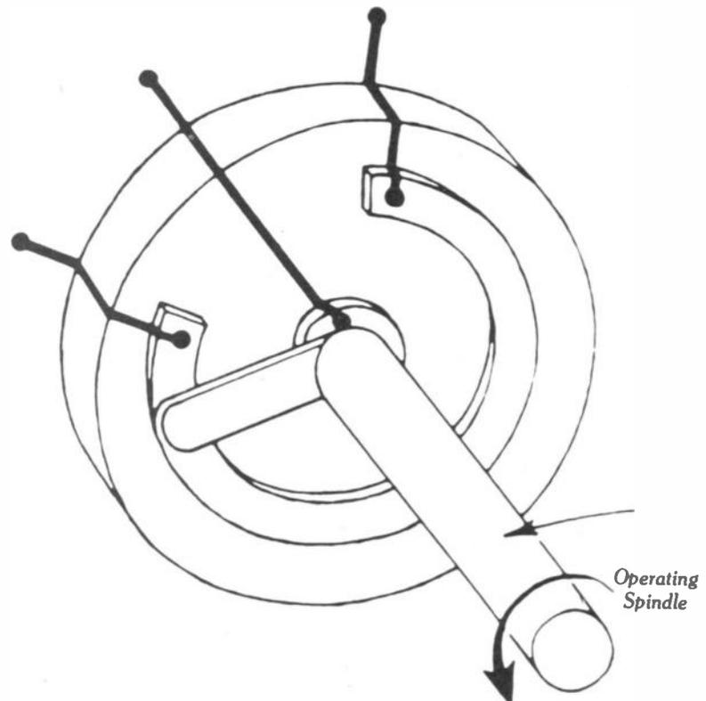
Rotary Type Variable resistor
