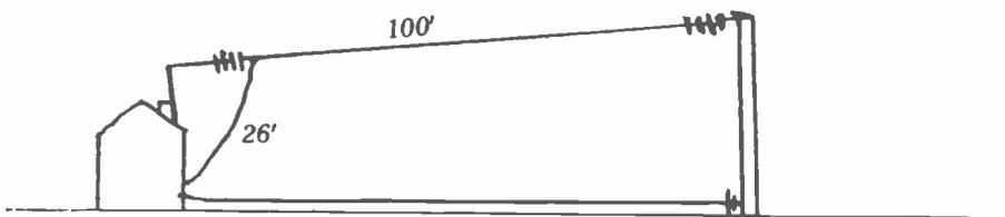
A method of turning a quarter wave inverted L aerial against a counterpoise. The counterpoise is a quarter wave length of insulated wire running about one foot above ground level. One end is connected directly to the rig on ATV and the other end disconnected. Improved performance can be obtained by using several similar radials all connected together at one end and laid out like spokes of a wheel. (If radials are used the equipment should also be earthed for safety purposes).
