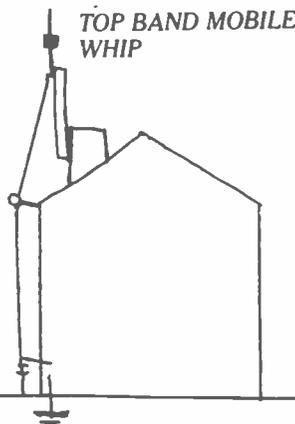
An old or redundant mobile whip can be used by connecting its base to an insulated (non metallic) pole attached to chimney etc. The base is connected to wire down lead and taken via a stand off insulator to the shack. The whip and the downhead will act as the aerial, but the conductor below the loading coil does the work. Such a system can be turned by using a series tuned ATV or a series inductor.
