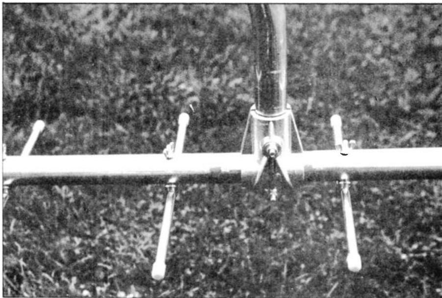
Anyway, the other relevant figures for the 18-element Parabeam suggest a front-to-back ratio of 18dB and a 3dB beamwidth (which tells you who sharp the thing is, in effect) of 25 degrees. The boom length of the beast is 2.8 metres.
