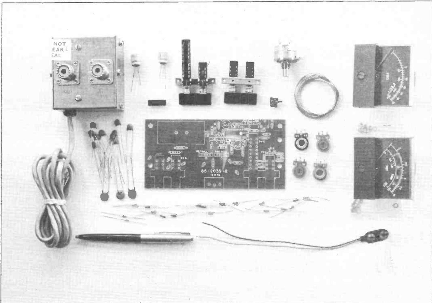
Pictures on these pages show resistors and capacitors (and a few other things as well) in their rightful positions as components of working radio. Note the comparison in size when seen next to valves and a 50p coin. Incidentally, the construction pictures show projects from previous issues of *Amateur Radio*.
