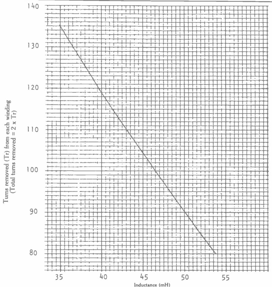
NOTE: This data applies to 88mH inductors in stacks with wooden end spacers. Inductance vs. turns removed from each winding of an 88mH inductor with wooden end spacers (for L3 modification)
