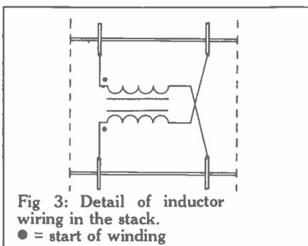
Fig 3: Detail of inductor wiring in the stack.
