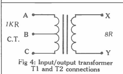
Fig 4: Input/output transformer T1 and T2 connections
