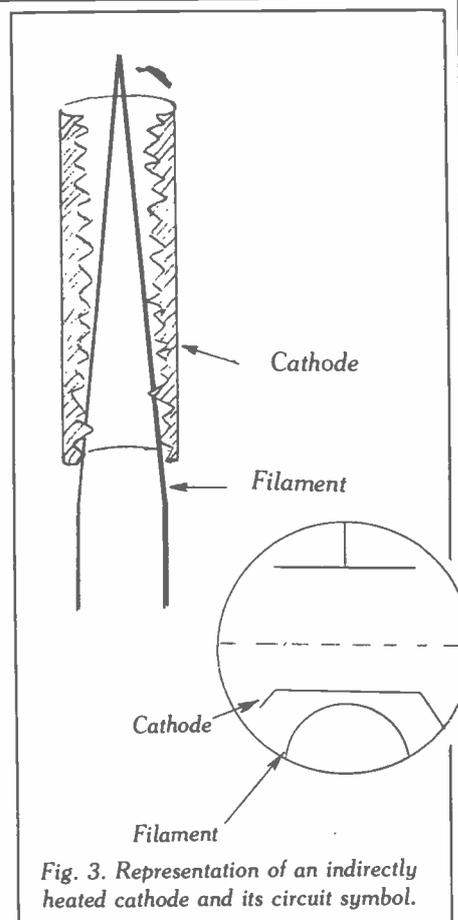
Fig. 3. Representation of an indirectly heated cathode and its circuit symbol.
