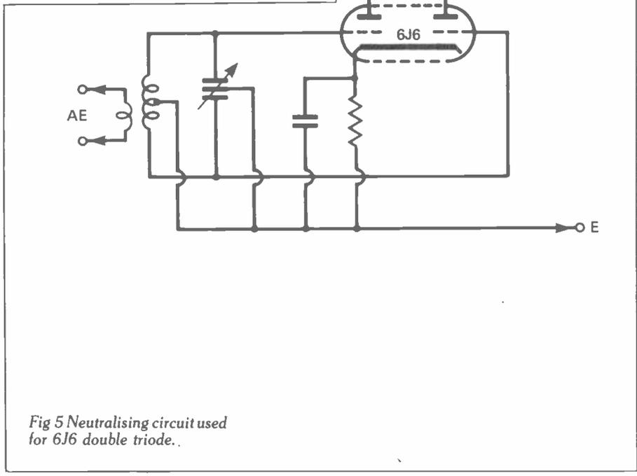
Fig 5 Neutralising circuit used for 6J6 double triode.
