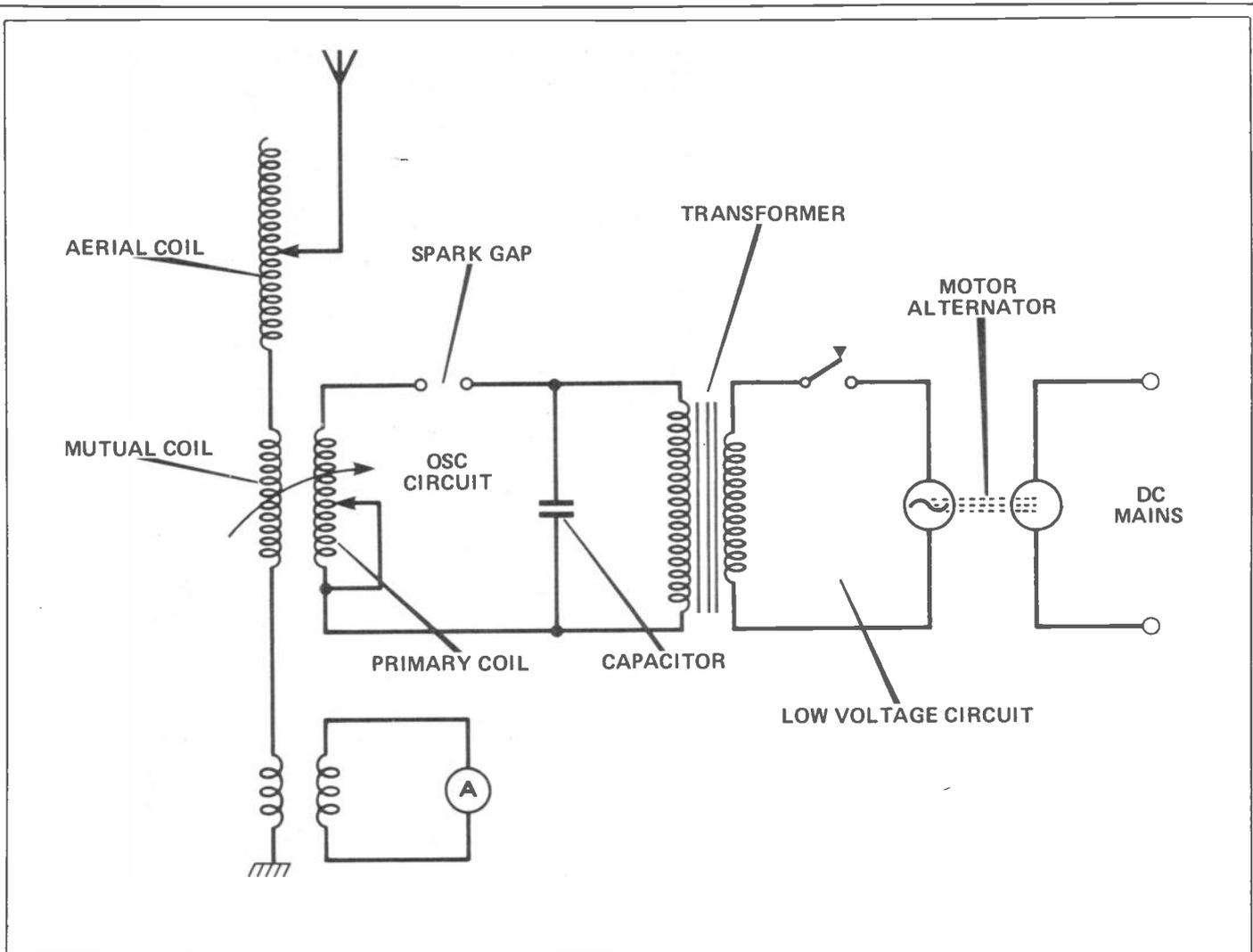
The "quenched gap" was essentially another form of the old fixed gap. In the quenched gap the spark gap was divided into a number of short gaps in series. The disc shaped electrodes, each roughly six inches diameter, were made of silver plated copper. A spark gap consisted of a number of such discs clamped together in the form of a sandwich, separated by mica washers roughly two millimetres thick.
