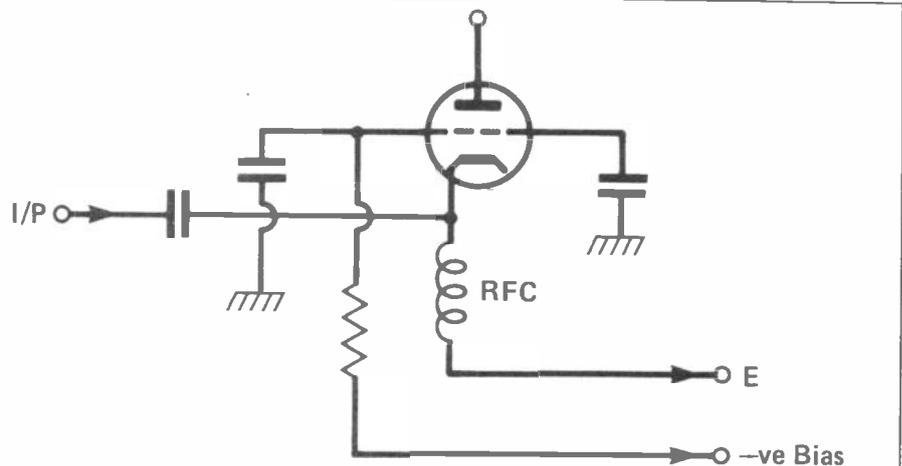
Fig 8 Directly heated valves need careful filtering of the heater supply
