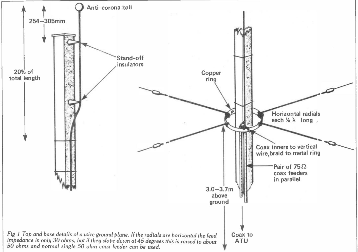
Fig 1 Top and base details of a wire ground plane. If the radials are horizontal the feed impedance is only 30 ohms, but if they slope down at 45 degrees this is raised to about 50 ohms and normal single 50 ohm coax feeder can be used.
