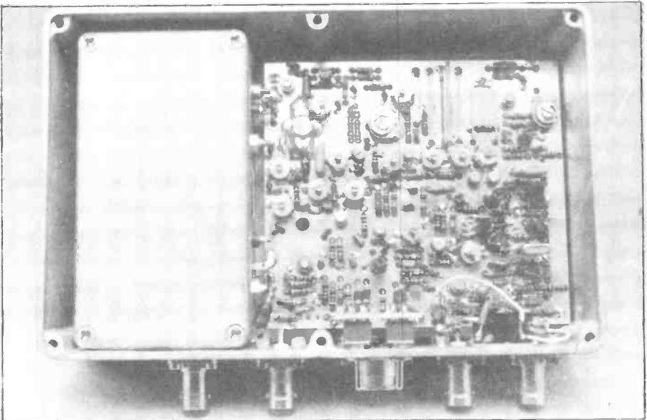
*Above: Microwave modules 432MHz transverter. Bottom of page: Lunar preamplifier.*
