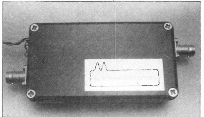
is, you must consider its gain. The lower the gain, the less able the preamp will be to overcome the noise of the main rig. An incredible preamp with 0.5dB noise figure, and 10dB gain would give a system noise figure of as high as 3dB when feeding a black box with a 10.5dB noise figure.
