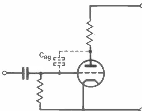
Fig 1 Capacitance exists between the grid and anode of a triode ( $C_{ag}$ ).
