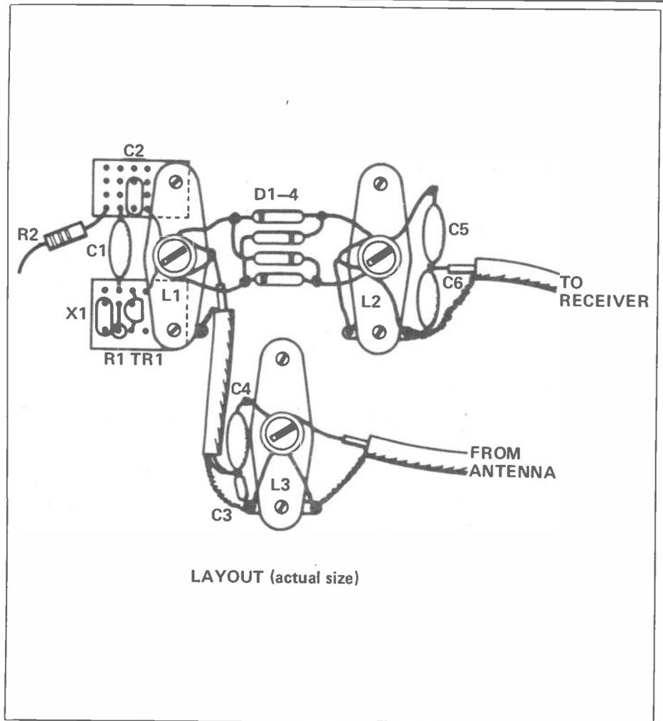
Above: wiring layout (fig 3A). Below: frequency conversion graph, Fig 4.
