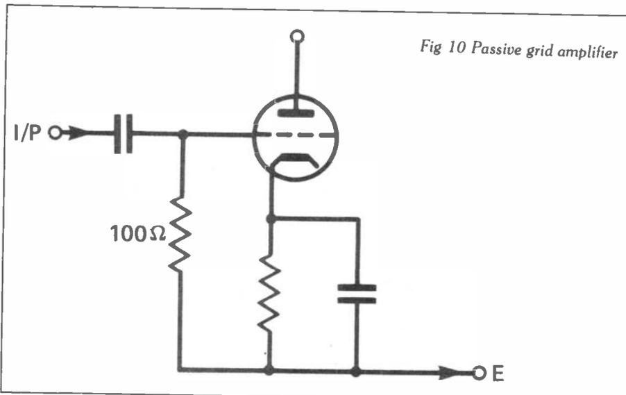
Fig 10 Passive grid amplifier
