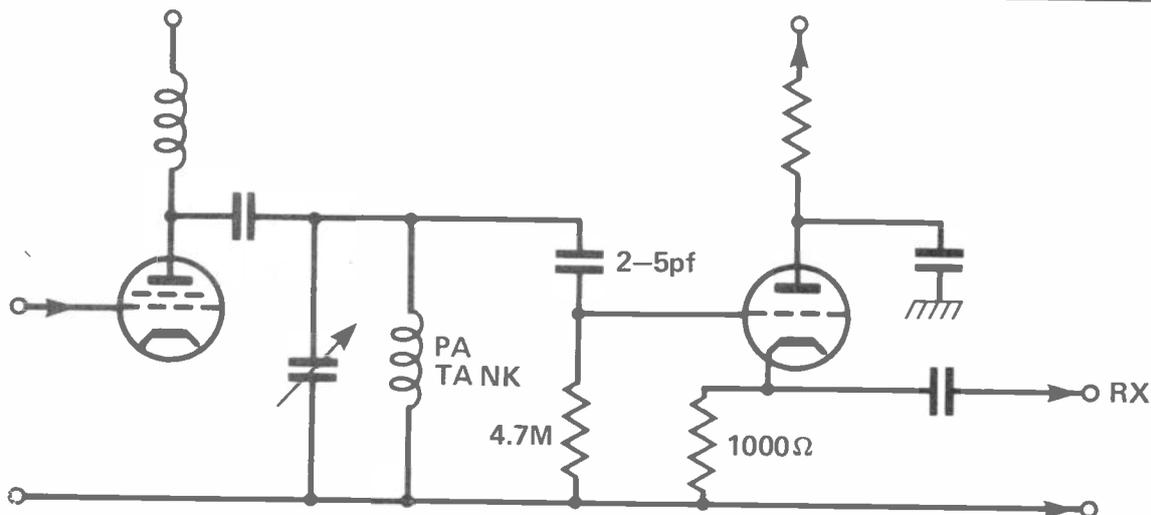
Fig 12 Electronic T/R switch
