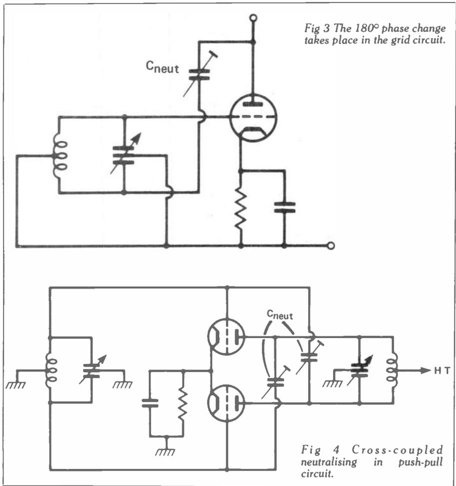
Fig 3 The 180° phase change takes place in the grid circuit.
