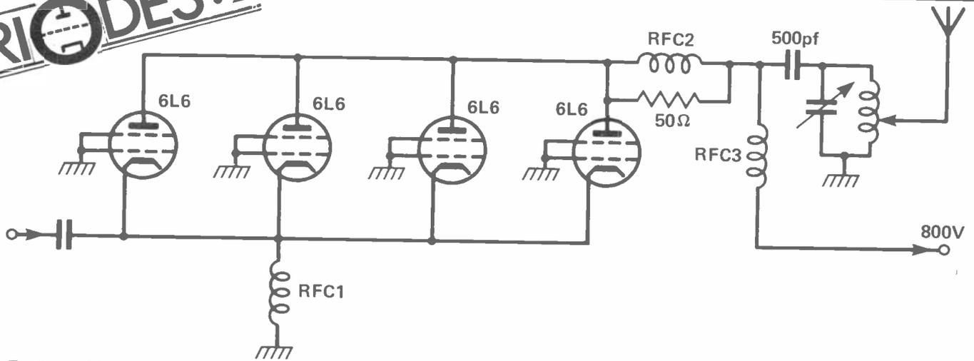
Fig 9 Amplifier circuit using four 6L6 tetrodes
