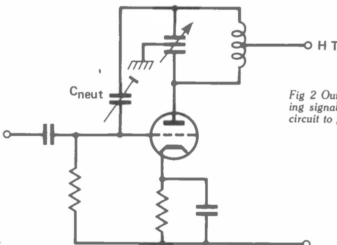
Fig 2 Out-of-phase neutralising signal is fed from anode circuit to grid.
