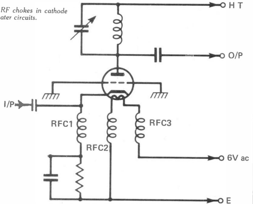
Fig 7 Grid is grounded as far as RF is concerned, but DC bias can still be applied.
