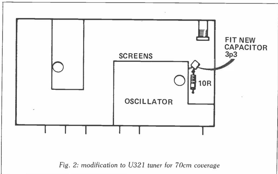
Fig. 2: modification to U321 tuner for 70cm coverage
