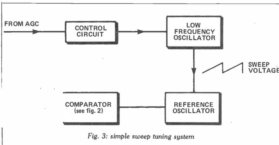
Fig 3: simple sweep tuning system
