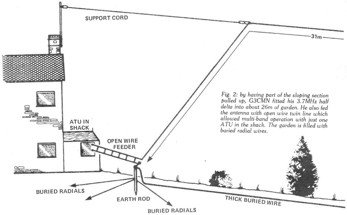
Fig. 2: by having part of the sloping section pulled up, G3CMN fitted his 3.7MHz half delta into about 26m of garden. He also fed the antenna with open wire twin line which allowed multi-band operation with just one ATU in the shack. The garden is filled with buried radial wires.
