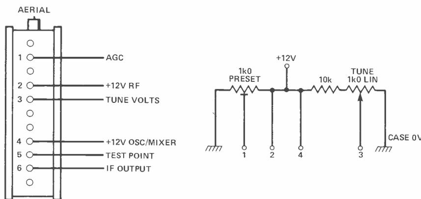
Fig. 5: ELC1043 pin connections and wiring
