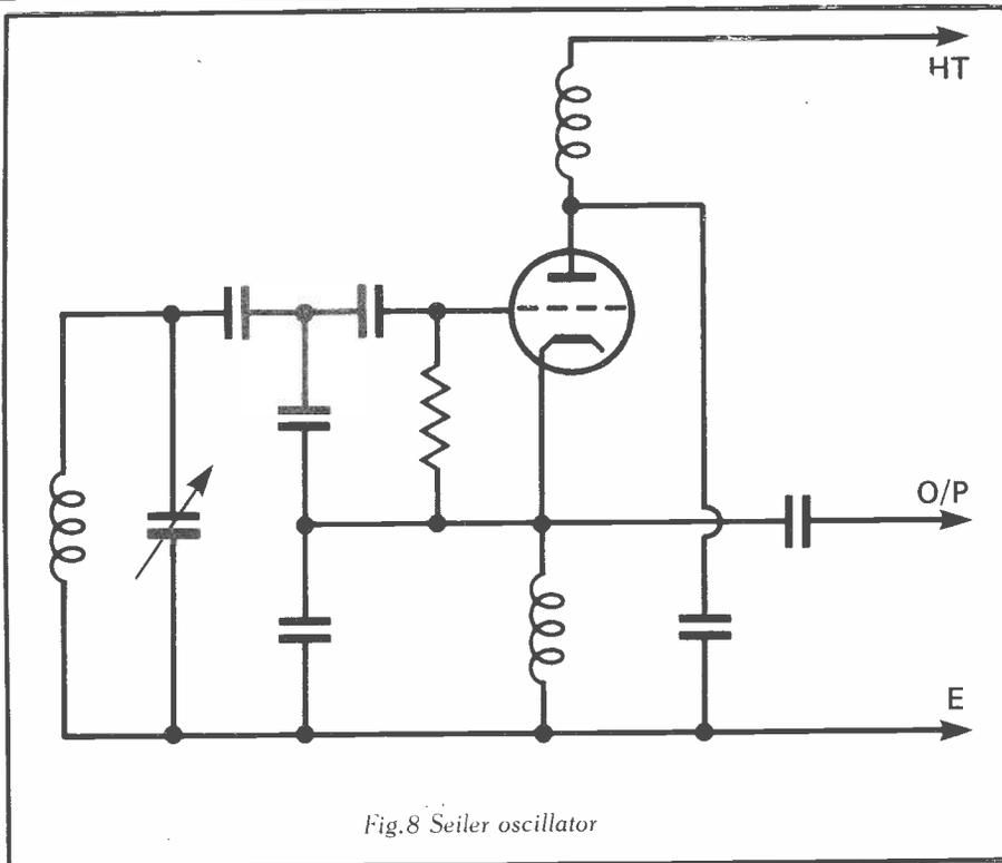
Fig.8 Seiler oscillator
