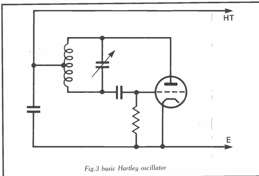
Fig.3 basic Hartley oscillator
