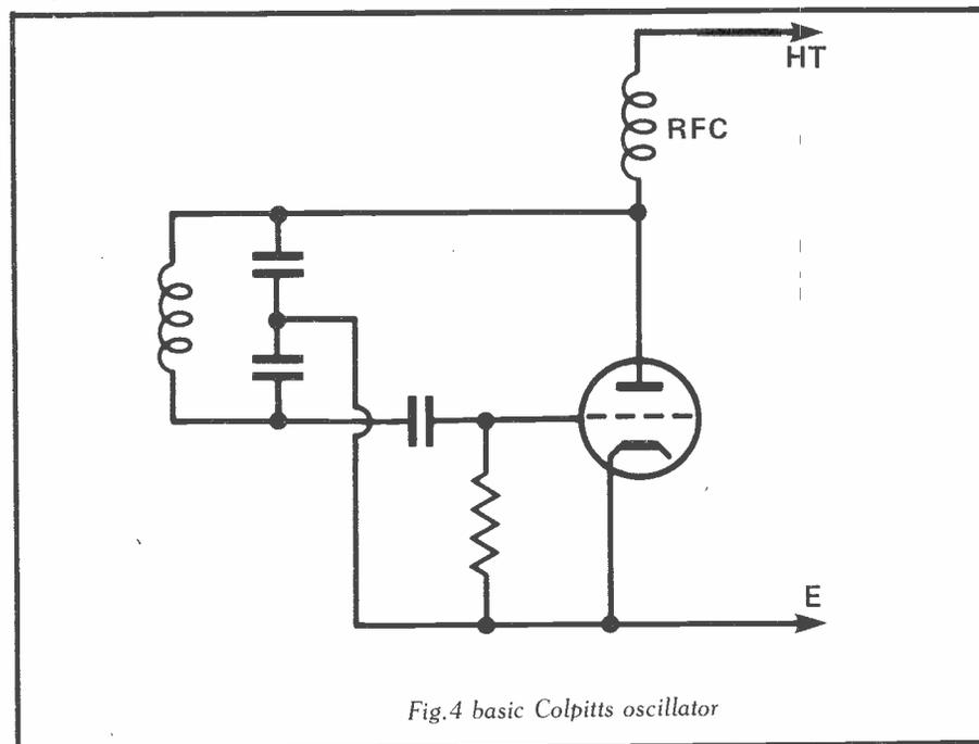
Fig.4 basic Colpitts oscillator
