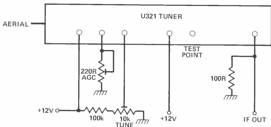
Fig. 6: U321 wiring for 70cm operation
