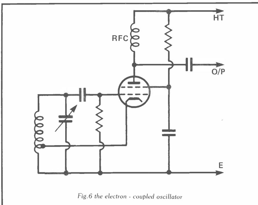
Fig.6 the electron - coupled oscillator
