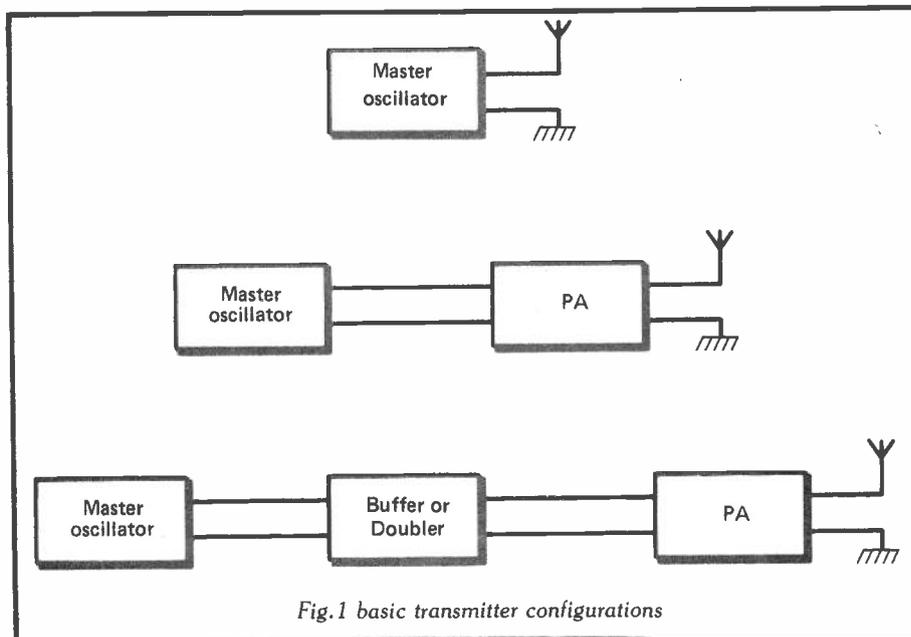
Fig.1 basic transmitter configurations
