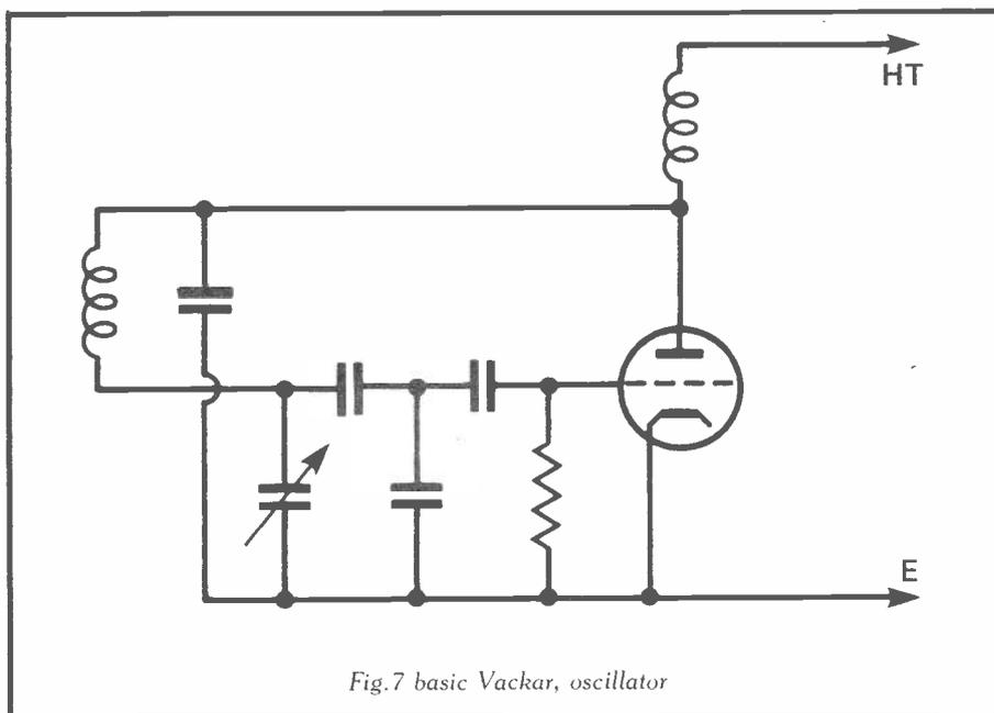
Fig.7 basic Vackar, oscillator
