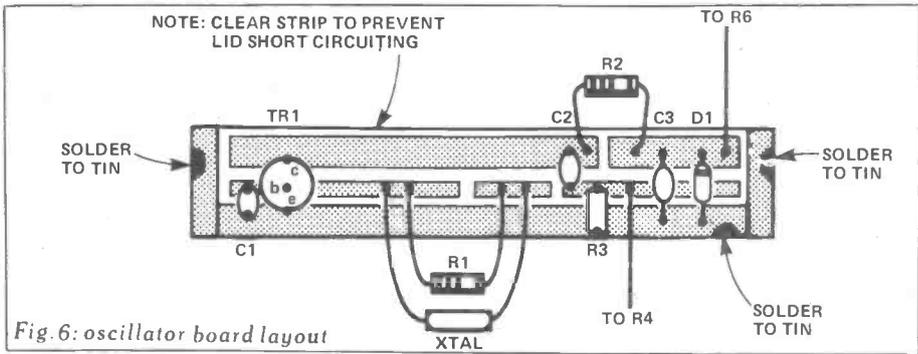
Fig. 6: oscillator board layout
