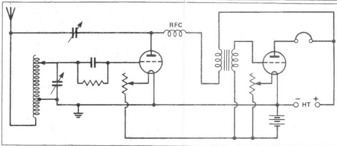
An O-V-1 receiver using the Reinartz detector circuit which is typical of the receivers of the 1920s.
