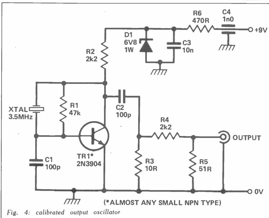
Fig. 4: calibrated output oscillator
