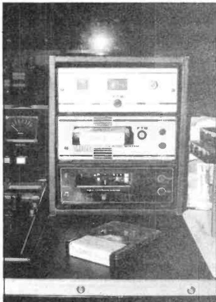
NAB cartridges contain an endless loop of tape and are used for jingles, commercials etc.
