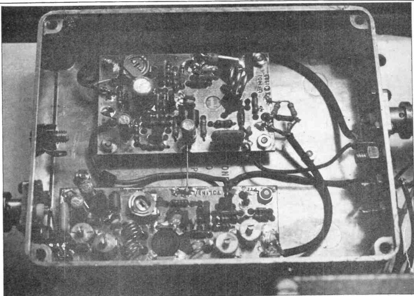
Wood and Douglas with the lid off: UFM01 power oscillator and 70LIN3 amplifier, assembled by G3YQC who finds a very satisfactory combination. Note 3dB pad between oscillator and amplifier stage to ensure stability.
