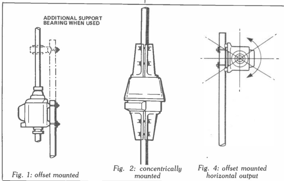
This is the horizontal force acting on the rotator and is directly related to the wind load of the aerial and its supporting structure, and the height of the aerial above the rotator. The bigger this distance is, the bigger the bending load on the rotator for a given wind speed. The extension mast also induces a side load on the rotator because of its own wind resistance.
