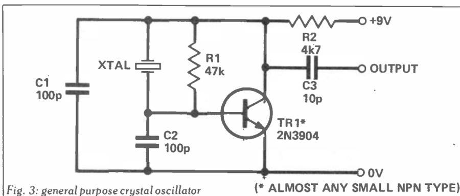
Fig. 3: general purpose crystal oscillator
