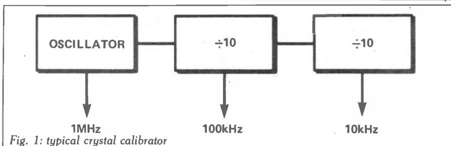
Fig. 1: typical crystal calibrator
