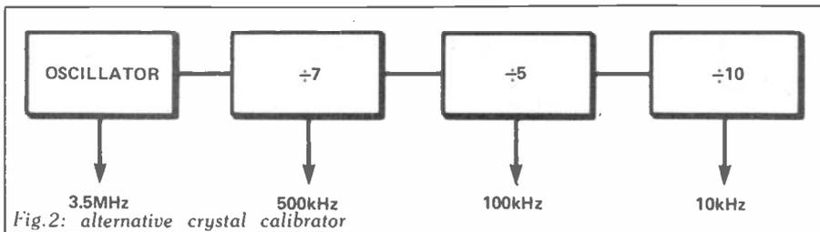
Fig.2: alternative crystal calibrator
