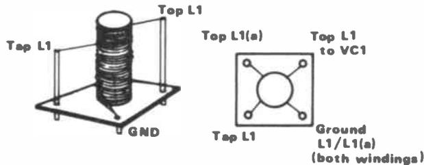
Fig 5 L1/L1A winding details
