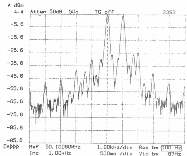
Complete transmitted response from mic socket input to RF carrier output, well below any ALC action showing filter response, alternate sideband and carrier rejections
