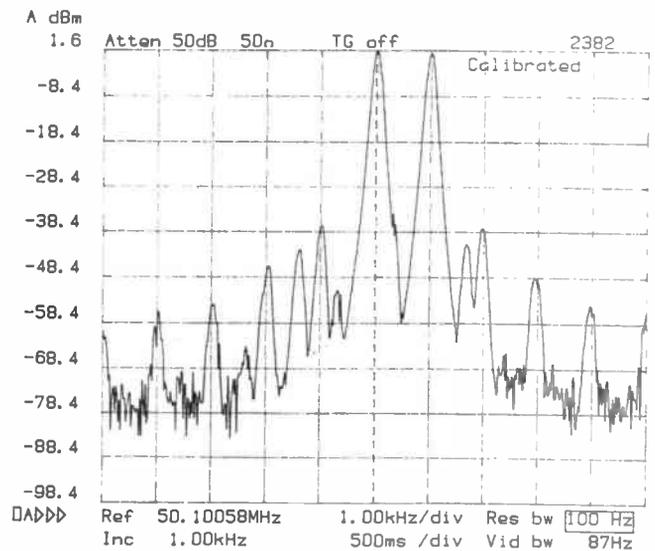
Two-tone test of TS670 on 50.1MHz at full power
