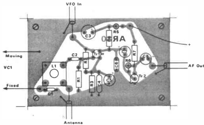
Fig 3 PCB with component overlay
