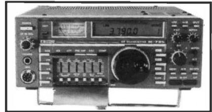
★ 12 tunable memories ★ Gen coverage RX ★ Scanning ★ 100kHz to 30MHz all mode super receiver
