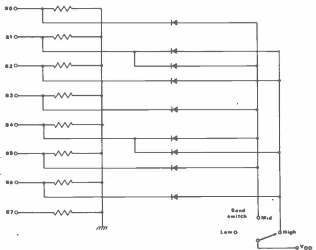
Fig 5 Modified diode matrix for 10m conversion
