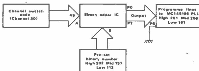
Fig 2 Block schematic diagram of binary adder circuit
