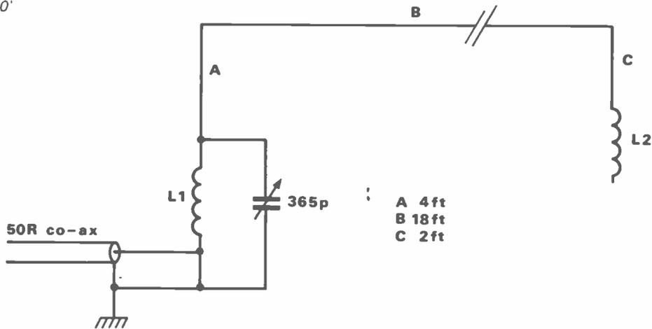
tuning capacitor has been adjusted for optimum results, there is no need to alter anything over the whole of the CW part of the 80 metre band.
