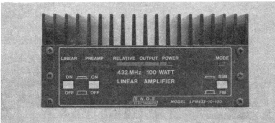
just 3W input for full output, whilst an almost identical version, having a fixed passive attenuator on the input, requires 10W for full output. BNOS have designed them so that they should be suitable not only for SSB, CW and FM, but also for amateur television. They have taken care to design the circuits for good linearity at
