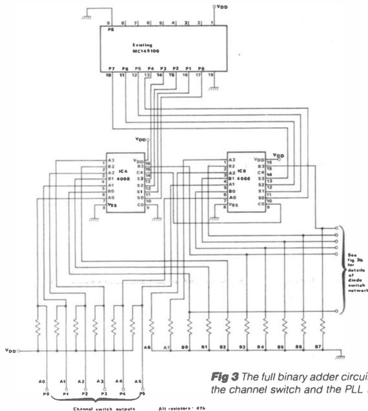
Fig 3 The full binary adder circuit interposed between the channel switch and the PLL IC
