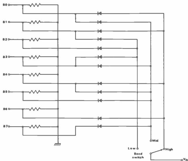
Fig 4 Diode switching matrix for unconverted set
