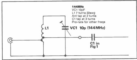
Fig 2: Circuit to limit response
