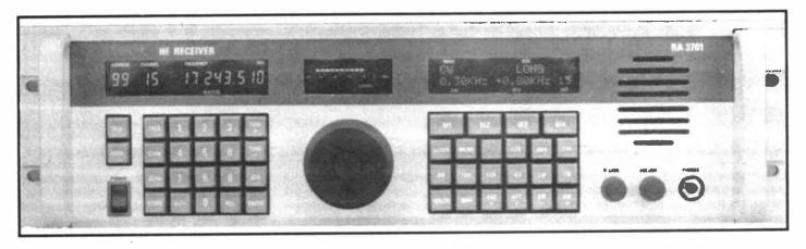
The front panel of the RA 3701 HF receiver
