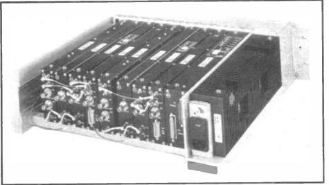
MA 3700 receiver control unit with a complete set of modules
