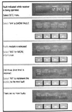
Step by step sequence of locating a fault via the BITE circuitry
