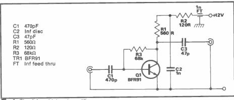
Fig 1: Circuit for wideband amplifier
