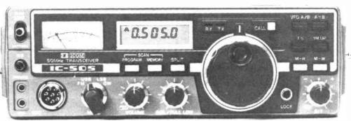
output, 3 watts or 0.5 watts on low power is available when using internal batteries. Other features include 5 memories with memory scan, program band scan, dual VFO's with split operation.
