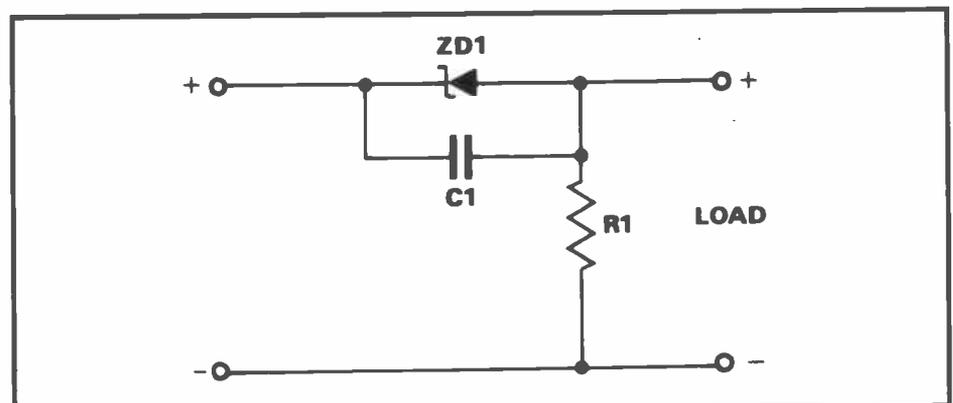
Fig 1: Series dropper circuit
