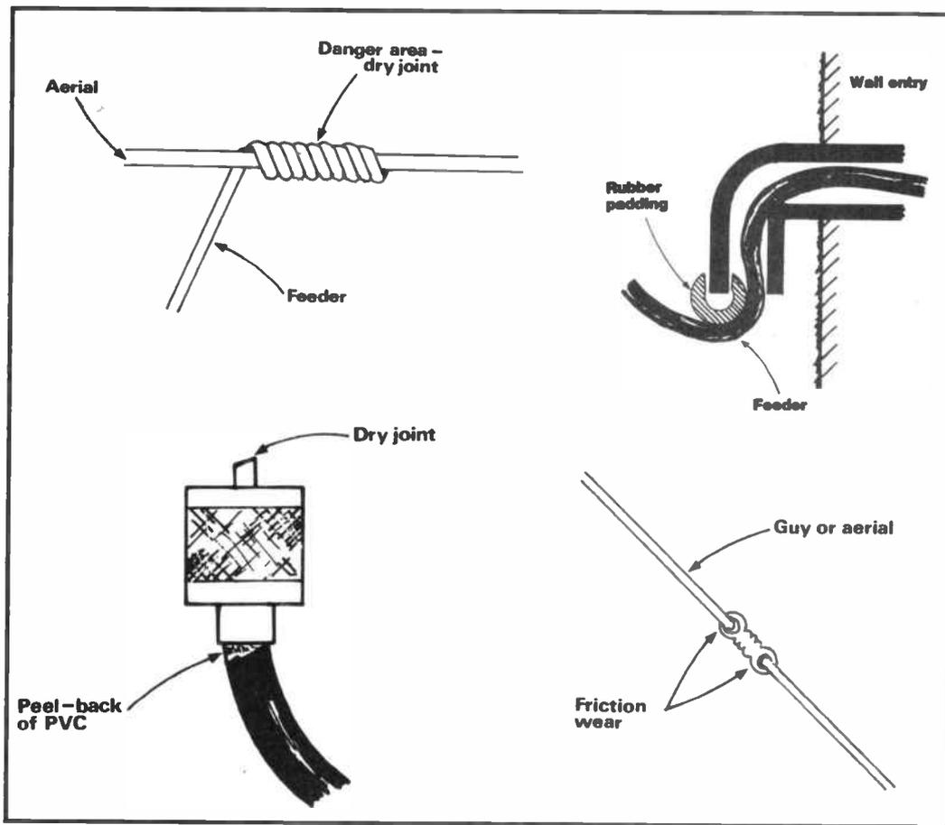
Repairing dry joints and friction wear
