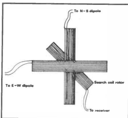
Principle of inductive goniometer. In practice the connections to the rotor would be made via the spindle and sliprings
