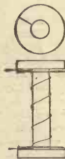
Fig. 3.—Method of Bringing Out Wire Between Paper Washers.
