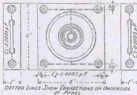
Fig. 2.—Connections of Two Fixed and One Variable Condensers.
