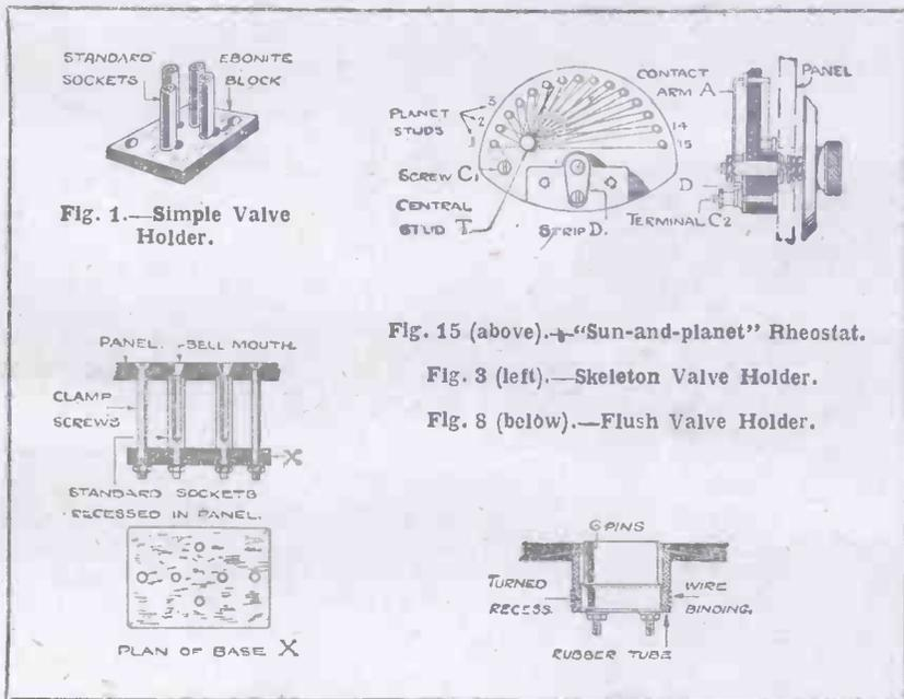
Fig. 1.—Simple Valve Holder.
