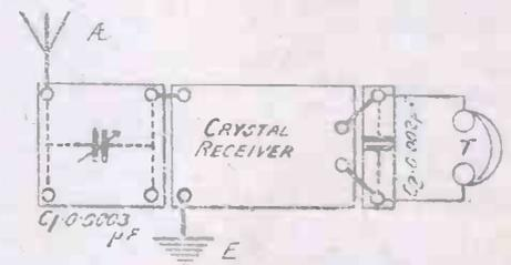
Fig. 5.—Another Method of Adding Condenser Unit.
