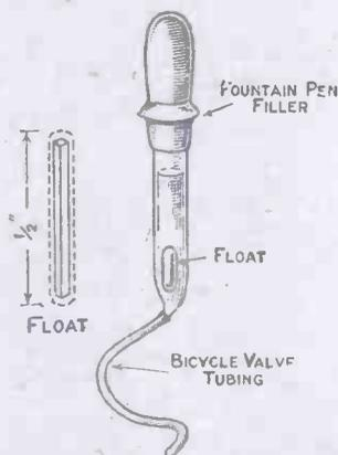
An Easily-made Hydrometer.
