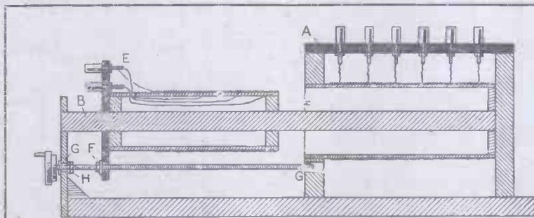
Fig. 1.—Section of Tuner.
