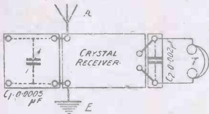
Fig. 4.—Method of Adding Condenser Unit.
