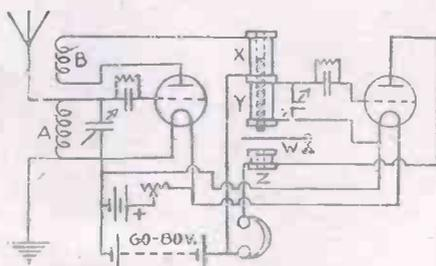
Fig. 3.—Circuit showing Arrangement of L.F. Transformer Reaction.
