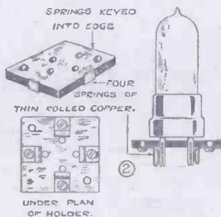
Fig. 2.—Valve Holder for Use in Limited Space.
