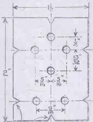
Template for Valve and Coil Sockets.
