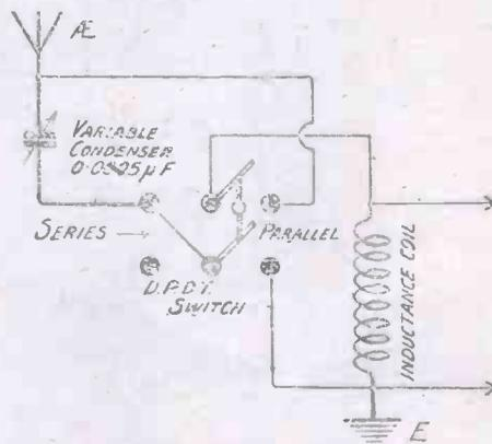
Fig. 6.—Circuit Including Series-parallel Condenser.
