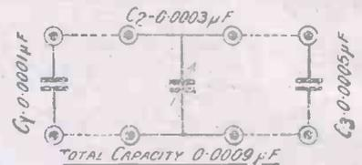
Fig. 3.—Theoretical Circuit of Fig. 2.
