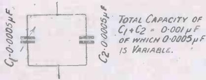
Fig. 1.—Condensers in Parallel.
