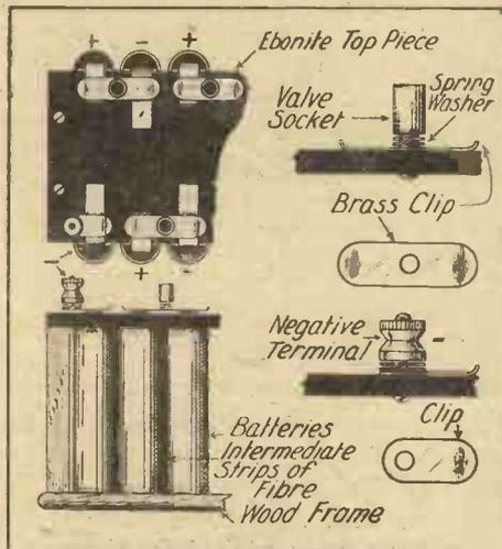
Diagrams showing Assembly Details of the Battery.
