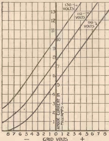
Fig. 4.—Three Curves of the Stentor Two Valve. Note the long straight portions.
