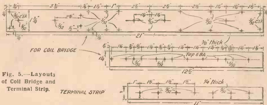
Fig. 5.—Layouts of Coil Bridge and Terminal Strip.
