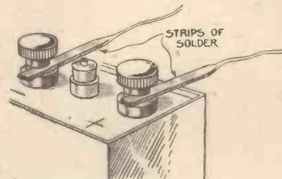
Non-corroding Battery Leads.
