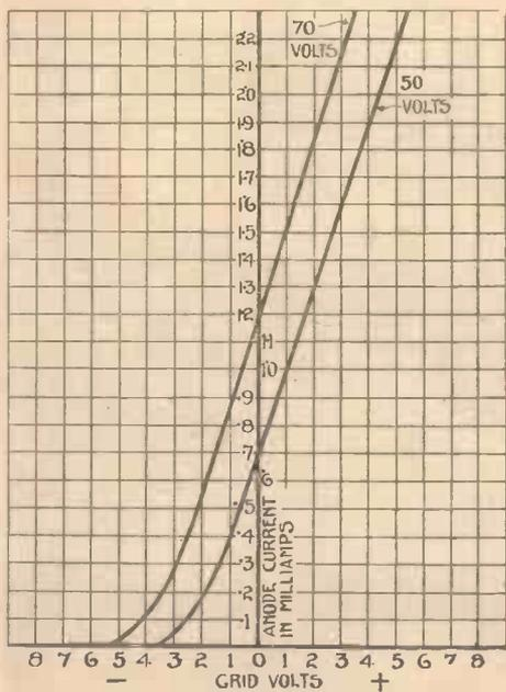
Fig. 2.—Curves Illustrating the Excellent Amplifying Properties of the Red Top Valve.
