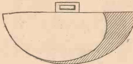
Fig. 2.—Diagram showing Alteration to Condenser Plates.
