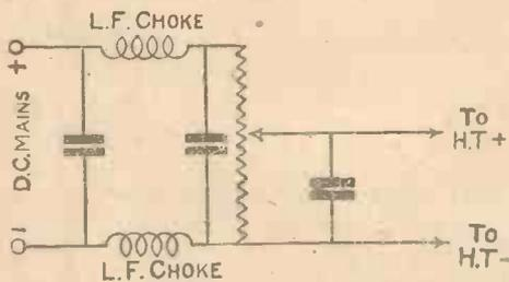
Fig. 4.—Circuit Arrangements for Obtaining H.T. from D.C. Mains.
