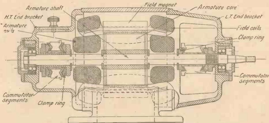
Fig. 3.—Vertical Section of Rotary Transformer.
