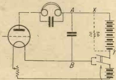
Connections for Battery Switch.
