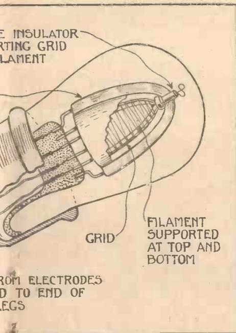
Features in the Construction of the New Valve.
