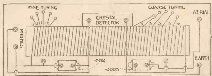
Fig. 3.—Details of Connections
