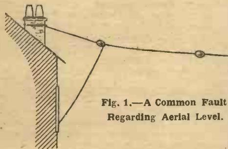
Fig. 1.—A Common Fault Regarding Aerial Level.
