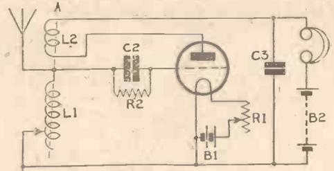
Fig. 2.—Single-valve Receiver with Reaction.
