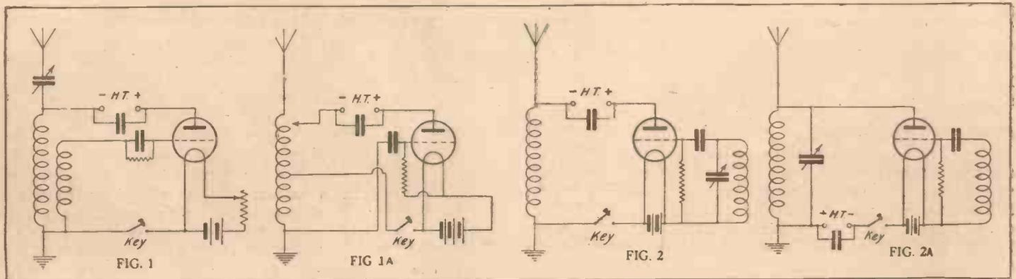
Fig. 1.—Reversed Feed-back Circuit.
