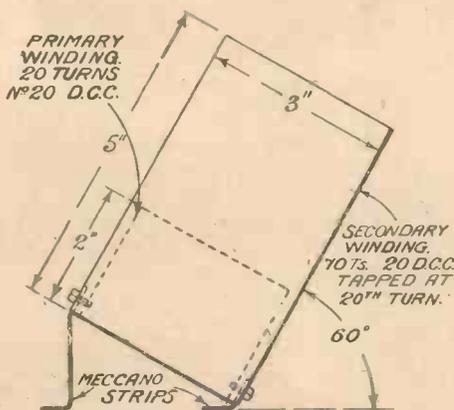
Fig. 1.—A Good Design for a 300-500 m. H.F. Transformer.
