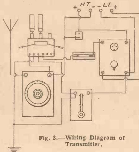
Fig. 3.—Wiring Diagram of Transmitter.
