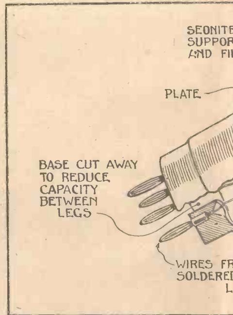
Fig. 1.—This Diagram shows the Special Features of the New Valves.
