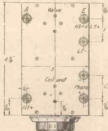
Fig. 3.—Plan showing Layout of Panel.
