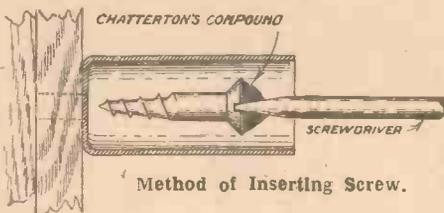
remedy. A loop of wire could also be used to hold the screw in position, but if the screw head is attached to the end of the screwdriver with a little Chatterton's compound it is not necessary to hold the screw.
