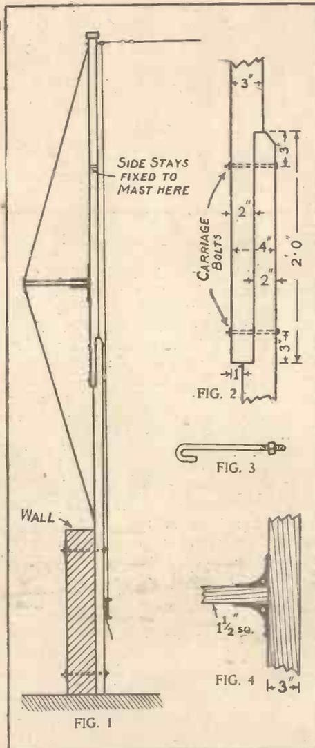
Fig. 1.—The Complete Mast. Fig. 2.—Details of Joint. Fig. 3.—Bolt for Securing Pulley. Fig. 4.—Method of Attaching Strut.
