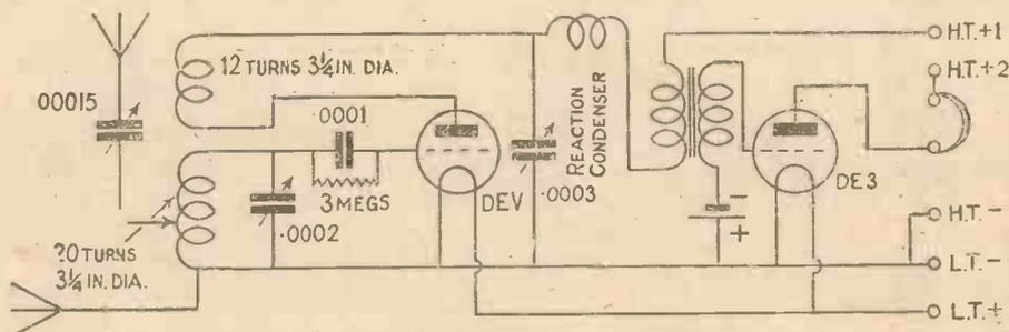
Circuit Diagram of a Good Short-wave Receiver.
