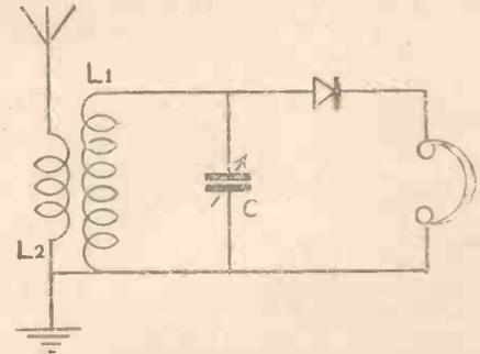
Fig. 5.—In this Circuit a Double-circuit Tuner is Used, the Aerial Being Aperiodic.
