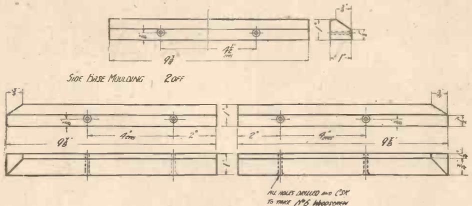
Fig. 7.—Details of Moulding for Base.
