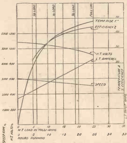
Fig. 9.—Graph of Test Performance of 25-watt Rotary Transformer.
