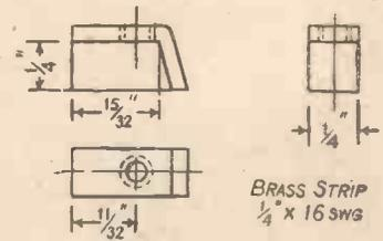
Fig. 4.—Details of Brackets for Securing Panels.
