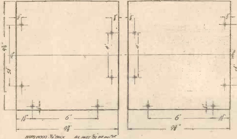
Fig. 5.—Details of Sides.
