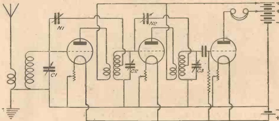
Fig. 2.—A Neutralised H.F. and Detector Circuit.
