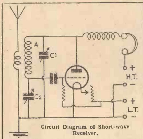
Circuit Diagram of Short-wave Receiver.
