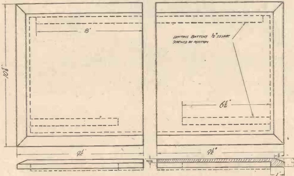
Fig. 6.—Plan and Elevation of Top.
