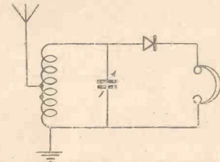
Fig. 4.—The Use of an "X" Coil will Also Improve Results without Altering the Wiring of the Set.
