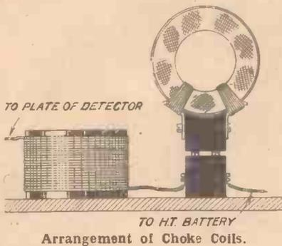
One solution of the difficulty is to construct a separate choke coil for the short waves by winding 100 turns of No. 36 d.c.c. copper wire on an ebonite former 3 in. in diameter and 2 in. long. The small choke is then wired permanently in series with a 500-turn plug-in coil, the latter being short-circuited when receiving on the 45-metre band. B. H.
