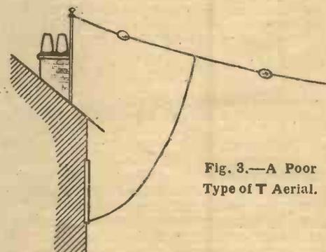
Fig. 3.—A Poor Type of T Aerial.
