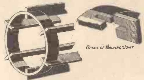
Construction of Low-loss Coil Former.
