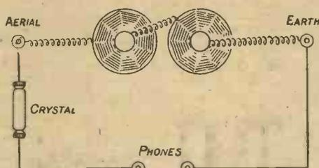
Fig. 6.—The Circuit Diagram for all the Sets.
