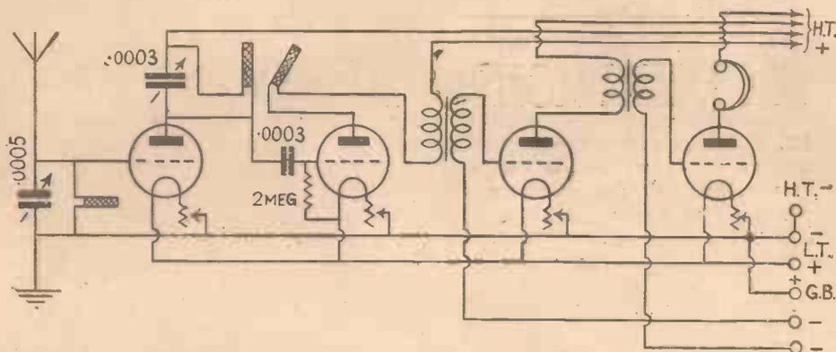
Fig. 3.—Circuit Diagram of the Improved Receiver.
