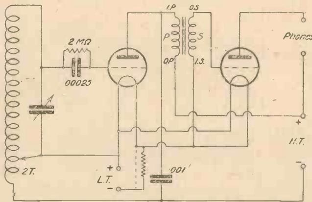
Fig. 1.—Circuit Diagram of Two-valve Portable Receiver.
