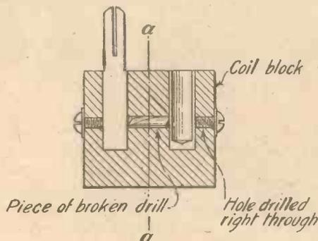
Section of Coil Holder showing Fault.
