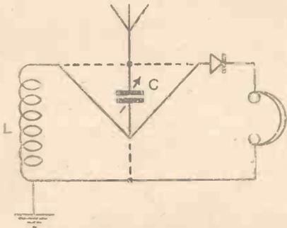
Fig. 3.—Placing the A.T.C. in Series Usually Improves Selectivity (original parallel connections are shown dotted).
