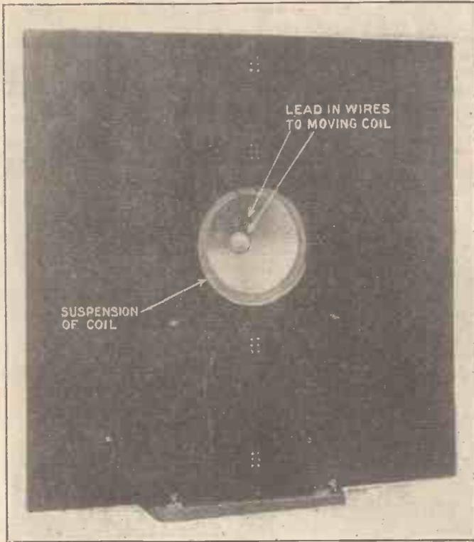
Fig. 3.—Front of McLachlan Loud-speaker with Wooden Board in position.
