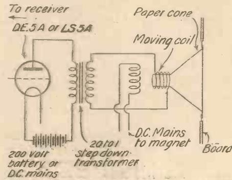
Fig. 5.—Circuit of Power Valve and Connections from Mains for Operating Loud-speaker.
