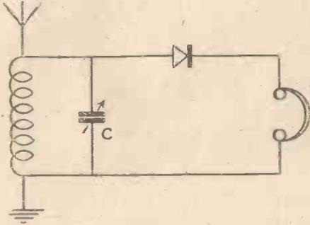
Fig. 1.—The Most Common Type of Crystal Circuit.
