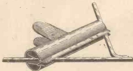
Use of Paper Clip when Soldering.
