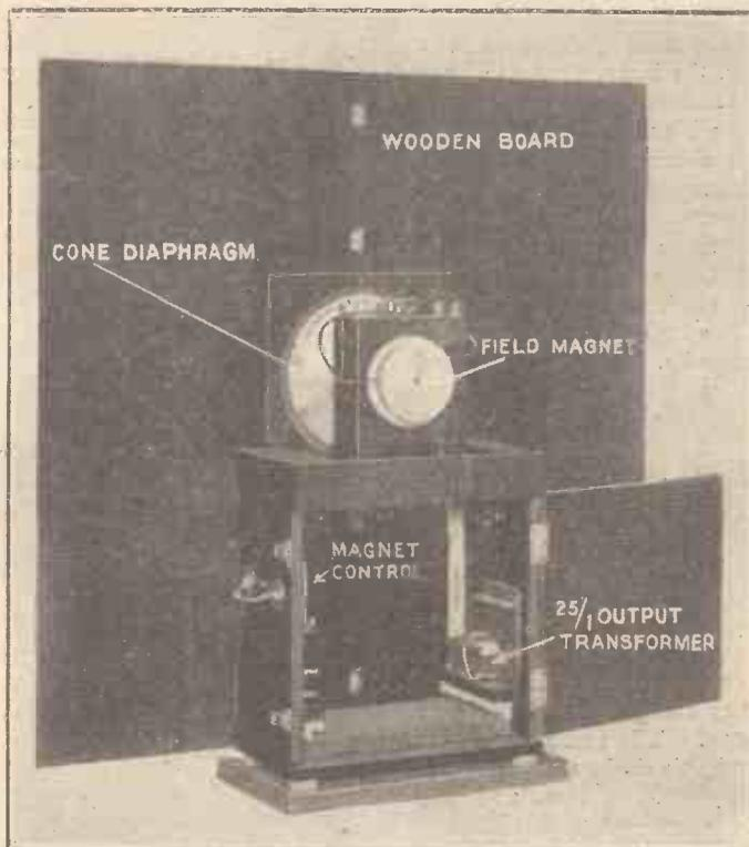
Fig. 2.—Rear of Loud-speaker with Wooden Board in place to Isolate the Two Sides of the Diaphragm.
