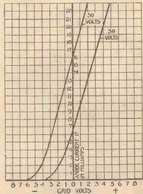
Fig. 3.—The Curves of the Plain Top Valve show its Usefulness as a First-stage L.F. Amplifier.
