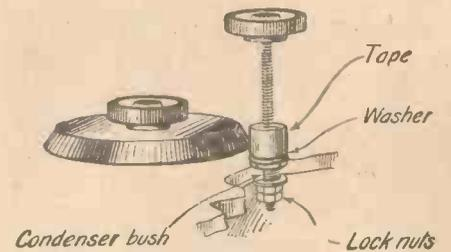
Vernier Adjustment for Condenser.
