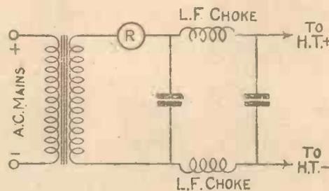
Fig. 5.—Circuit Arrangements for Obtaining H.T. from A.C. Mains.
