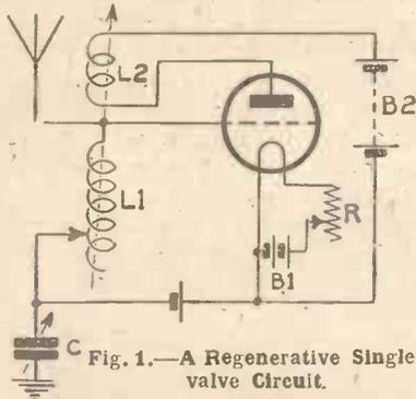
Fig. 1.—A Regenerative Single-valve Circuit.
