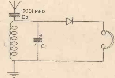
Fig. 2.—A Small Fixed Condenser in Series with the Aerial will Improve Matters.
