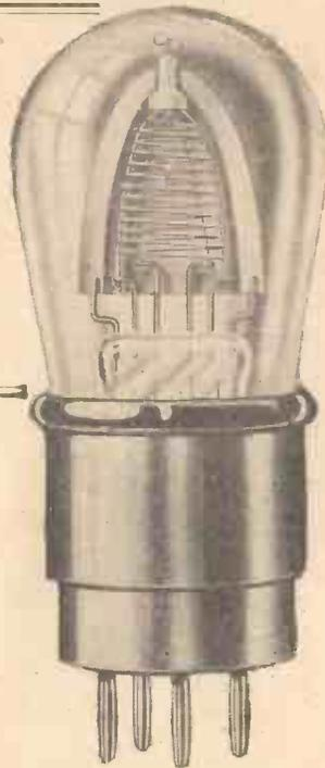
The co-axial method of mounting the three electrodes is clearly seen here.
