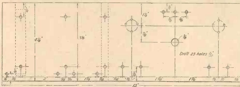
Fig. 2.—Layout of Panel.
