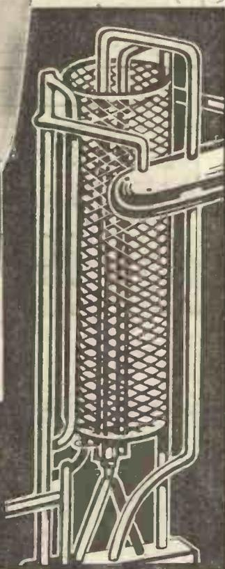
**NOTE** the gauze anode which assists in the ready dissipation of heat and maintains the initial efficiency of the valve throughout a long and useful life.
