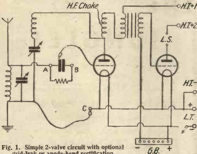
Fig. 1. Simple 2-valve circuit with optional grid-leak or anode-bend rectification
