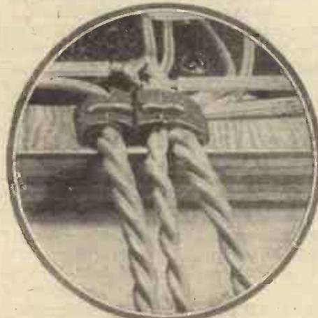
**Terminals need not always be used. H.T., L.T. and G.B. leads can be twisted into groups and connected direct to the batteries**
