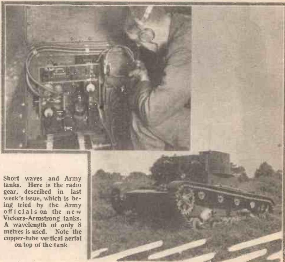
Short waves and Army tanks. Here is the radio gear, described in last week's issue, which is being tried by the Army officials on the new Vickers-Armstrong tanks. A wavelength of only 8 metres is used. Note the copper-tube vertical aerial on top of the tank
