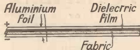
This diagram shows the constructional features of the paper dielectric condenser.
