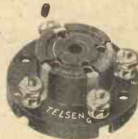
TELSEN FOUR-PIN VALVE HOLDER. PRICE 1/- each. TELSEN VALVE HOLDERS. Pro. Pat. No. 20286/30. An entirely new design in Valve Holders, embodying patent metal spring contacts, which are designed to provide the most efficient contact with the valve legs, either split or NON-split. Low capacity, self-locating, supplied with patent soldering tags and hexagon terminal nuts.
