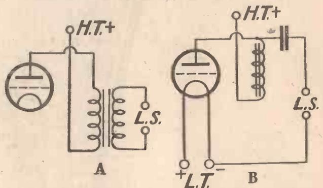
Fig. 5 (A) Transformer output (B) Choke output
