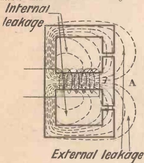
Fig. 1. Magnetic system of moving-coil speaker showing disposition of the flux
