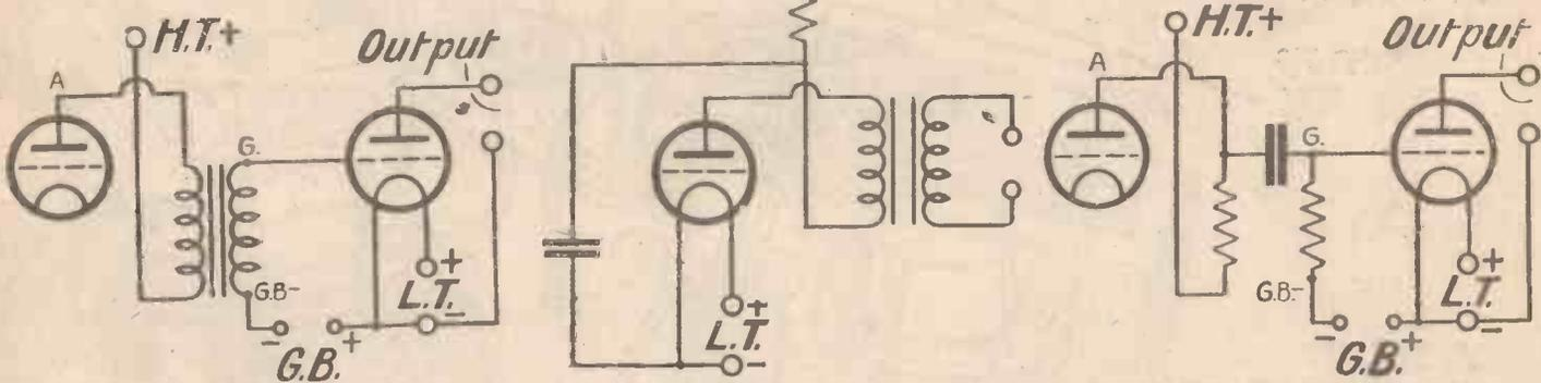
Fig. 2. Two valves coupled by transformer Fig. 4. How a de-coupling arrangement is incorporate1 Fig. 3. Resistance-capacity L.F. coupling
