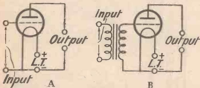
Fig. 1 (A). A skeleton valve amplifying circuit. (B) Transformer coupling arrangement for L.F. valve
