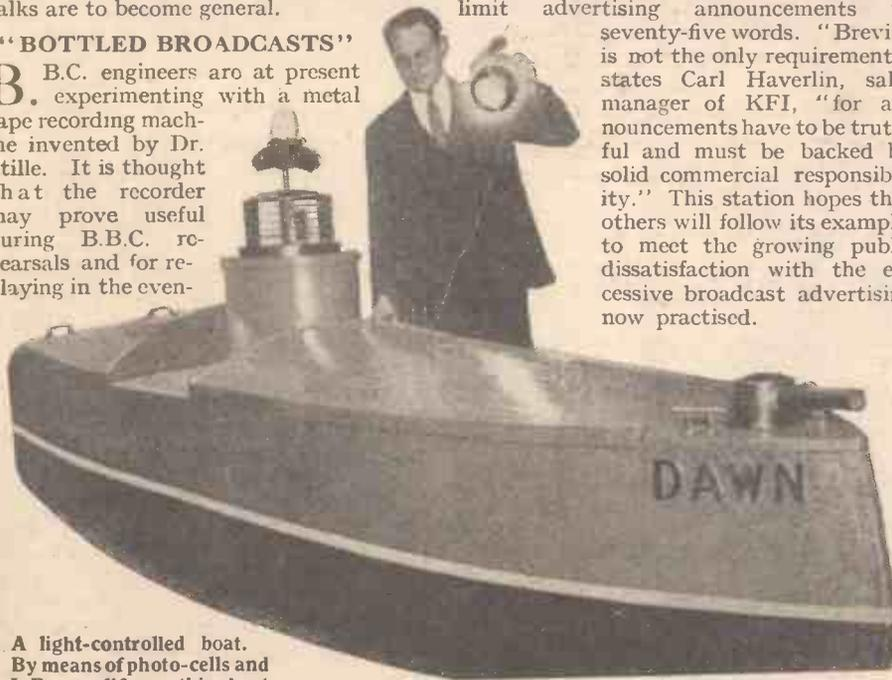
A light-controlled boat. By means of photo-cells and L.F. amplifiers this boat has actually been controlled, and the gun fired, at a distance of several thousand yards
