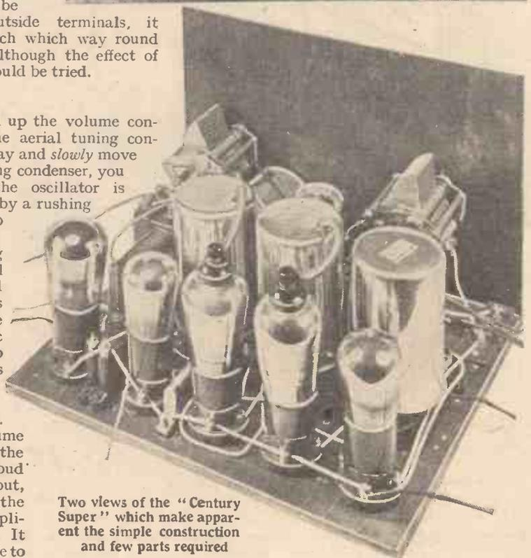
Two views of the "Century Super" which make apparent the simple construction and few parts required
