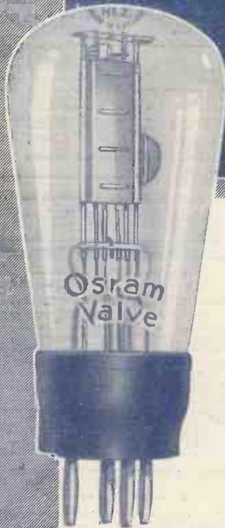
**T**HIS is an entirely new 2-volt general purpose valve. Its outstanding feature is its "mica bonded" electrode system wherein the electrodes are locked or bonded together in a mica template, making for absolute rigidity which gives consistency in characteristics between valve and valve, and freedom from microphonic or parasitic noises. The valve is, therefore, most suitable for use in Portable Receivers as a highly efficient Detector — or first stage Low Frequency Amplifier.
