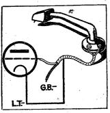
Earthing the shielded pick-up wiring
