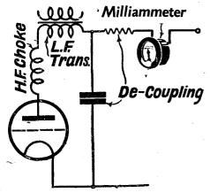
This skeleton circuit shows the correct position for the insertion of a low-reading milliammeter to ensure correct ganging. Note the meter is connected to the hightension-positive end of the detector circuit
