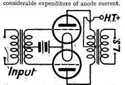
Fig. 1. An ordinary push-pull circuit
