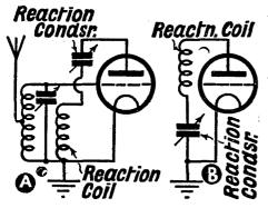
The two reaction arrangements, A and B, referred to
