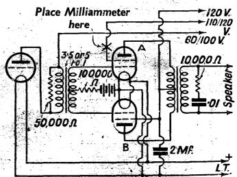
Fig. 2. This circuit is a modification of the first, employing pentode valves and capable of a large output
