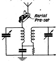
The aerial pre-set in this circuit of a bandpass input to a high-frequency stage is used for adjusting the aerial load, and not for varying the volume
