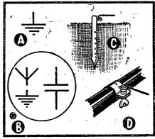
At A is the symbol for the earth connection. At B you will see how the aerial and earth are considered as the two plates of a condenser, with the intervening air as the di-electric. At C is a common form of earth contact—a buried spike or tube. At D is an alternative earth contact-a main water pipe
