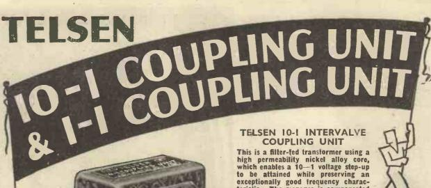
exceptionally good frequency characteristic. The response is compensated in the higher frequencies for use with a pentode valve, this combination giving an amplification greater than
