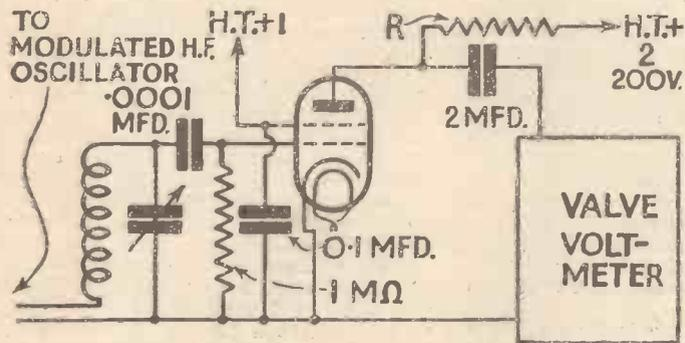
Fig. 1. A typical screen-grid detector circuit using cumulative grid rectification. The anode resistance should be 20,000 to 50,000
