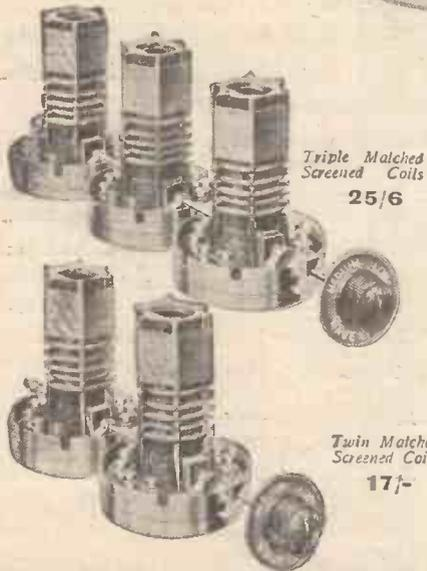
Full instructions are supplied with every Telsen Screened Tuning Coil, showing you the alternative methods of mounting the coils, either singly or in twin-matched or triple-matched form, as required.
