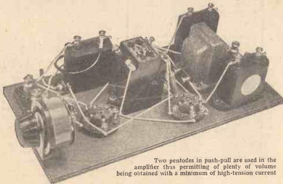
Two pentodes in push-pull are used in the amplifier thus permitting of plenty of volume being obtained with a minimum of high-tension current
