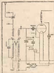
Tune in a station at the top of the medium wavelength band—say the Northern Regional. Note the signal level. Now connect a Telsens Mica Condenser (up to .0003 mfd. in value) across the aerial tuning condenser. Decrease the value of the
