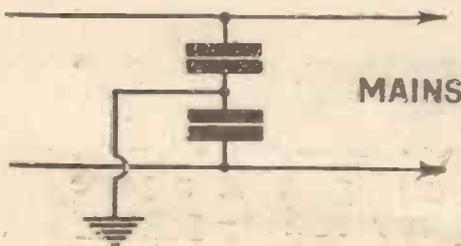
Fig. 1. A simple filter circuit to by-pass H.F. interference on electric light wires. The centre connection between the two condensers is earthed
