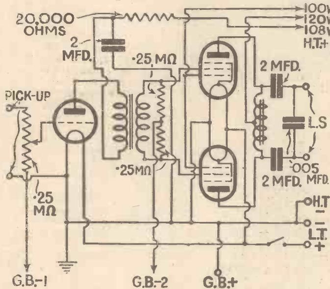
Although this amplifier has pentodes in push-pull, the circuit is quite simple. The input transformer has quarter-megohm leaks across the secondary, to avoid the necessity for a special tapped secondary transformer, and the output is taken through a choke and double condenser arrangement, so that no tapped output transformer is needed. These are factors which make the amplifier cheap to build.
