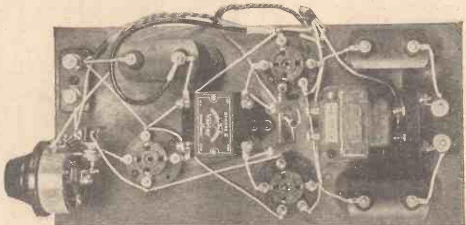
This plan view shows the simple construction of the amplifier, with all the components mounted on a baseboard
