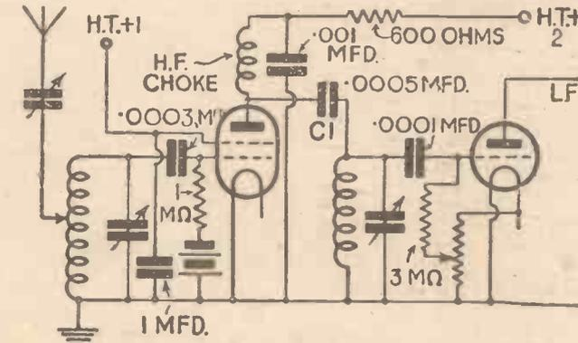
Fig. 1. A good short-wave circuit in which a screen-grid valve is used
