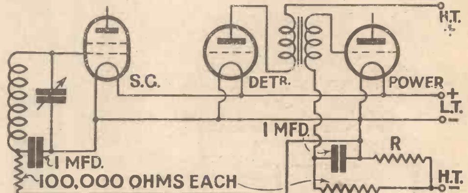
This is a typical three-valve circuit in which automatic bias is applied by means of voltage-dropping resistances
