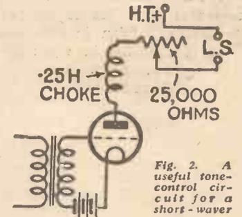
Fig. 2. A useful tone-control circuit for a short-waver
