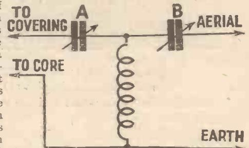
Fig. 2. A filter circuit which is put between the sheathed aerial and the set. A is the tuning condenser and B the coupler
