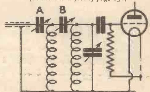
Fig. 3. A complete circuit using the sheathed aerial and the filter shown by Fig. 2
