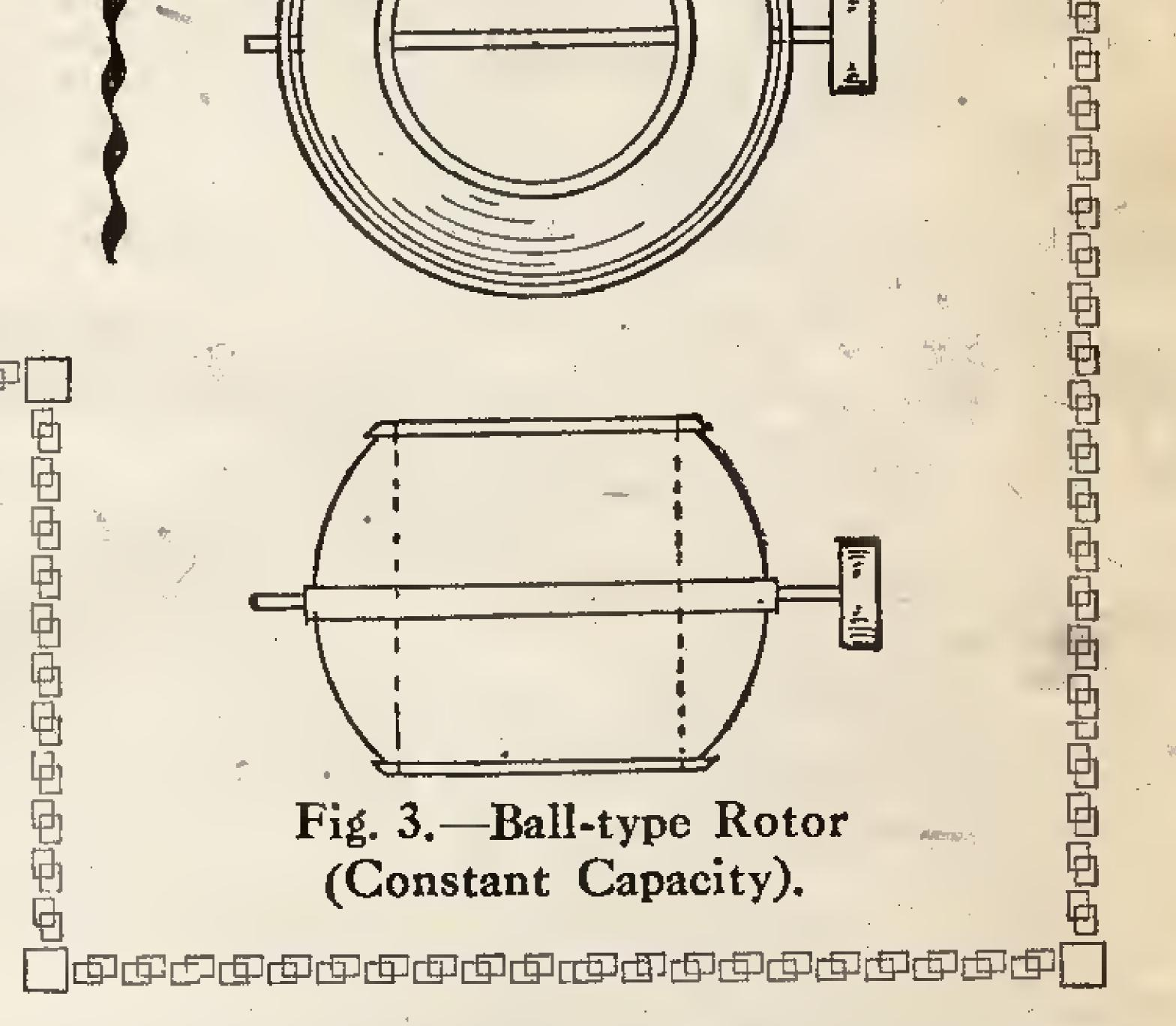
ing must be put on in two parts and joined at the centre, as it is only possible to wind "up the hill." The winding should be started at each end and continued upwards (inwards), and the two ends then soldered together and tucked inside.
