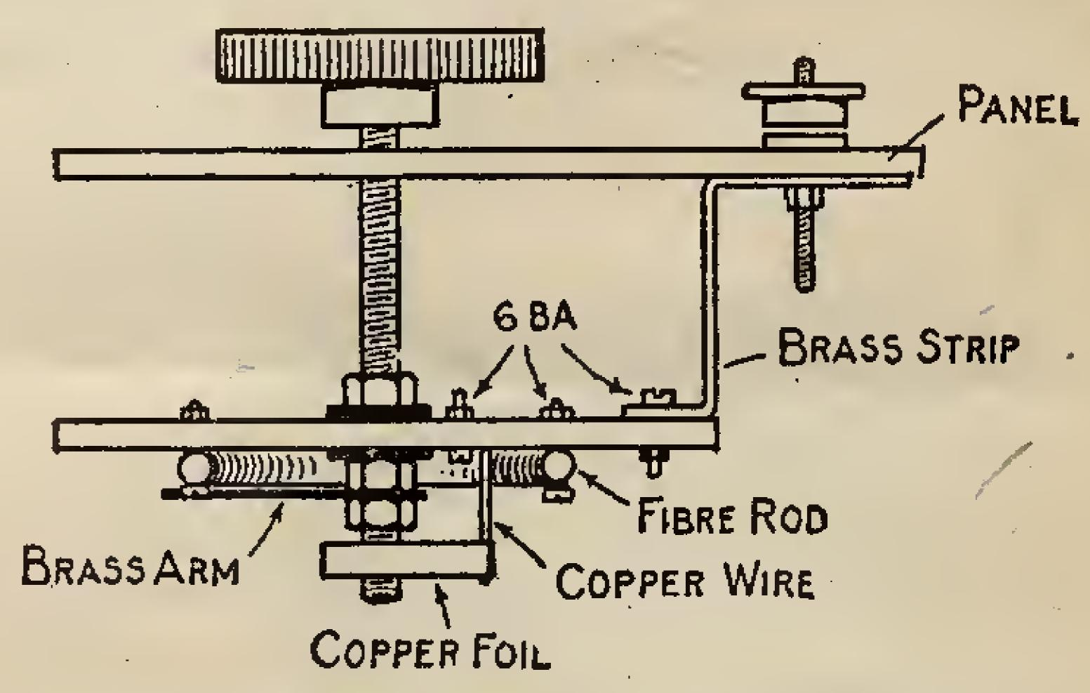
Fig. 3.—Enlarged Detail of Filament Rheostat.
