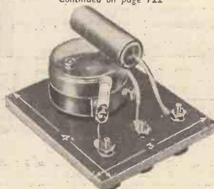
Fig. 3.—Here is an under-panel view of a simple beam deflector of which the circuit and values are given by Fig. 4
