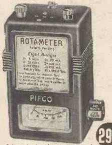
Radio testing is made easier, quicker and more accurate by the Pifco ROTAMETER Any one of eight dials are brought into view by turning the octagonal knob at the side of the instrument. Size of each dial 13 by \$\frac{1}{2}\$ in. Convenient in size and of amazing accuracy. Finished in black bakelite, complete with leads, in velvet-lined case.
