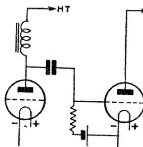
Fig. 3.—Choke-capacity coupling
