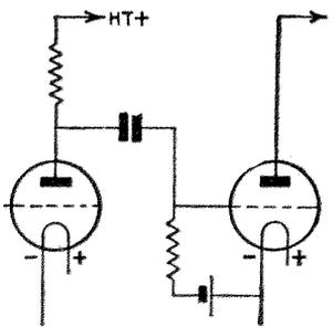
Fig. 2.—Resistance-capacity coupling
