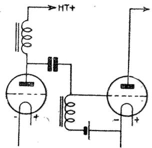
Fig. 4.—Dual-impedance coupling
