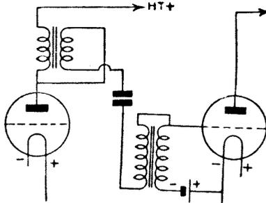
Fig. 7.—Auto-transformer-fed auto-transformer coupling
