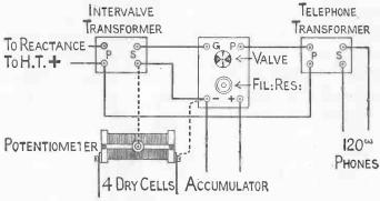
Fig. 47.-Method of Connecting Intervalve Transformer.
