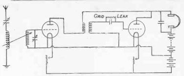
Fig. 82.—High-frequency Air-core Transformer Coupling.
