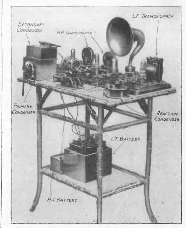
Fig. 66.—Photograph of the Units Arranged as a Four-valve Receiver.
