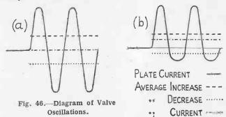
the average increase in the plate current greater than the average decrease or vice versa. It will be seen from Fig. 46 that if the average increase is equal to the average decrease, the average plate current will remain the same and the telephone diaphragm will not be affected. When the signals are rectified there is an increase or decrease in the average plate current depending on the connections of the rectifying valve.
