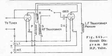
current is from H.T. positive through telephones to stud A, and from thence via the switch arm to stud B or C to the detector valve or L.F. valve according to the position of the switch.
