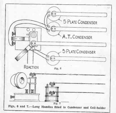
coupling. These small condensers should also be fitted with long handles, and should be left in about the midway position. After getting the best adjustment possible with the large condenser and the reactance coupling as described, finish off with the two small condensers.
