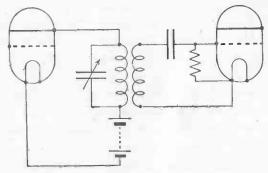
Fig. 48.—Connections of H.F. Transformer.
