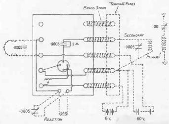
Fig. 79.—Wiring Diagram of Valve-rectifying Panel.
