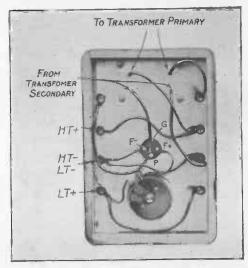
Fig. 86.-Under Side of High-frequency Panel.
