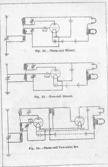
on the secondary, so the coils are from rear to front on photographs, and top to bottom on diagrams, Figs. 52 to 54. (1) Three-coils; (2) two-coil circuit; (3) three-coil two-valve set.
