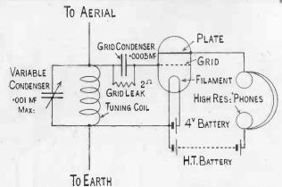
Fig. 2.—Circuit Diagram of Single-valve Set
