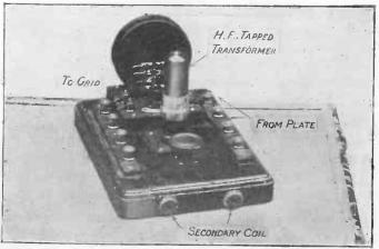
Fig. 70.—High-frequency Transformer-coupled Unit.
