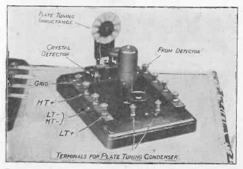
Fig. 68,-Crystal Detector Panel with H.F. Valve and Tuned Plate.
