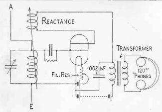
Fig. 4.—Circuit Diagram of Improved Set
