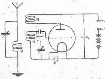
Fig. 29.—Circuit to Prevent Re-radiation.
