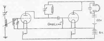
Fig. 83.—Tuned-anode Coupling of H.F. to Rectifying Valve.
