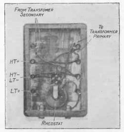
Fig. 78.—Bottom View of Valve-rectifying Panel.
