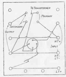
Fig. 87.—Wiring Diagram of H.F. Transformer Panel.
