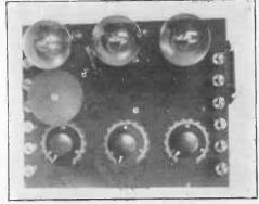
Fig. 57 .- Top View of Three-valve Receiver.
