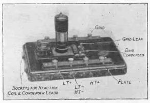
Fig. 77.-Photograph of Valve-rectifying Panel.
