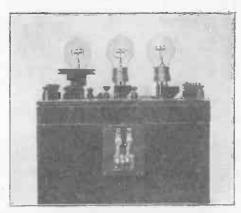
Fig. 56.—Front View of Three-valve Receiver.
