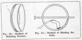
Accurately measure off two 18 ft. lengths of No. 26-gauge wire. Wind one upon the inner and one upon the outer former in a simple close-up layer,
