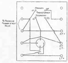
Fig. 91.—Wiring Diagram of Low-frequency Panel.
