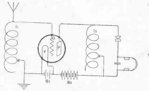
Fig. 8.—Valve as High-frequency Amplifier with Crystal Detector.
