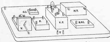
Fig. 30.—Diagram of One-valve Variometer Set.
