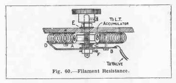
Now take about 3 yd. No. 21 s.w.g. "Chronic" resistance wire and wind it tightly round a lead pencil with the spirals touching. When removed from the pencil the spirals will keep their shape and the coil can be fixed to the ebonite disc in the place allotted to it. The turns of wire should not touch then.
