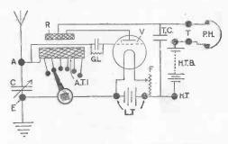
Fig. 45.—Circuit Diagram of Portable Receiver.
