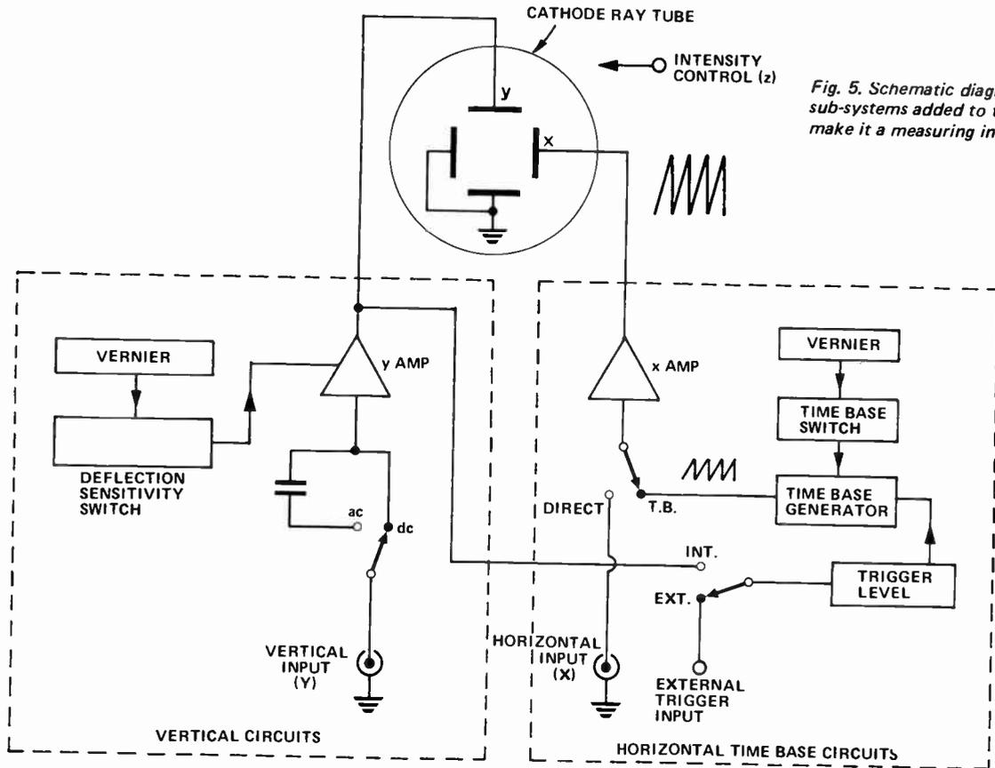
Fig. 5. Schematic diagram of essential sub-systems added to the CR tube to make it a measuring instrument.
