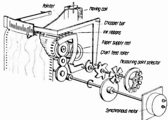
Fig. 11. Dotting recorders offer the advantages in slow-speed applications of being suitable for multi-channel multiplexing.
