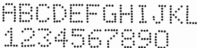
Fig. 7. Alpha-numeric characters as generated by 5 x 7 dot matrix.
