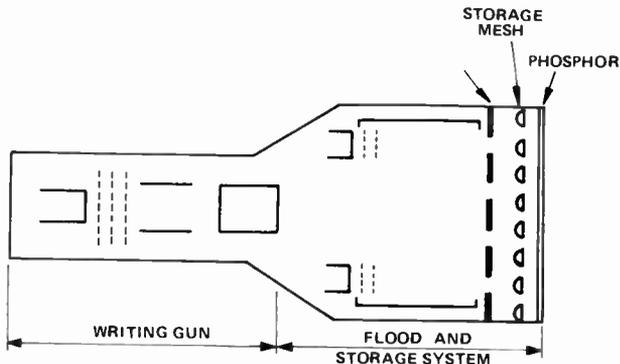
Fig. 2. Schematic construction of storage cathode ray tube.
