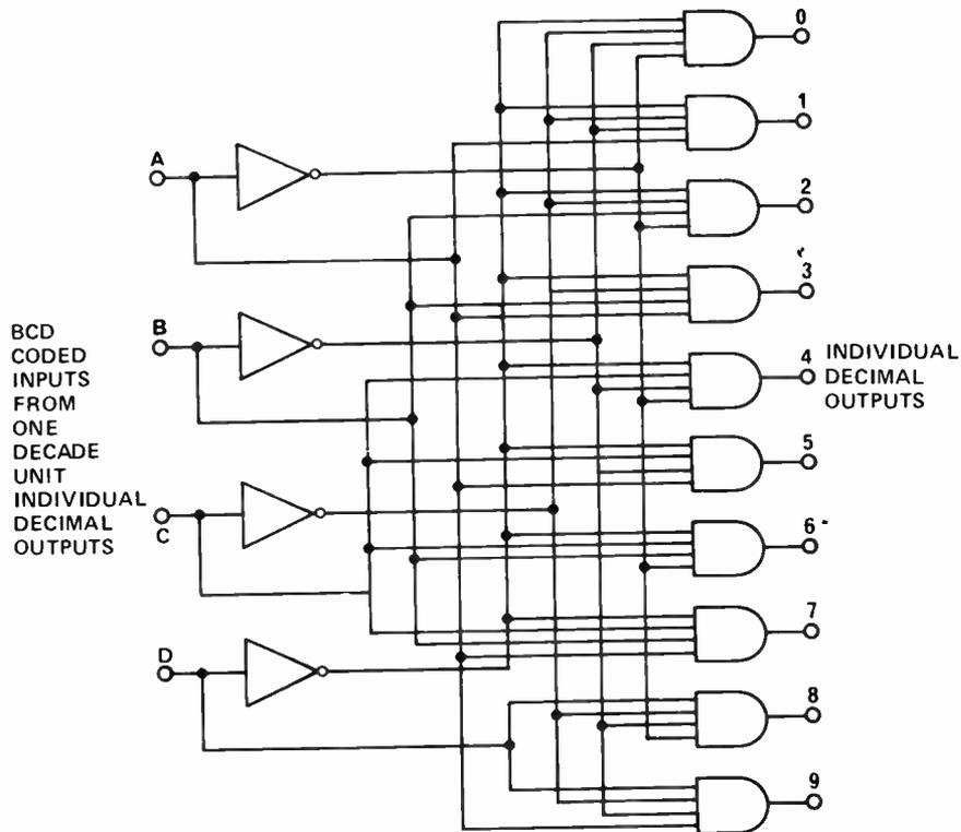
Fig. 6. Logic arrangement for decoding BCD units into one-of-ten outputs.
