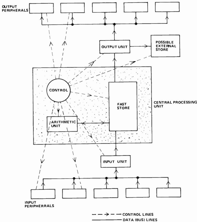
Fig. 14. Basic functional blocks of electronic data processing system.
