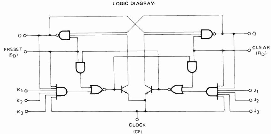
Some flip-flops provided in IC form also may contain three-input AND gates that feed the set and reset inputs. These are known as the J and K inputs giving the name J-K flip-flop. The JK flip-flop overcomes an ambiguous output state, when both inputs are high, that occurs with the RS flip-flop. We will see, when counting systems are discussed, why the reset ability is vital in many counters. Fig. 16 gives the schematics of some of the available flip-flop ICs.
