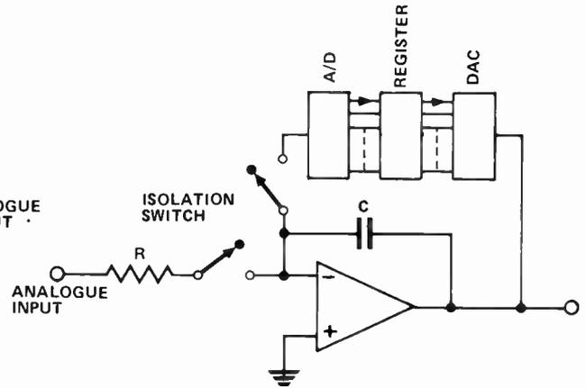
Fig.23. Infinite hold is obtained by transferring the integrated value into a digital store using A/D and D/A conversion.
