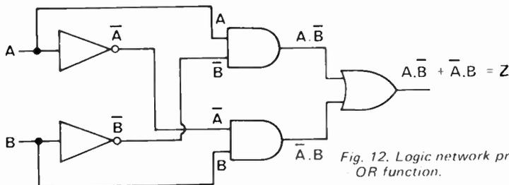
Fig. 12. Logic network providing exclusive OR function.
