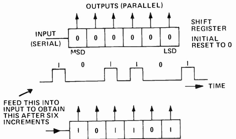
Fig. 8. Registers can provide serial to parallel word conversion, the reverse also applies.
