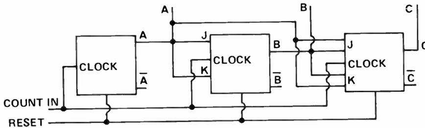
Fig. 3. Synchronous binary up-counting with JK flip-flops.
