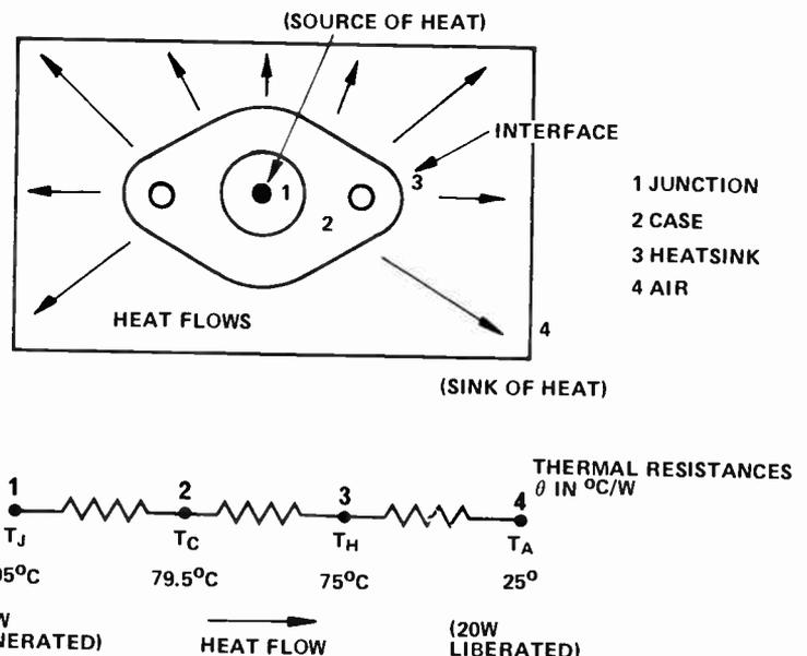
Fig. 2. Thermal resistances for a 20 W power transistor.
