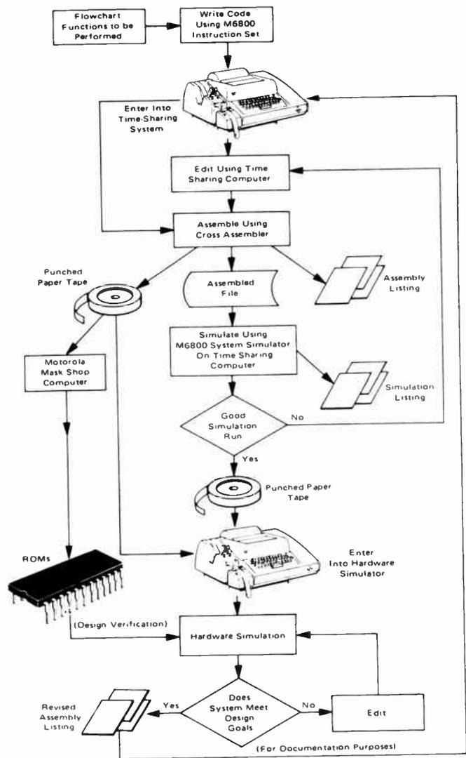
Fig. 19. This flow chart shows how the Motorola Company produces a custom-tailored ROM ready to slip into their M6800 microprocessor system.
