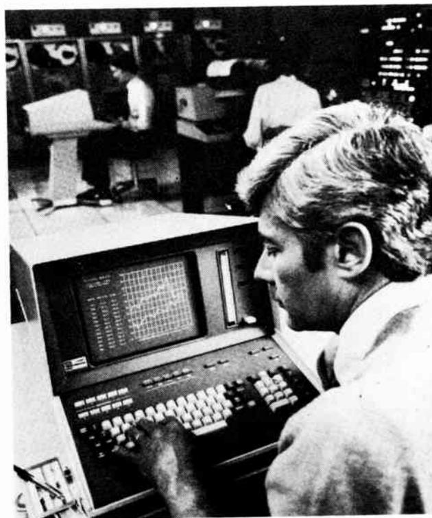
*Fig. 11. Interactive graphic units often now incorporate their own processing and memory to form an off-line self-contained unit — 4051 Tektronix BASIC graphic computing system.*
