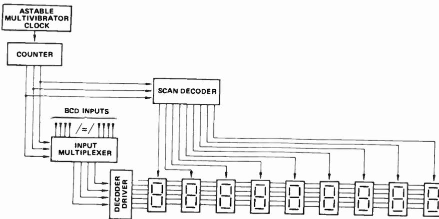
Fig. 16 Schematic of a multiplexing system for use with a multidigit, 7-segment display.
