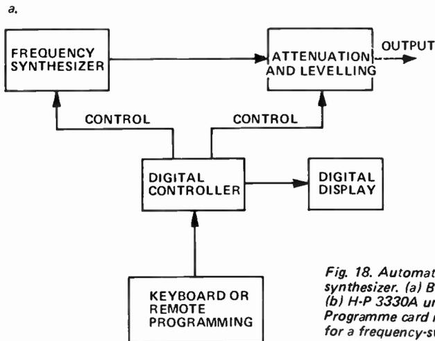
Fig. 18. Automatic frequency synthesizer. (a) Block diagram. (b) H-P 3330A unit. (c) Programme card marked up for a frequency-sweep routine.
