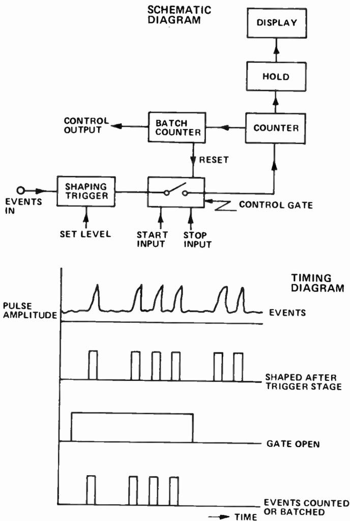
Fig. 9. Schematic diagram of totalizing and batching use of counter with display.
