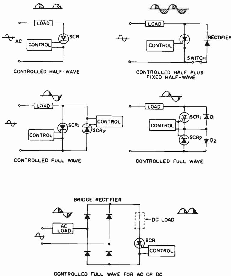
Fig. 5. Five arrangements by which a load can be fed with power flow controlled by SCR devices.
