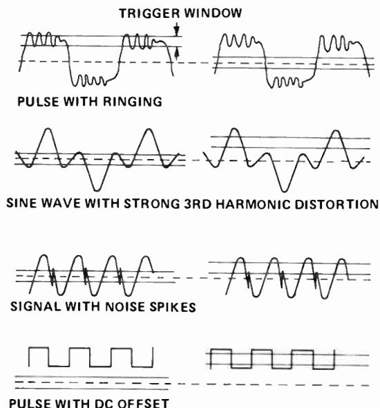
Fig. 14. Trigger height for the window must be chosen to suit the wave shape.
