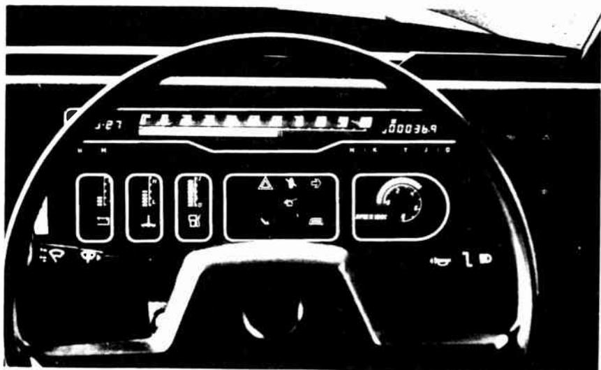
Fig. 6. On-vehicle electroluminescent display dash panel (Smiths Industries).
