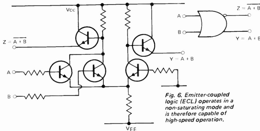
Fig. 6. Emitter-coupled logic (ECL) operates in a non-saturating mode and is therefore capable of high-speed operation.
