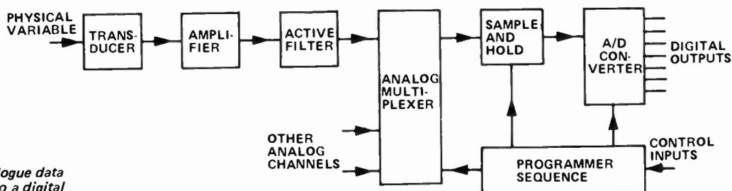
Fig. 2. Typical layout of an analogue data acquisition system interfacing to a digital output.
