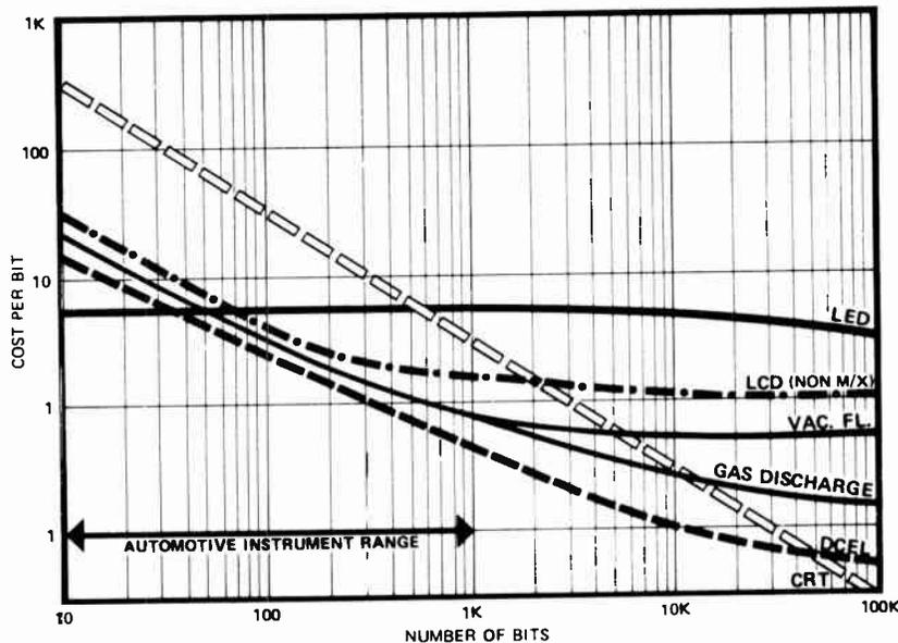
Fig. 3. Comparison of the cost per bit of the various display options.
