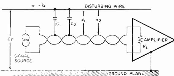
Fig. 14. Twisted wires provide best common-mode rejection when making connections between stages in which a symmetrical signal source is joined to a differential input amplifier.
