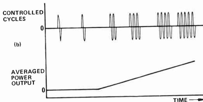
Fig. 7. (a) Zero-voltage-switching temperature controller using a zero voltage switching IC driving a TRIAC from a thermistor sensor. (b) Output signal with gradually increasing power.
