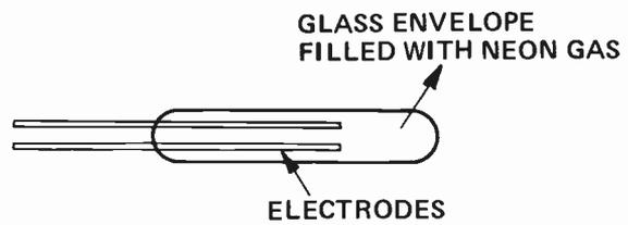
Fig. 3a. Construction of the basic neon lamp. b. How a multi-digit neon indicator is constructed from an anode grid and ten separate character-shaped cathodes.
