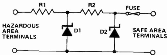
Fig. 9. Circuit used in a Zener barrier.
