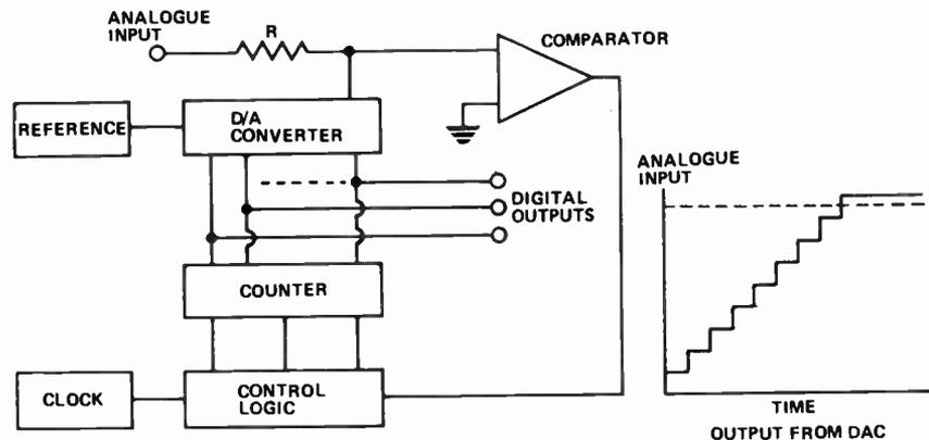
Fig. 20. Schematic of servo A/D converter system.
