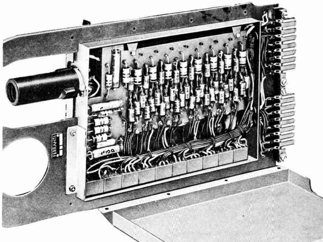
*Fig. 8. Compact electronic computer systems become reality when valves were replaced by solid-state components. This single plug-in unit, from a Pegasus computer of the 50s, would today have its entire function made on a pinhead in LSI technology.*
