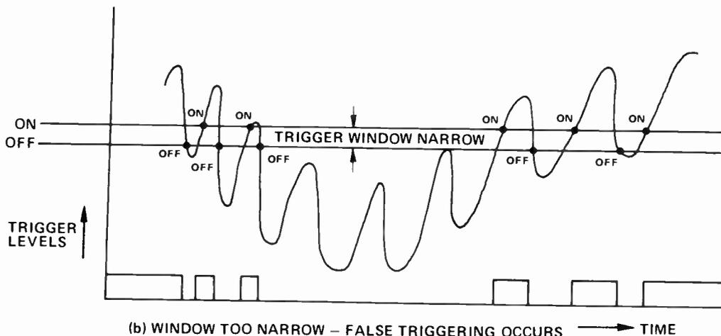
a time just shorter than the expected interval. This is known as trigger masking. It is very useful in eliminating contact-bounce retriggers.
