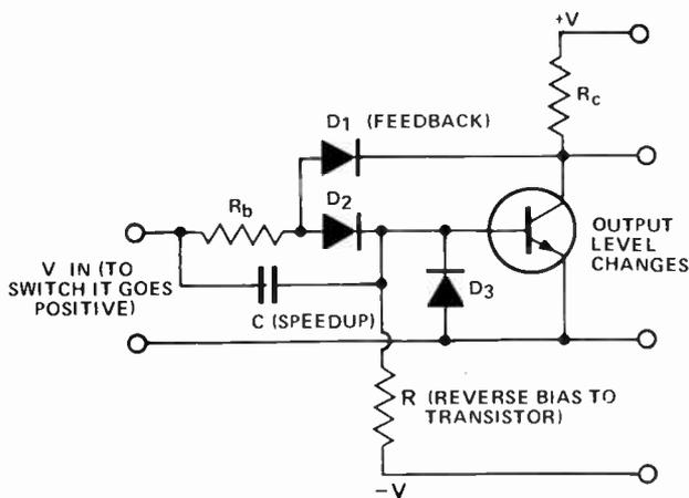
Fig. 11. High-speed switches are designed to remain non-saturated. This circuit employs feedback D1 with D2 providing a voltage supply needed. The speed-up capacitor is C. Diode D3 assists reduce the delay time.
