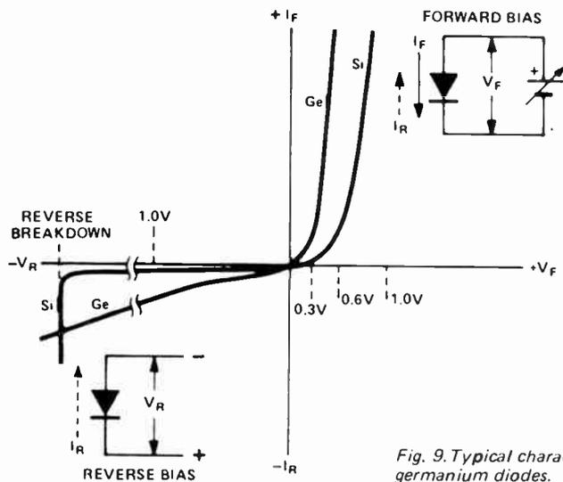
Fig. 9. Typical characteristics of silicon and germanium diodes.
