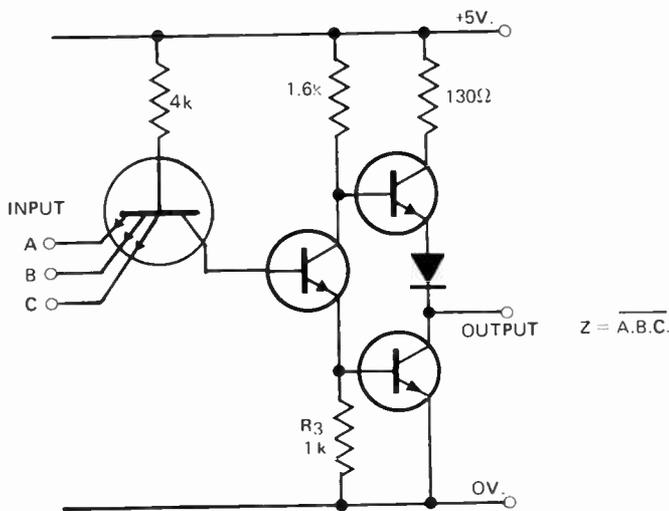
Fig. 4. In the TTL (transistor-transistor logic) form of NAND gate a multi-emitter transistor replaces the diodes of DTL.
