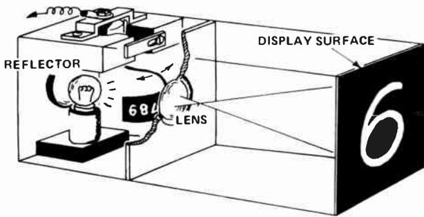
Fig. 2. The moving-coil numerical character display is based on an optical projection system. The numbers are on a graticule which is rotated behind a lens by a meter-line movement. (Drawing courtesy of Electronics Australia).
