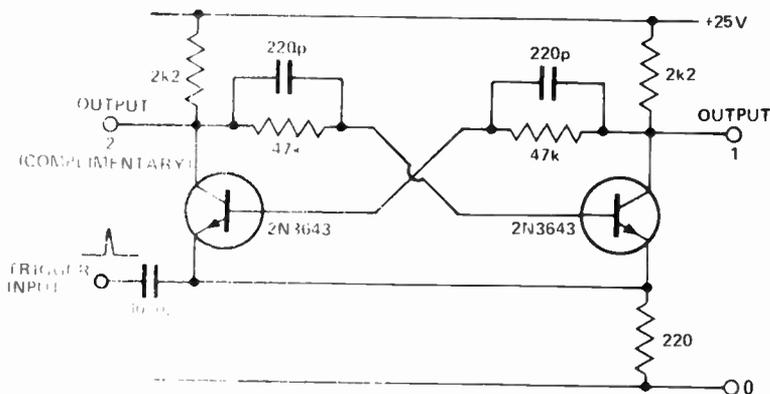
Fig. 13. A basic flip-flop built with discrete components.
