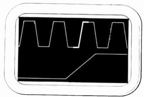
Fig. 9. Trace brightening is used to show which part of the waveform is to be expanded. In this display the expanded portion is also displayed on the second trace of the CRO.
