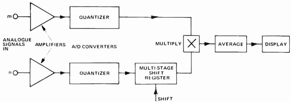
Fig. 17. The simplified block diagram of an auto correlator.
