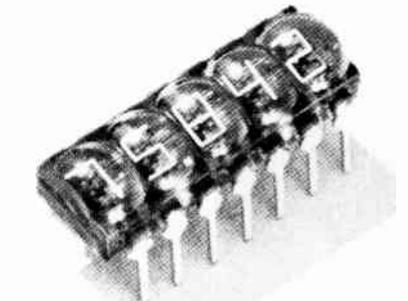
Fig. 13. Some seven-segment displays suitable for calculators etc are assembled in groups and have plastic lenses to increase character size.
