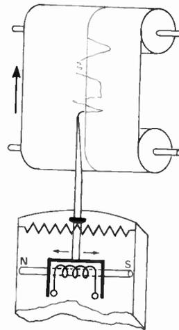
(b) Schematic using linear motor.
