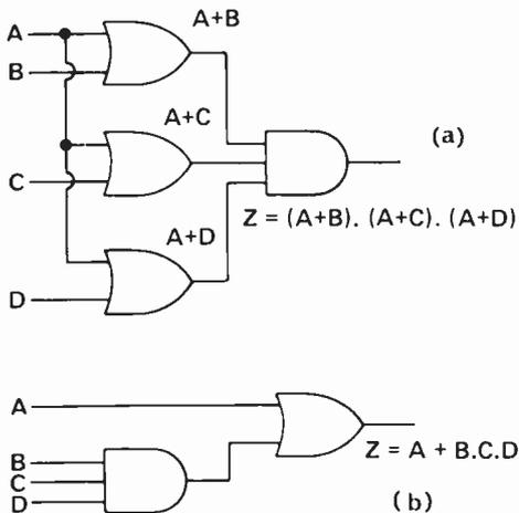
Fig. 16. Logic network realising  $Z = (A + B) \cdot (A + C) \cdot (A + D)$
