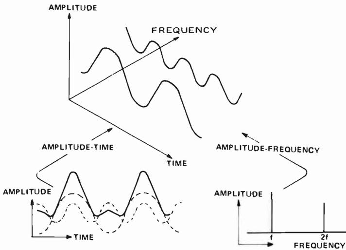
Fig. 8. Second harmonic distortion is not always easily seen on an amplitude versus time display. In the amplitude versus frequency display the second harmonic distortion and its amplitude are clearly seen.
