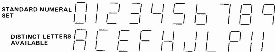
Fig. 5. Format of seven-segment numeric and alphabetic characteristics.
