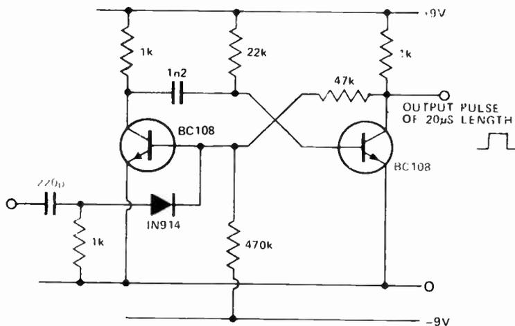
Fig. 17. A basic monostable constructed with discrete components.
