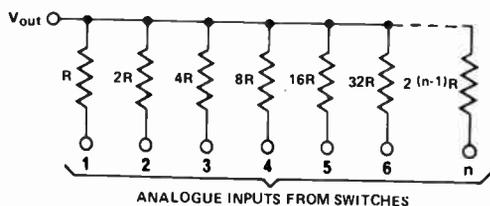
Fig.5. Basic binary-weighted resistance sequence.
