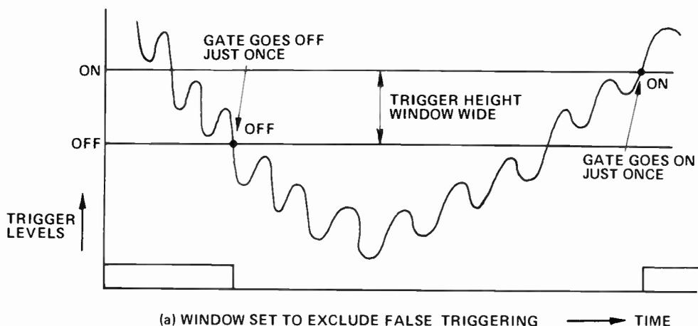
Fig. 13. Noise reduction in counting by use of a trigger height window.
