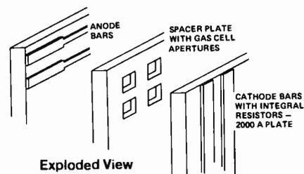
Fig. 4. Construction of dot-matrix gas-discharge display unit.
