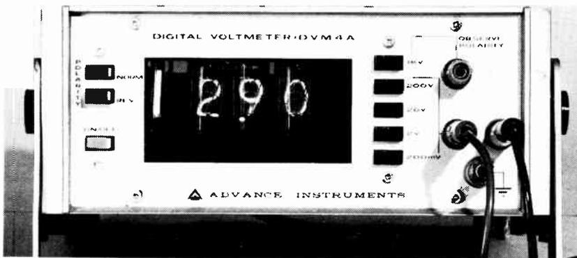
Fig. 1. This typical digital multimeter uses a neon-indicator tube display.
