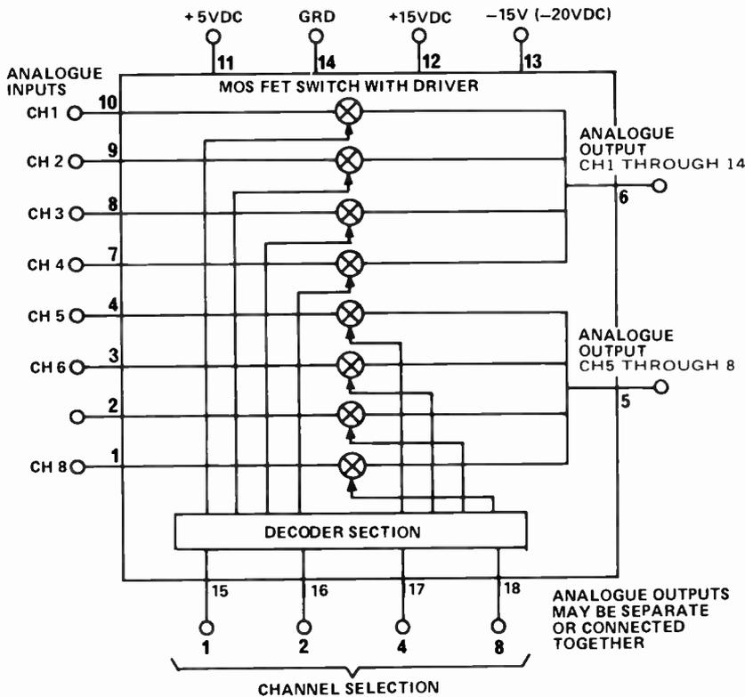
Fig.25. Internal schematic of Datel 8 channel, MM-8 multiplexer.
