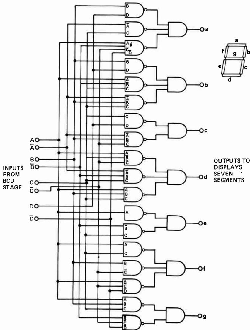
Fig. 7. Logic for converting BCD to seven-segment display format.
