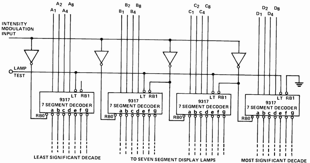
Fig. 12. Connections for ripple blanking in a four-decade display system. (RBO ripple blank output, RBI ripple blank input).
