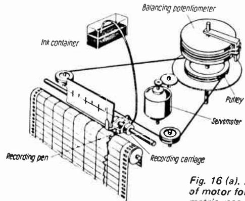
Fig. 16 (a). Arrangement of motor form of potentiometric recorder.
