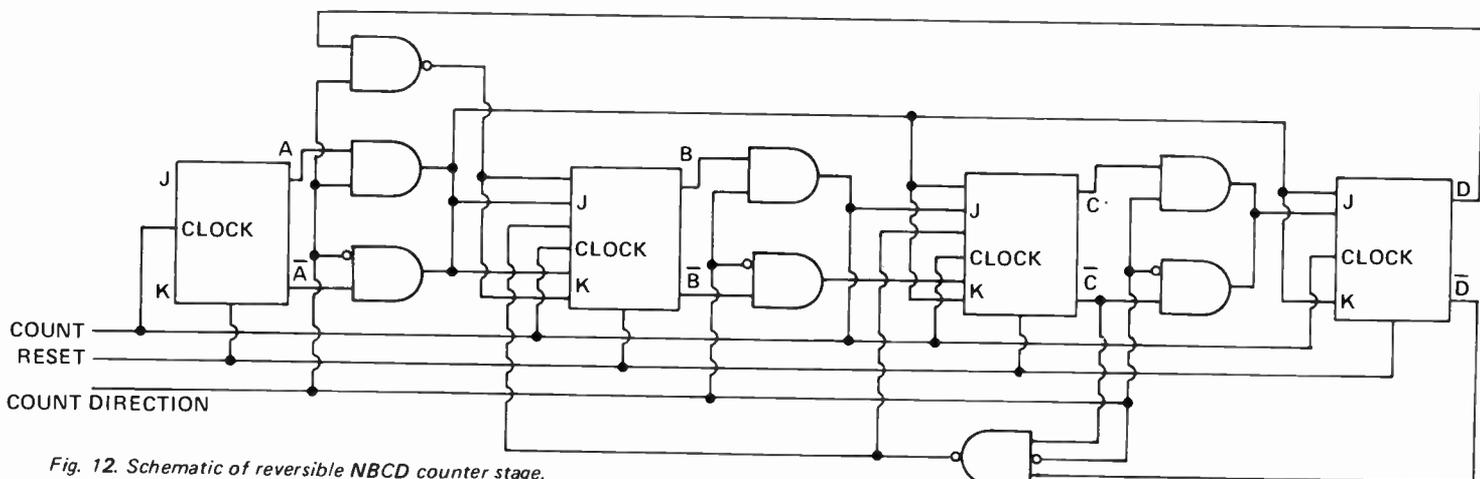
Fig. 12. Schematic of reversible NBCD counter stage.
