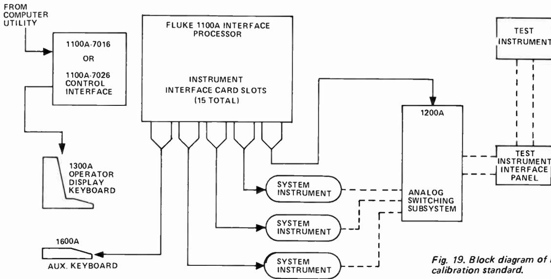
Fig. 19. Block diagram of Fluke calibration standard.
