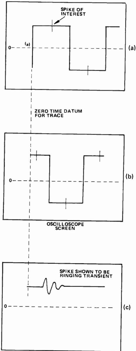
Fig. 8. Use of introduced delay in triggering to enable an event away from trigger transient to be investigated. (a) Original spike on pedestal of square wave. (b) Delay introduced to bring spike back to time origin. (c) Scale expanded to reveal true nature of spike.
