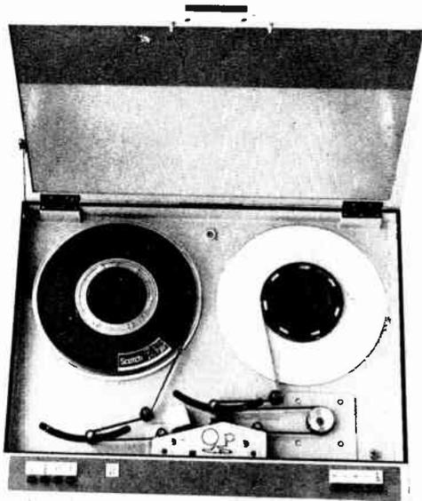
Fig. 15. The Hewlett-Packard 7970 magnetic tape unit designed as a peripheral to EDP systems.
