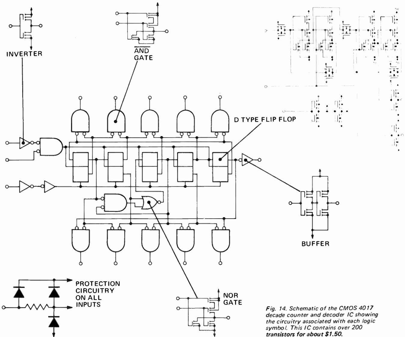
Fig. 14. Schematic of the CMOS 4017 decade counter and decoder IC showing the circuitry associated with each logic symbol. This IC contains over 200 transistors for about \$1.50.
