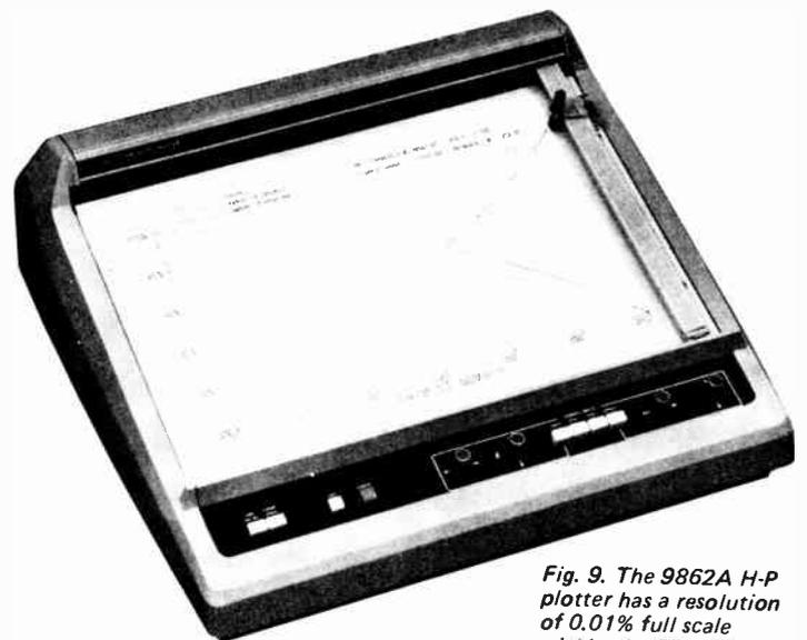
*Fig. 9. The 9862A H-P plotter has a resolution of 0.01% full scale within the 25 x 38 cm area. It will plot vectors at 30 cm per second.*
