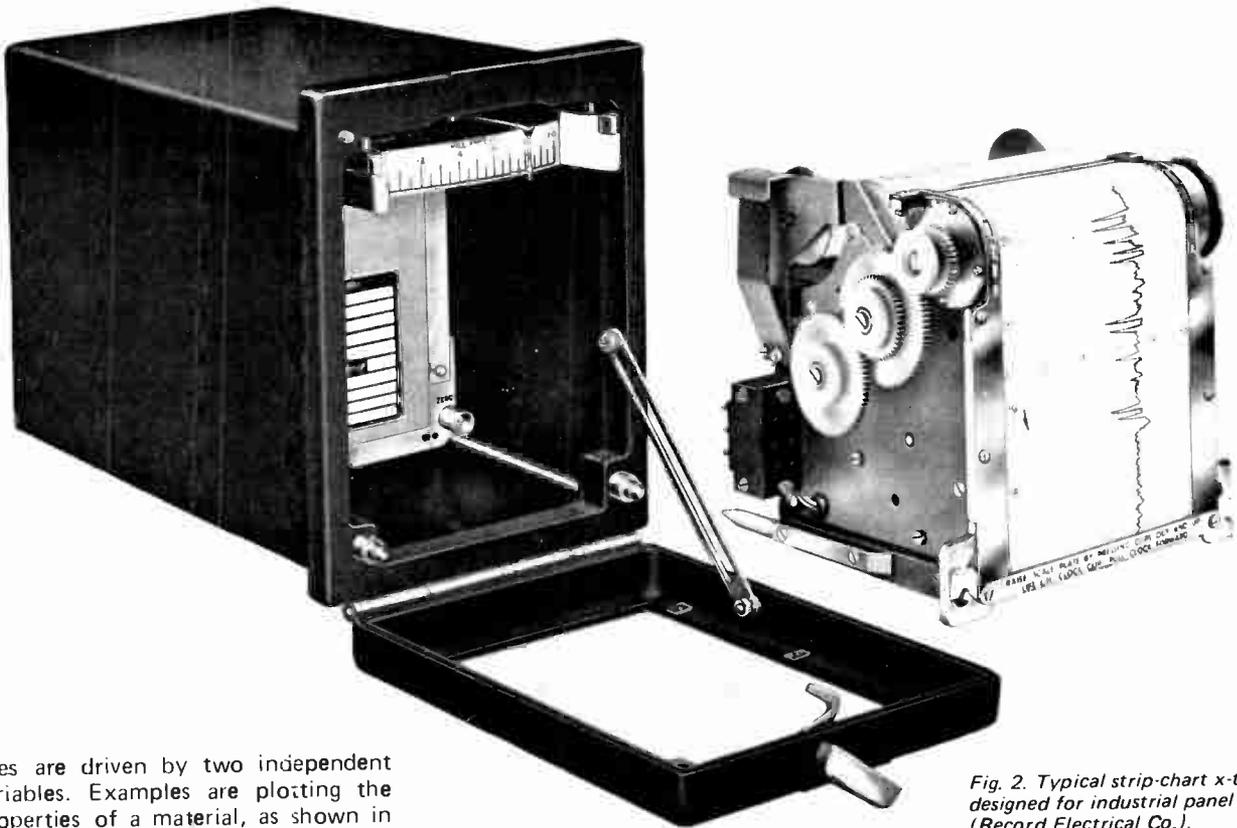
Fig. 2. Typical strip-chart x-t recorder designed for industrial panel mounting. (Record Electrical Co.).
