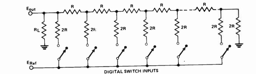
Fig.6. The R-2R ladder network requires only two values of resistance and presents constant impedance to the output.
