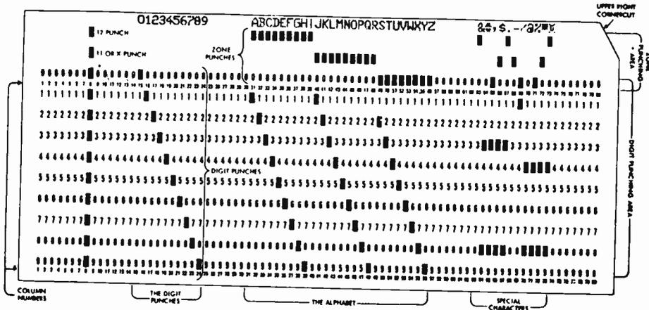
Fig. 1. Standard Hollerith Code used for punched cards.
