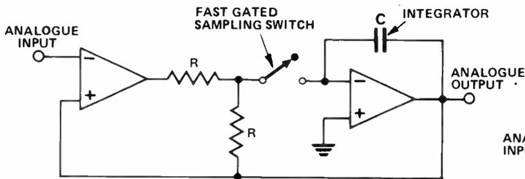
Fig.22. One form of stable and accurate sample-and-hold circuit.
