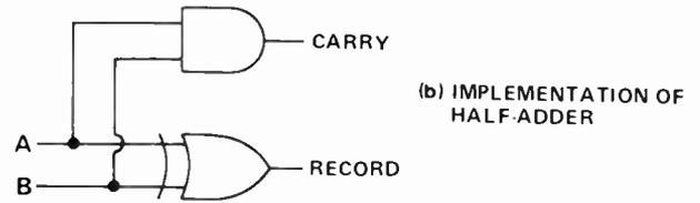
Fig.15 (b). One form of half-adder logic network.
