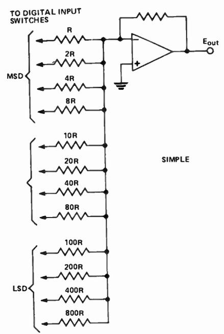
Fig. 7. Resistance layout of R2R, BCD ladder D.A.C.
