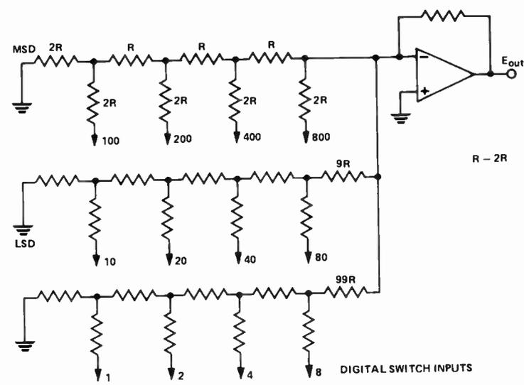
Fig. 7. Resistance layout for simple BCD-weighted DAC.
