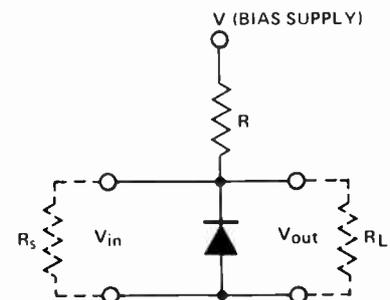
Fig. 8. Diode wired to provide shunt switching action.
