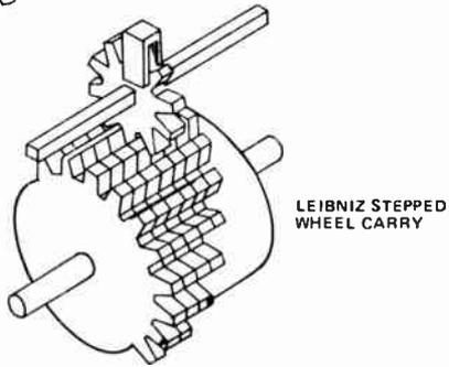
Fig. 10. Pascal's calculator of 1642 used stripped-gear toothed-wheels to produce a carry to the next decade: The Leibniz machine made use of the stepped wheel.
