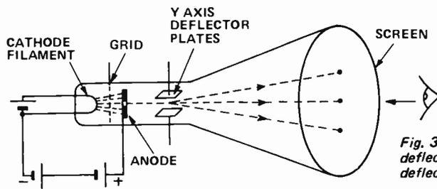
Fig. 3. The electron beam can be deflected by voltages applied to deflection plates.
