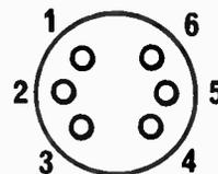
Underneath view. Note that pins 1 and 3 are internally connected as are pins 4 and 6. Polarity is not important.
