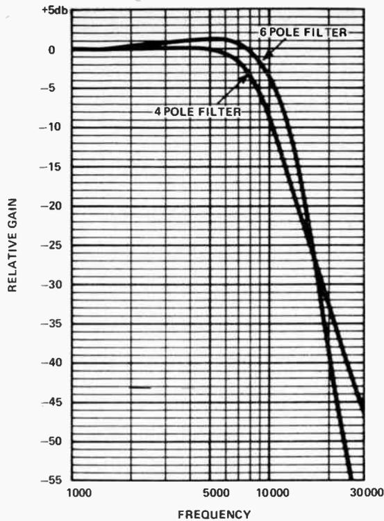
Fig. 3. The frequency response of the two filters. The overall response is approximately the sum of these two filters provided the clock frequency is at least 20 kHz.
