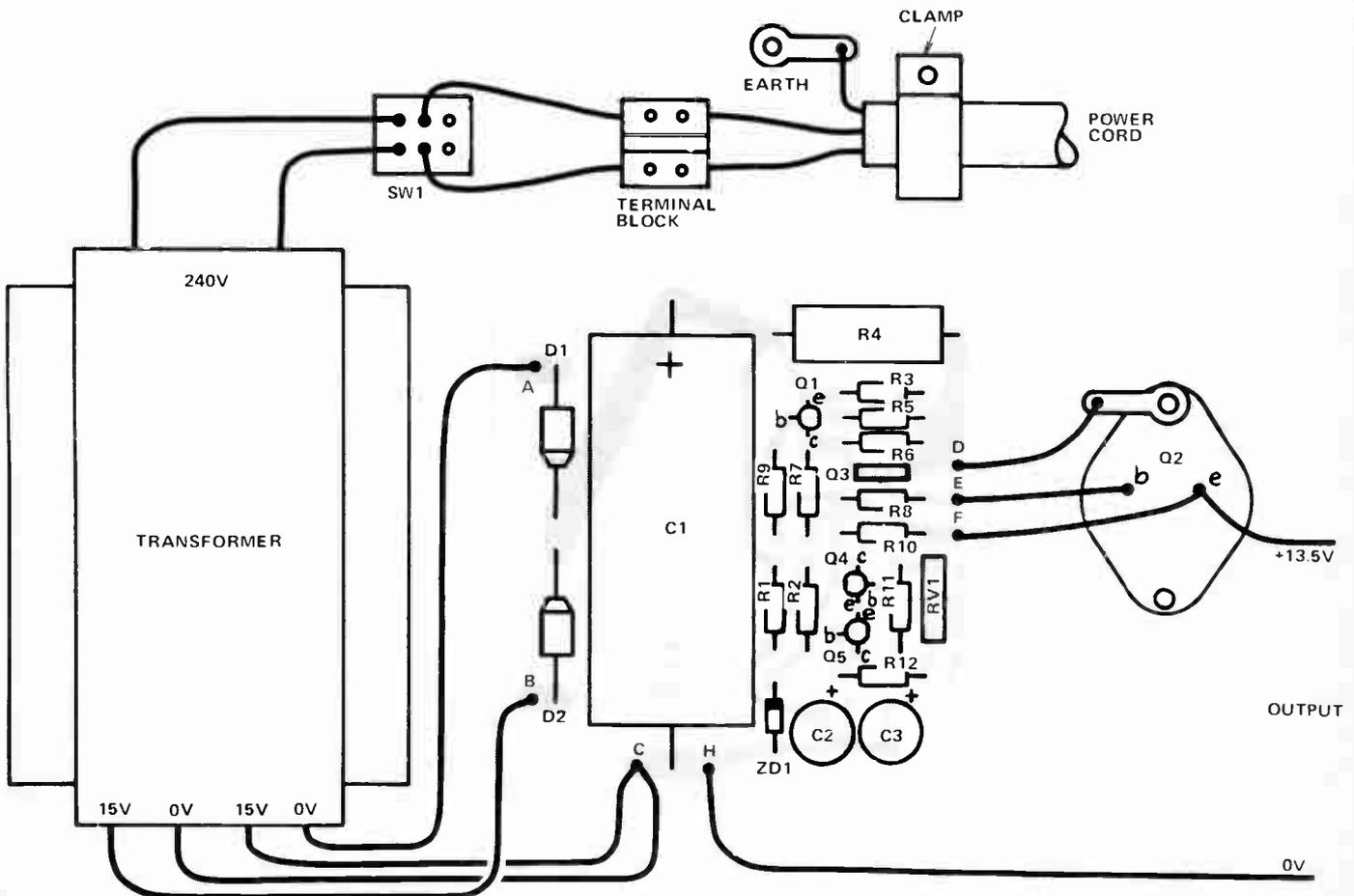
Fig. 3. Component overlay and wiring diagram.
