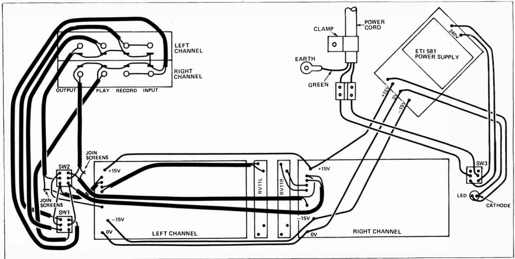
Fig. 6. Interconnection diagram for the unit.
