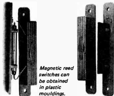
*Magnetic reed switches can be obtained in plastic mouldings.*
