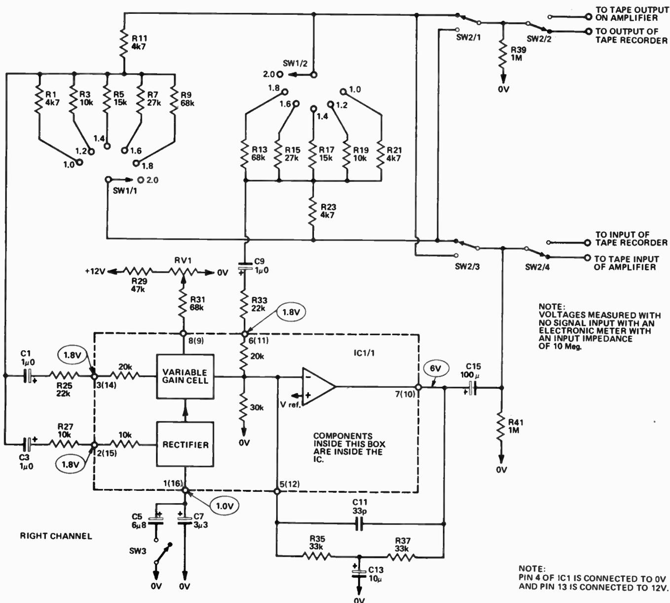
Fig. 1. Circuit diagram of the right channel.
