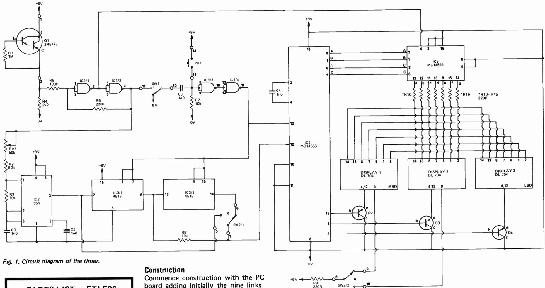
Fig. 1. Circuit diagram of the timer.
