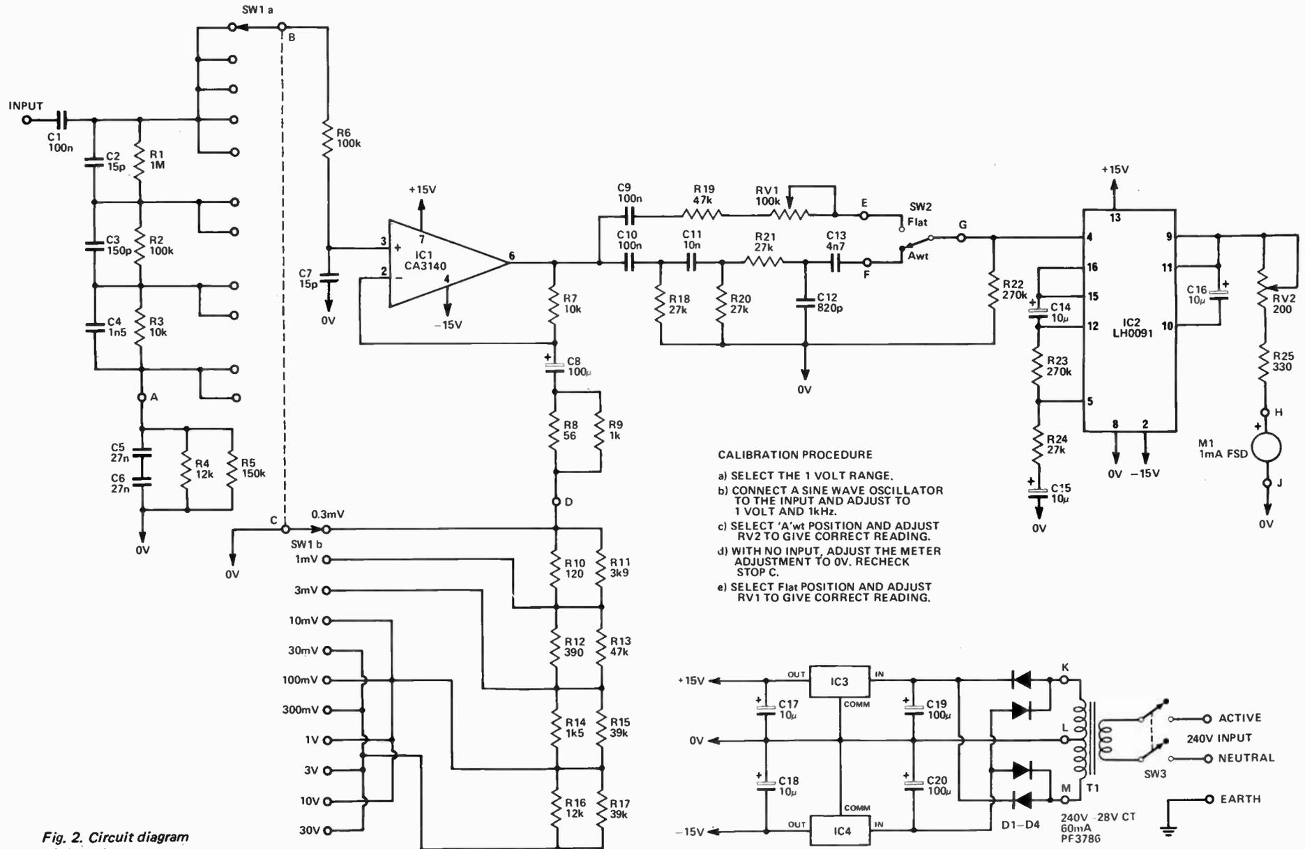
Fig. 2. Circuit diagram of the voltmeter.
