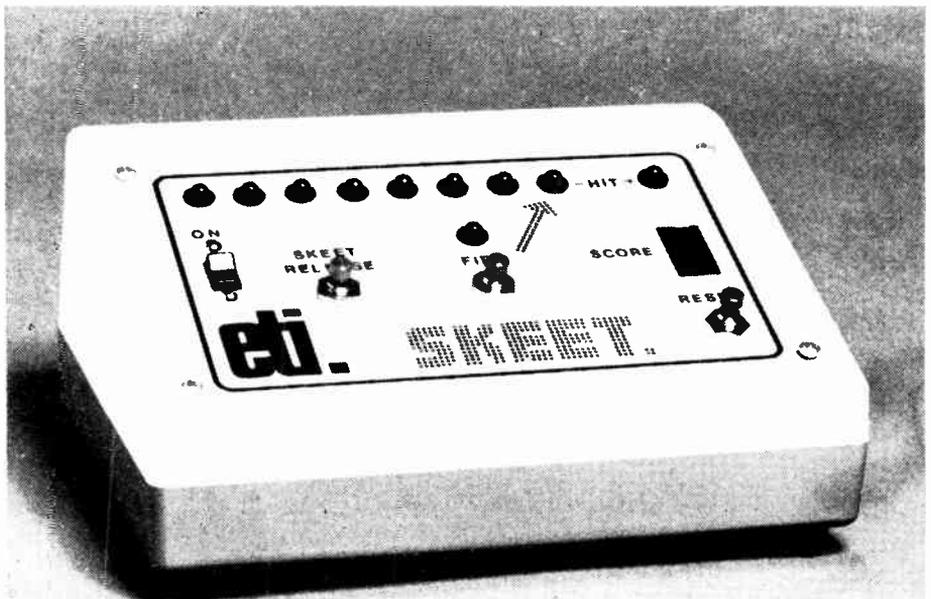
At the instant that the LED turns off, if the Skeet has just reached the end of its flight, a "hit" is registered and the "hit" LED lit.
