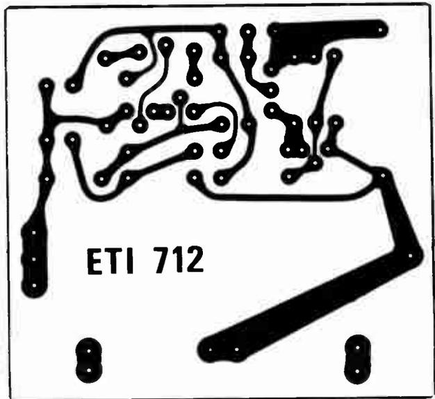
Fig. 2. Printed circuit layout. Full size 80 x 75 mm.
