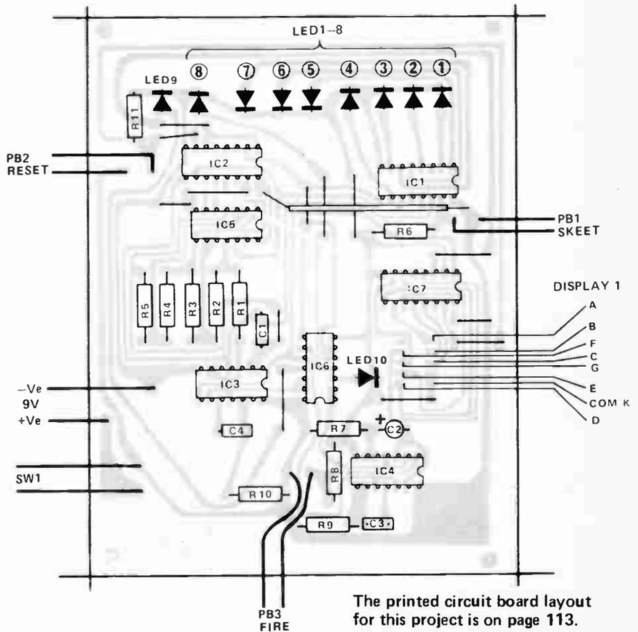
Right: the component overlay for the skeet game. All the links but for that between IC1 pin 16 and IC2 pin 16 may be made from uninsulated wire.
