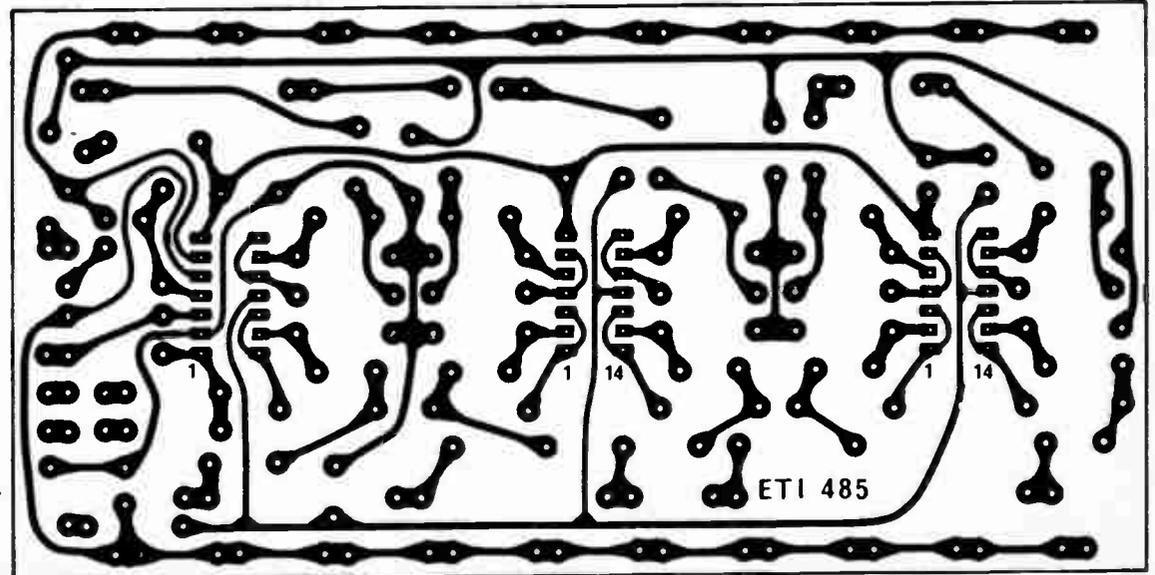
Fig. 2. Printed circuit layout. Full size 150 x 75 mm.
