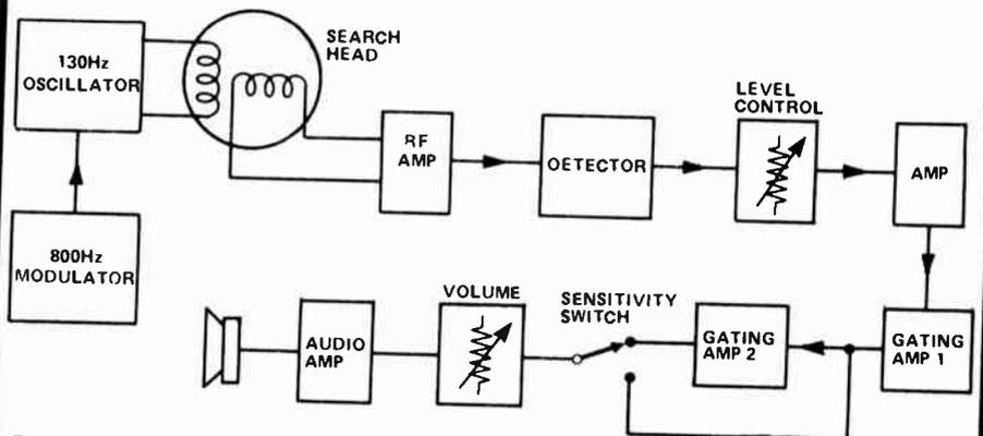
Fig. 2b. Block diagram of our IB design.
