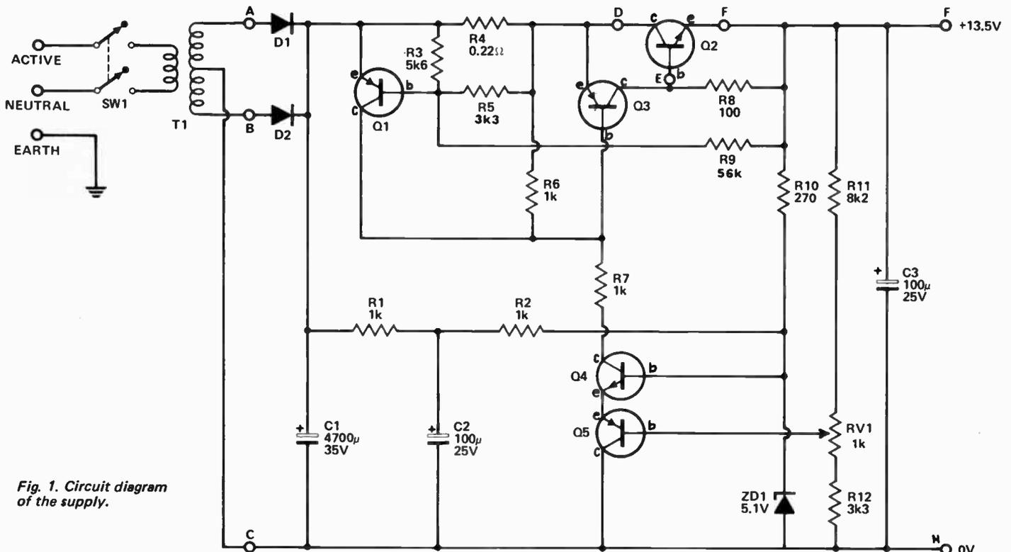
Fig. 1. Circuit diagram of the supply.
