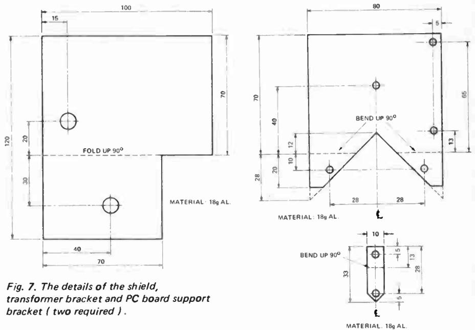
Fig. 7. The details of the shield, transformer bracket and PC board support bracket (two required).
