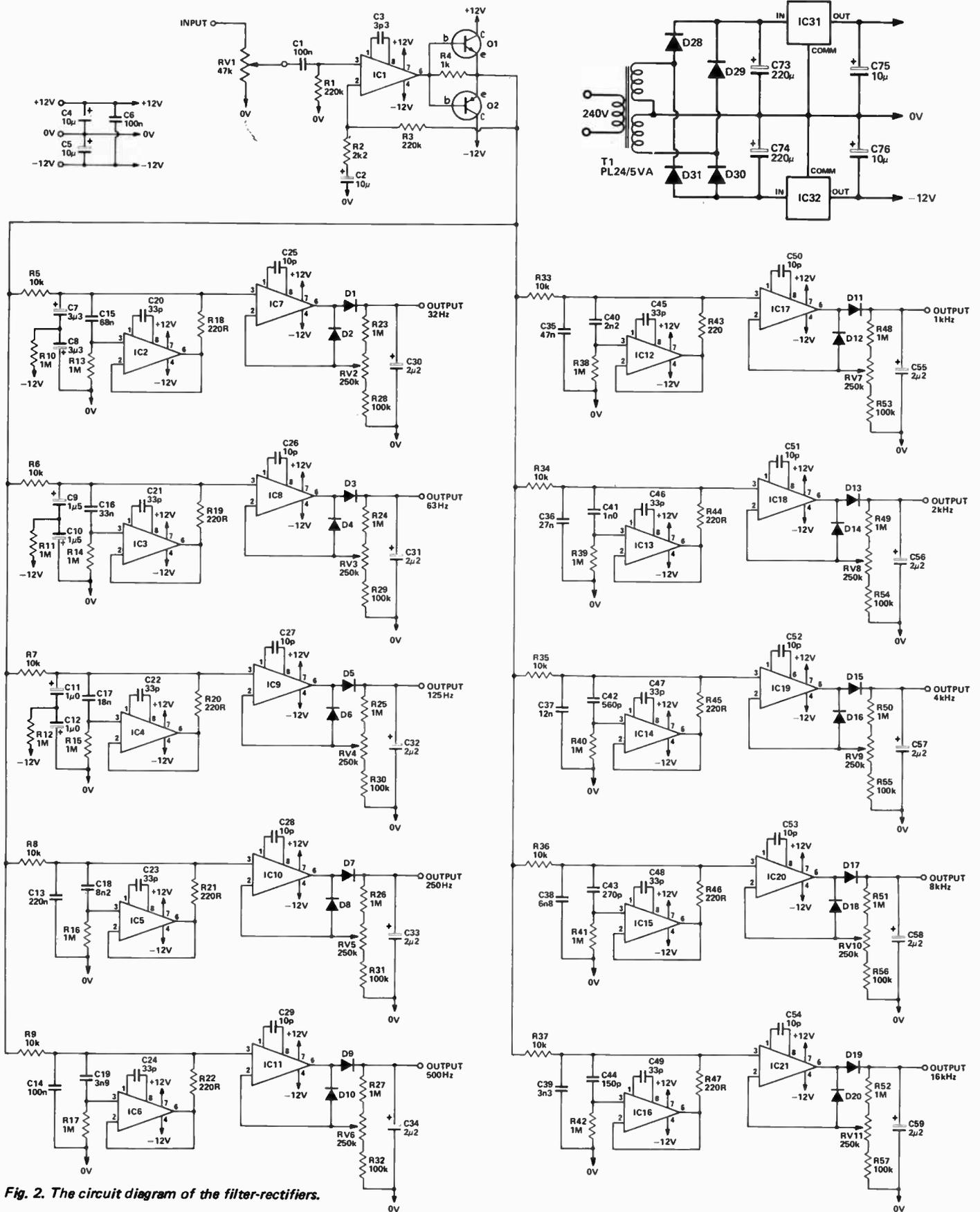
Fig. 2. The circuit diagram of the filter-rectifiers.
