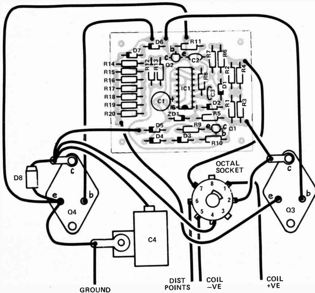
Fig. 2. Overlay and wiring diagram.
