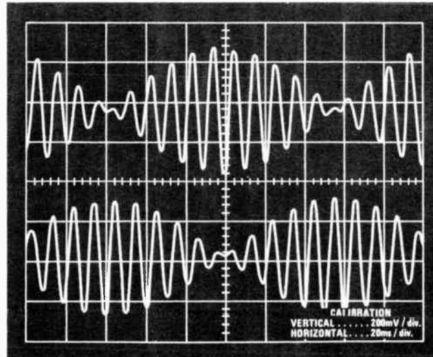
Fig. 2. The output of IC3 (top) and IC4 (lower) with a 100 Hz input signal. Note the phase difference.
