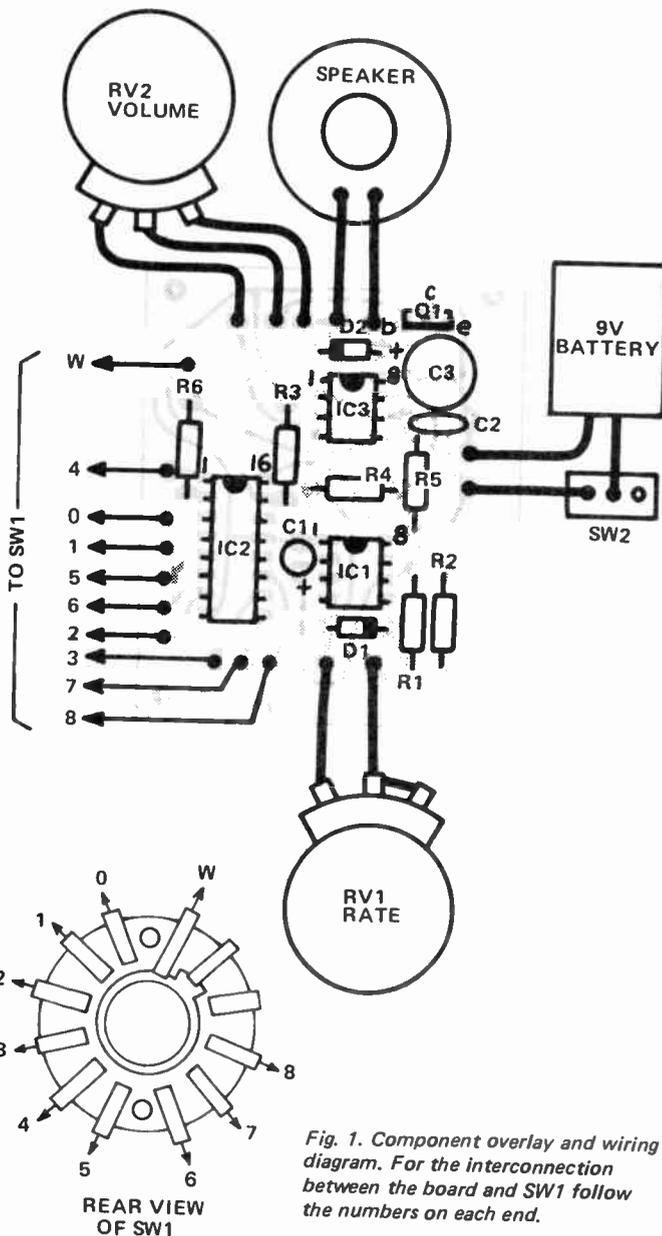
Fig. 1. Component overlay and wiring diagram. For the interconnection between the board and SW1 follow the numbers on each end.
