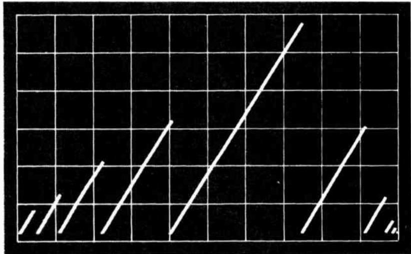
Fig. 7. The waveform on the Y output (vertical) with a 1 kHz tone input. See page 38 for the X-Y display. Note that the time between cycles varies with the height.
