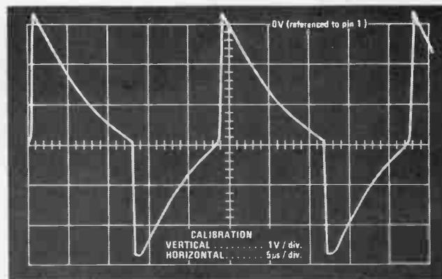
Fig. 9. The input of the oscillator — pin 40.
