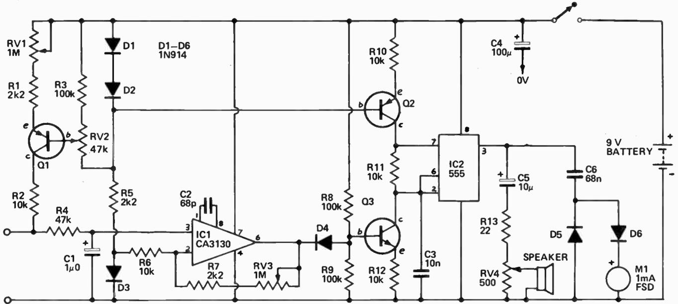
Fig. 1. Circuit diagram of the GSR monitor.
