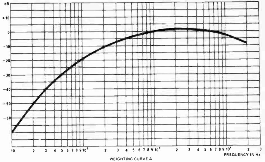
Fig. 6. The response in the "A" weight position.
