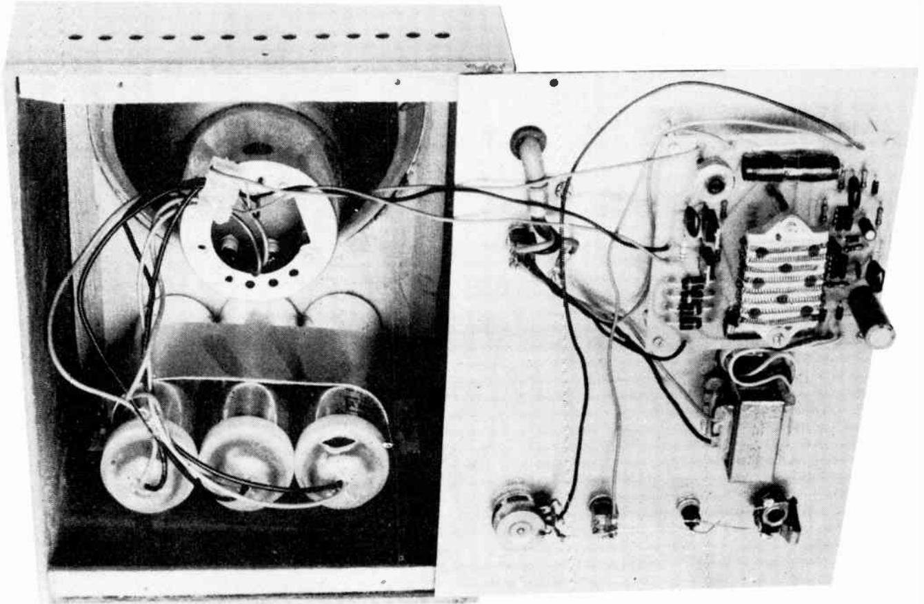
long metal spacers to allow for cooling. If you plan to run the strobe at more than 10 or 12 flashes per second a piece of asbestos about 100 mm square must be placed between the resistor and the pcb to prevent heat damage. Similar protection should be given to any burnable substances (the wooden box, if used) near the resistor.
