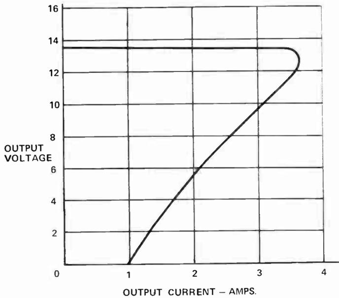
Graph showing relationship between output voltage and current. Note that the current into a short circuit is less than that available at 13 V.
