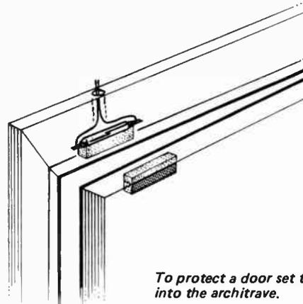
To protect a door set the reed switch into the architrave.
