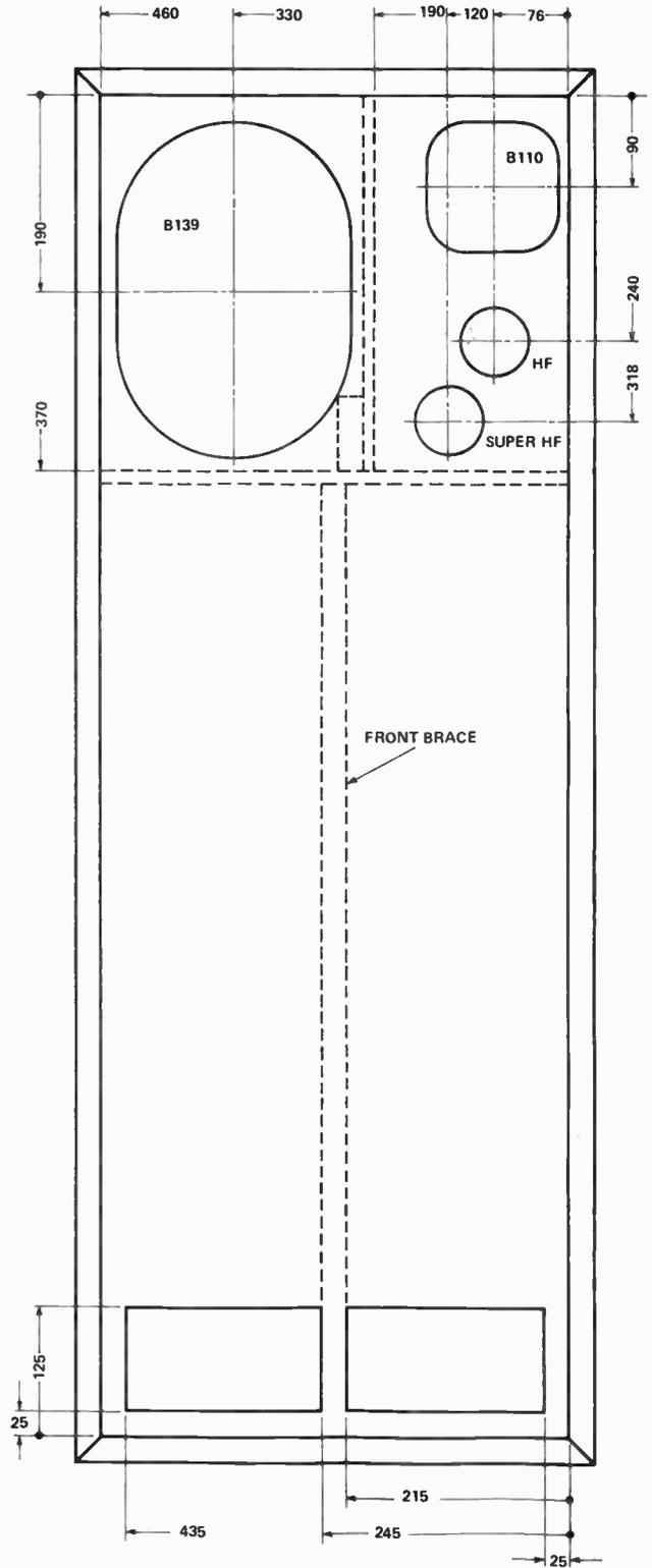
*Study these drawings in conjunction with the one on the following page. Note that ideally the speakers should be built as a 'mirror-image' pair – that is, so that when placed in the listening room the tweeters should be innermost.*
