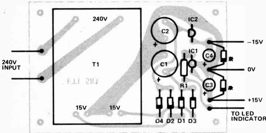
Fig. 3. Component overlay of the higher powered version.
