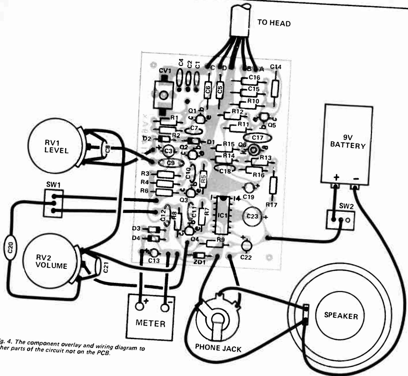
Fig. 4. The component overlay and wiring diagram to other parts of the circuit not on the PCB.
