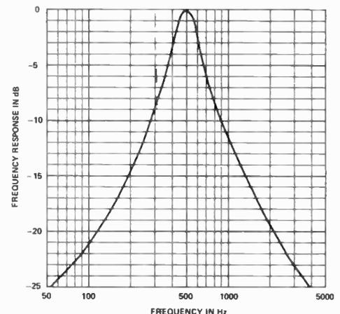
Fig. 1. The frequency response of the 500Hz filter. All other filters follow a similar curve.
