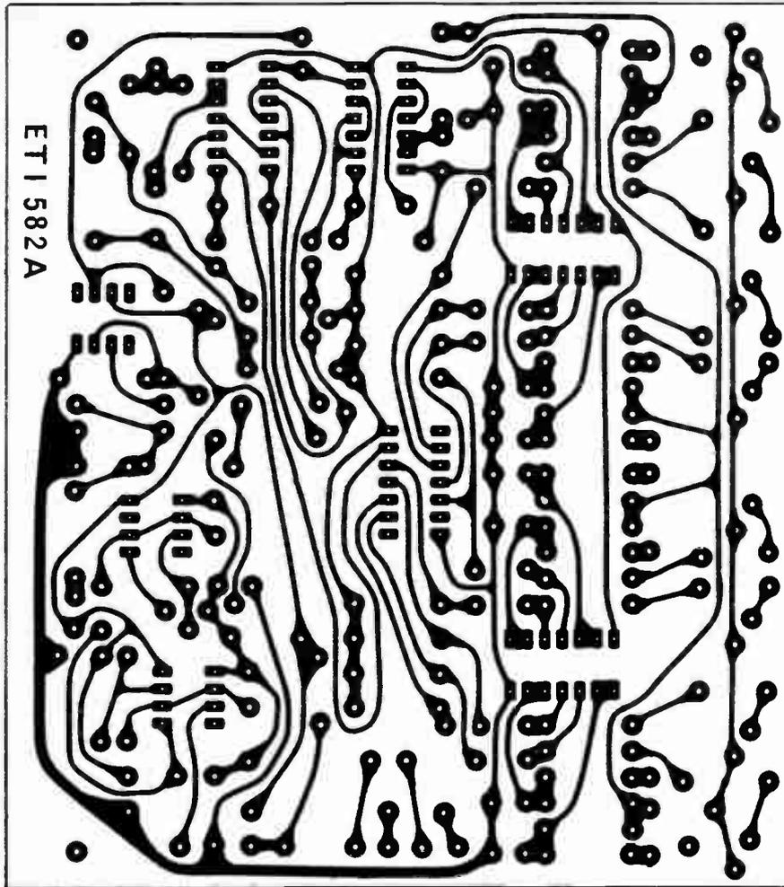
Fig. 7. PC board layout of board 'A'. Full size 130 x 115 mm.
