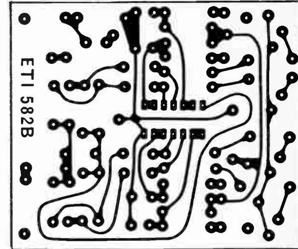
Fig. 6. PC board layout of board 'B'. Full size 75 x 65 mm.
