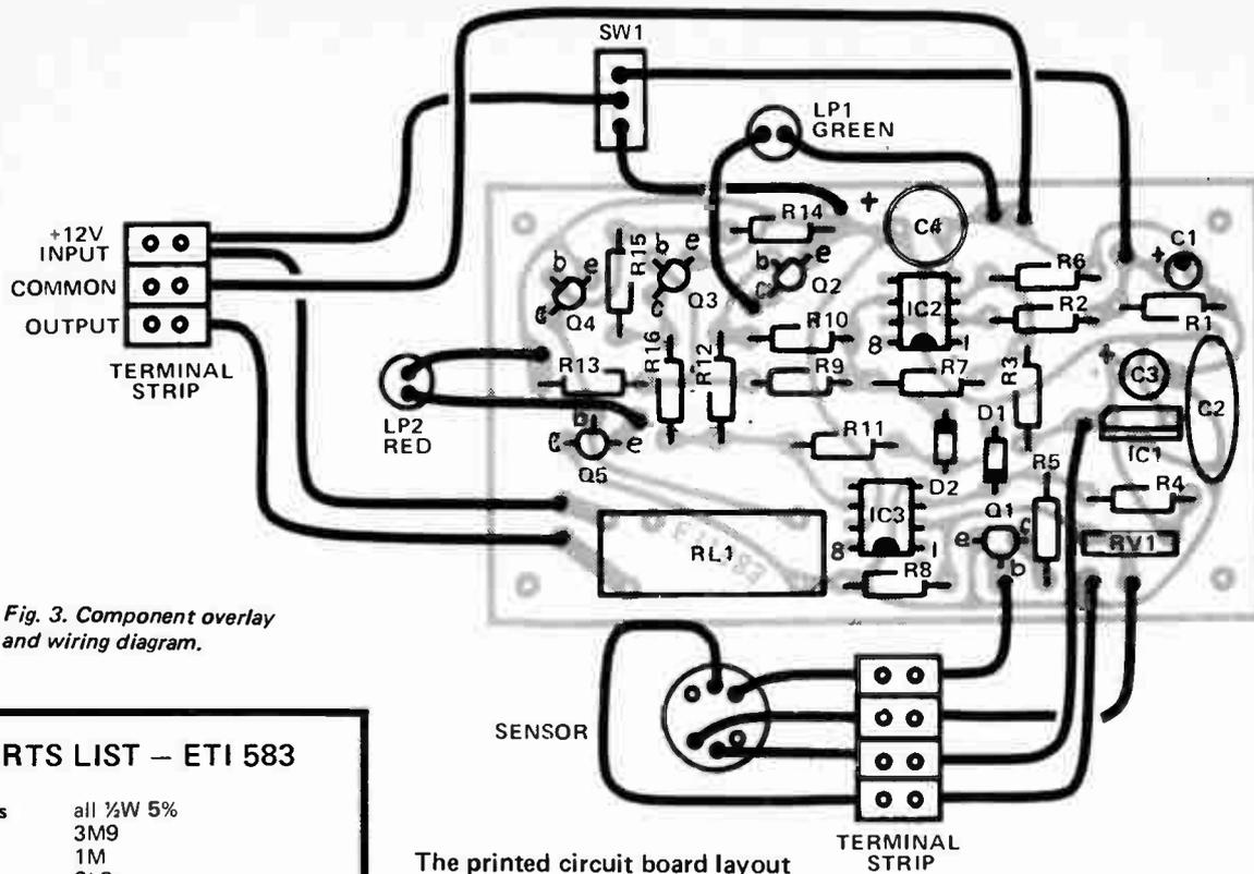
Fig. 3. Component overlay and wiring diagram.
