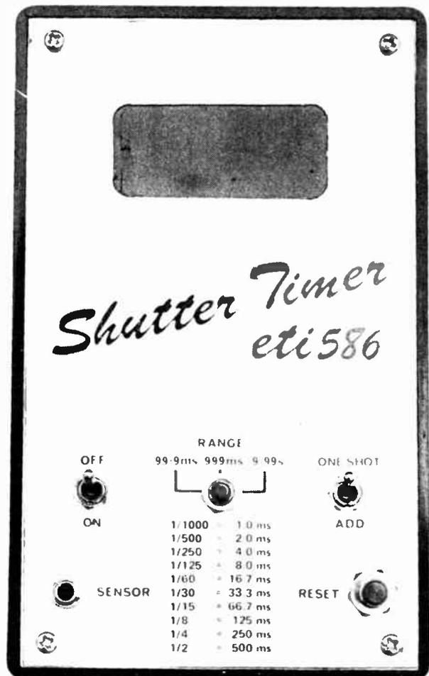
It is suitable for checking cameras with a hinged or removable back so that the sensor can be placed in the film plane. For cameras where the film fits into a slot this unit cannot be used.
