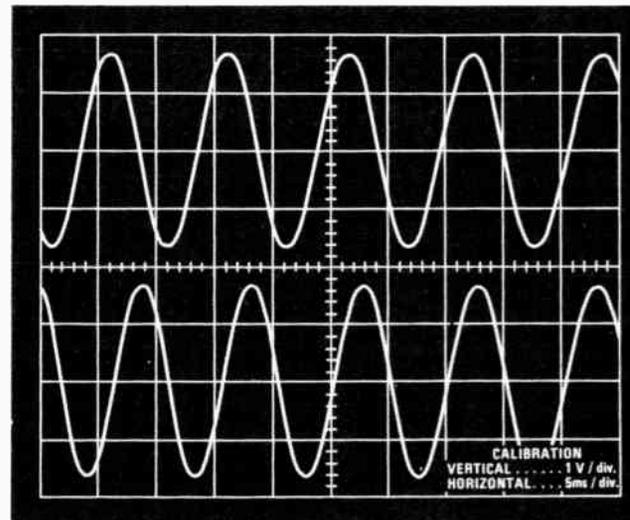
Fig. 3. The input signal (top) and the output (lower). Note the difference in frequency.
