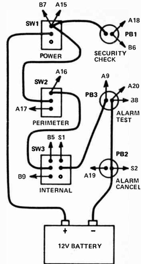
Fig. 3. Wiring of the switching and pushbuttons.
