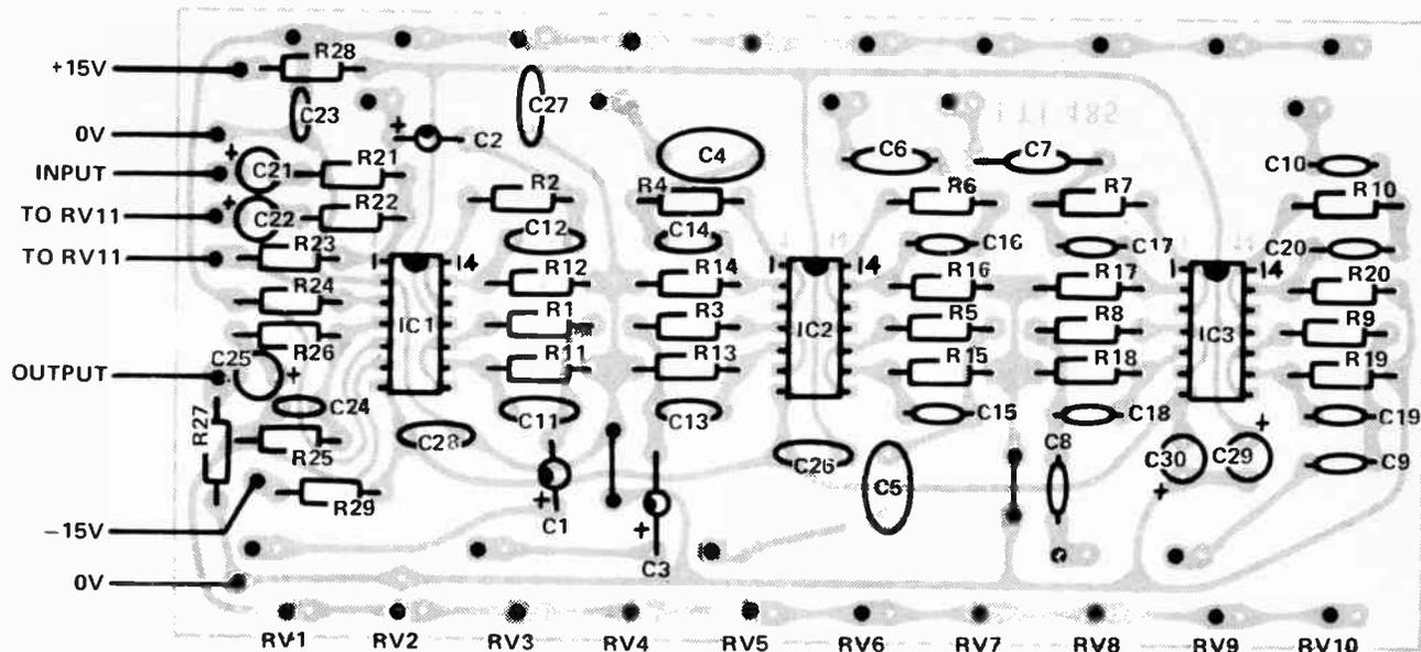
NOTE: RV1–RV10 ARE ON THE COPPER SIDE OF THE BOARD
