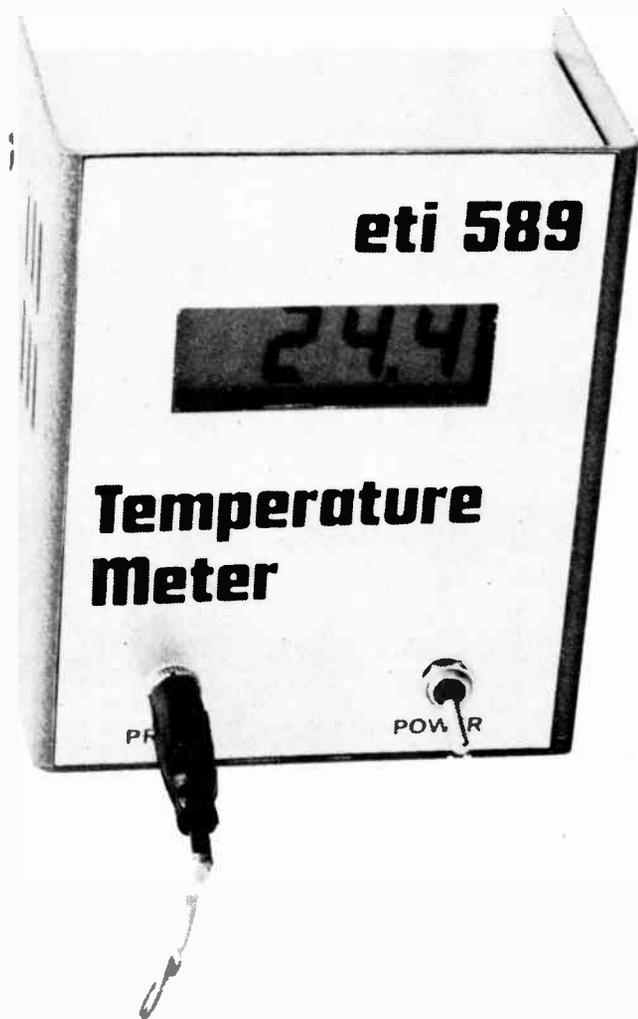
the diode. Silicon grease should be used to minimise the surface-to-surface temperature difference. Also when measuring small objects, e.g. a TO-18 transistor, the probe will actually cool the device slightly. At high temperatures these effects could give an error of up to 5% (the reading is always less than the true value). If the probe is in a fluid, e.g. water or air this problem does not occur.
