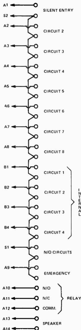
Fig. 5. Connection of the rear terminal blocks.
