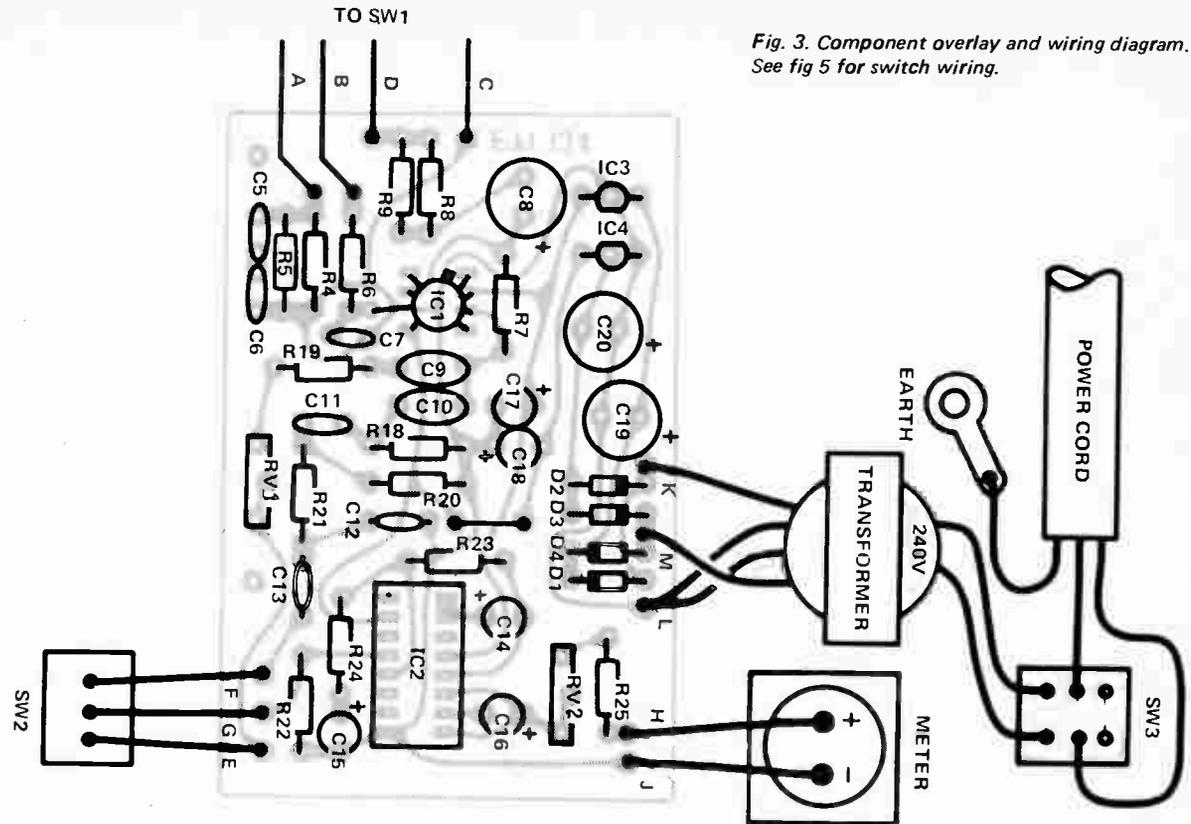
Fig. 3. Component overlay and wiring diagram. See fig 5 for switch wiring.
