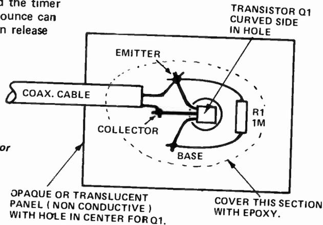
Fig. 3. Connection of the transistor on the sensor plate.
