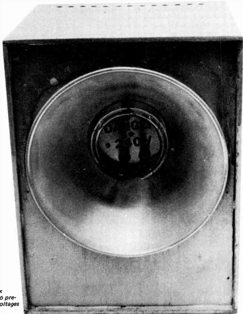
*The front of the strobe with the perspex cover removed. The cover is necessary to prevent accidental contact with the mains voltages applied to the flash tube.*
