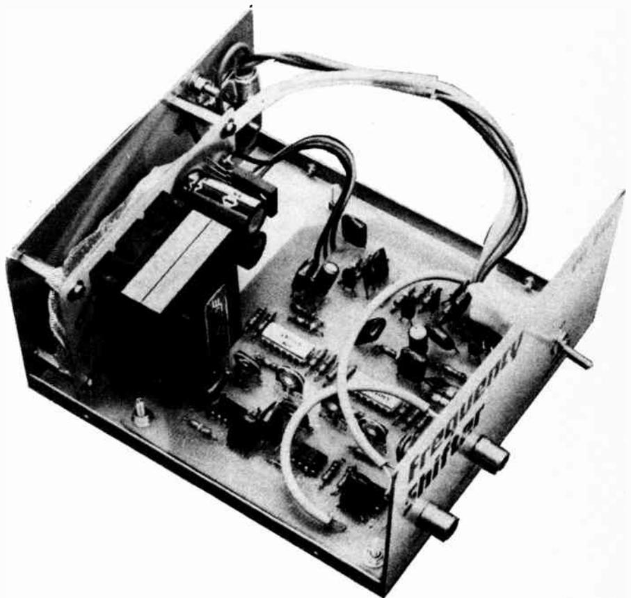
the output with a 1 – 2 V input signal and adjust RV6 to give the minimum amplitude modulation. Alternatively, by using an amplifier and speaker, RV5 can be adjusted by ear. The unit is now set up.
