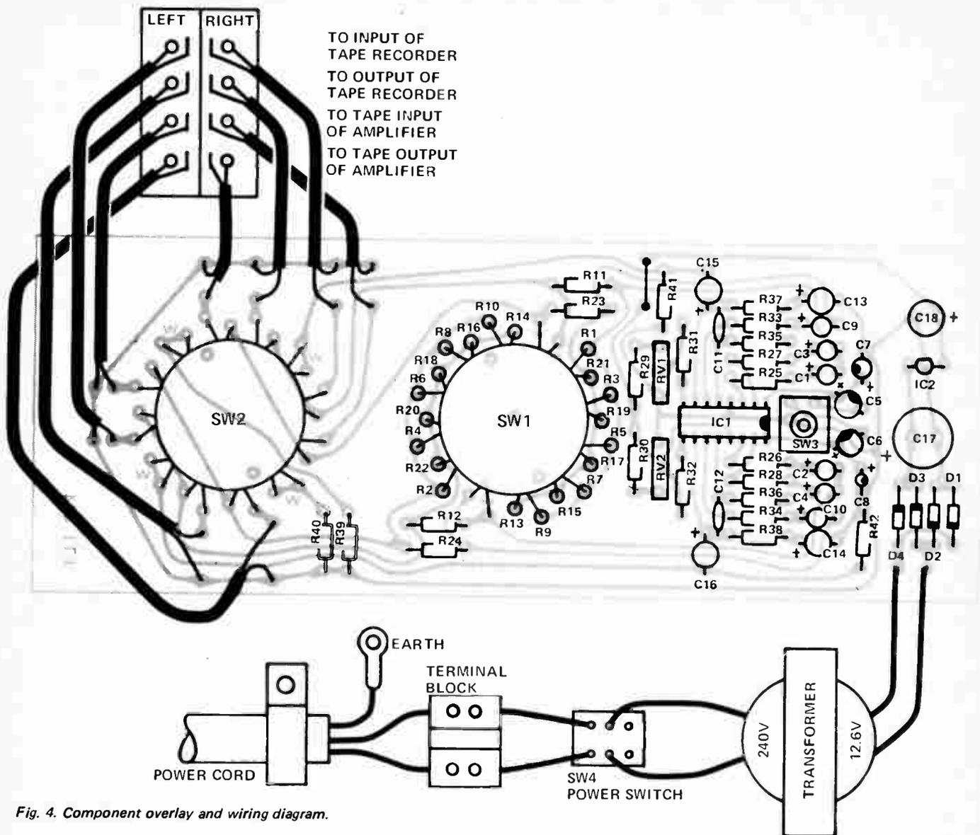
Fig. 4. Component overlay and wiring diagram.
