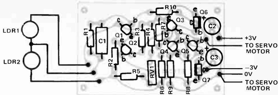
Fig. 2. Component overlay.
