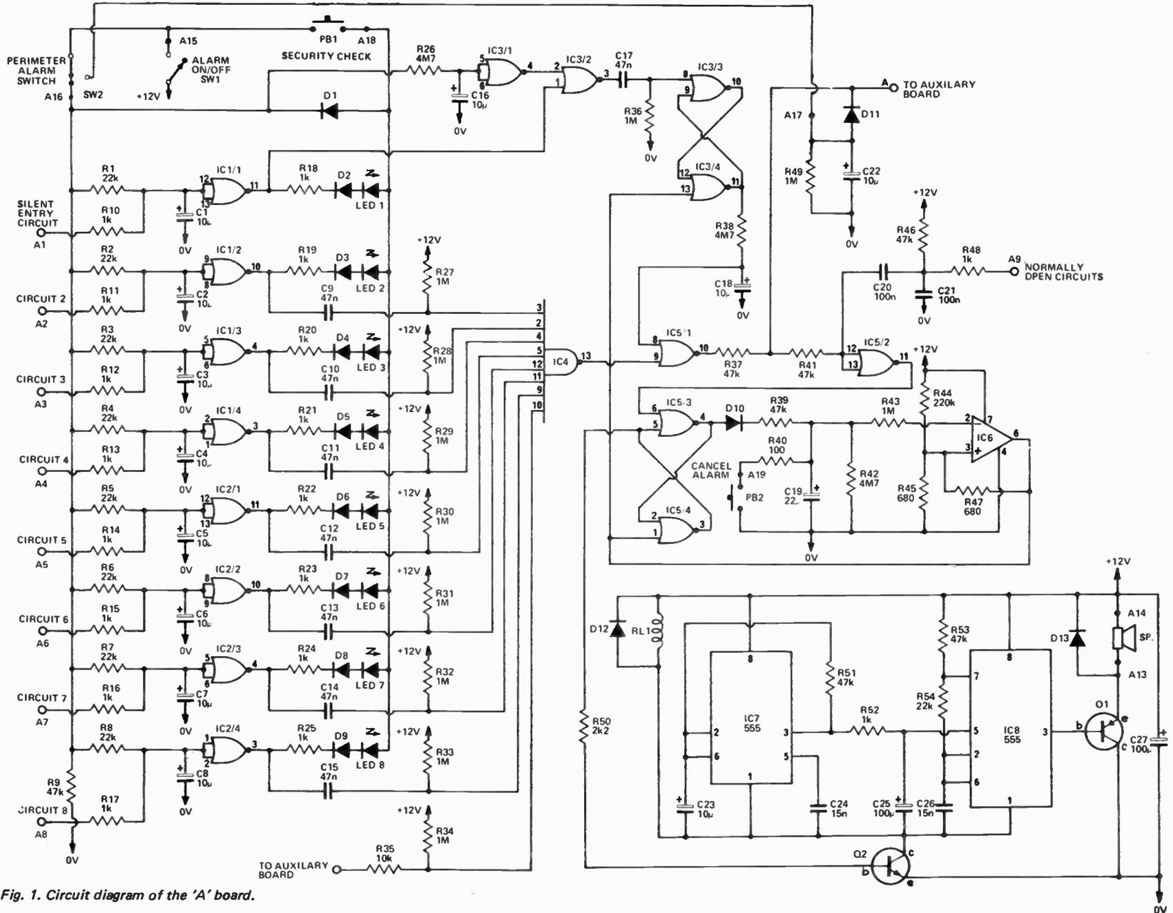
Fig. 1. Circuit diagram of the 'A' board.
