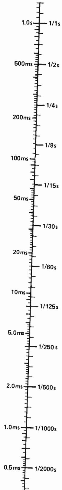
Fig. 4. Graph showing the relationship between time and shutter speed. Each of the small divisions on the right hand side corresponds with a 1/2 stop.
