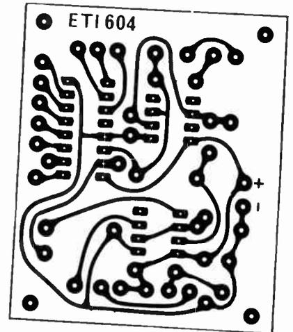
Fig. 4. Printed circuit layout.
