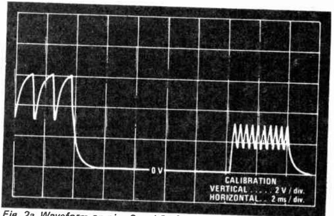
Fig. 2a. Waveform on pins 2 and 6 of IC3.
