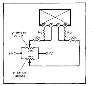
$(R_x \text{ and } R_y)$  for the x and y sections of the multiplier are in k $\Omega$ . Conversion gain of the multiplier is
