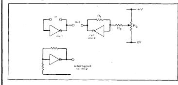
Typical performance IC CD4001AE NOR gates with 2 inputs active Supply +10VR<sub>1</sub> 27k $\Omega$ R<sub>2</sub> 1M $\Omega$ R<sub>3</sub> 100k $\Omega$
