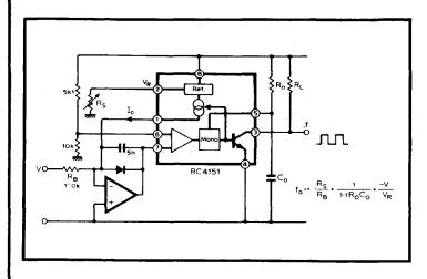
The new generation of linear integrated circuits includes complete v-f modules that will compete with the hybrid and modular versions for many applications. One such monolithic device RC4151 is in line of succession to the 555. It includes a monostable comparator and output stage, but adds a switched current generator. It can be used without additional active devices, but for improved linearity is combined with an op-amp to form a chargebalancing system. The input
