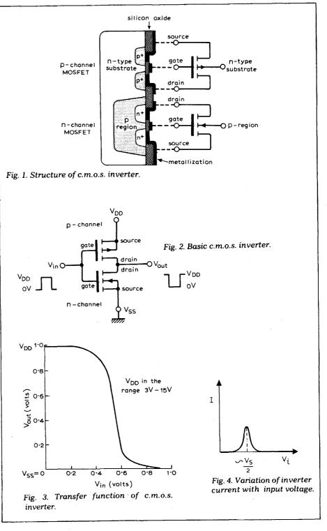
logic level inverter, but the transient current pulse as shown in Fig. 4 is then the only significant contribution to current drain, as one or other of the transistors is non-conducting in each of the logic states. (At high pulse rates power consumption is associated with the multiple charge/discharge of internal and load capacitances.)
