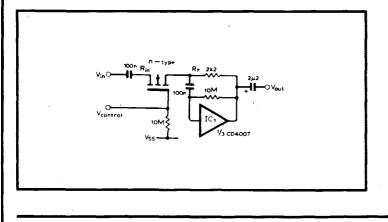
This voltage controlled amplifier is derived from a CD4007 package. IC<sub>1</sub> inverter is biased into its linear region by the 10M $\Omega$ resistor, and one of the n-type f.e.t. is used as a voltage variable resistor. Control voltage range is dependent on  $|V_{DD} - V_{SS}|$ . With above network gain is claimed variable from zero to just over unity.
