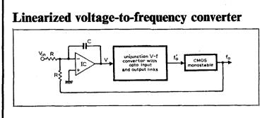
Components R 100k $\Omega$ , C 0.22 $\mu$ F IC 741 Unijunction V-f'\_o-see over, centre. Monostable-see over, right V<sub>in</sub> 0 $\rightarrow$ -10V
