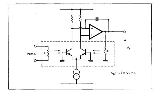
heat to each is equal. Any unbalance is amplified by the operational amplifier forcing the direct output voltage to deliver the same power to the righthand resistor as the input delivers to the other. Hence the r.m.s. values of the two voltages are equal. A neat idea, though one that requires a very carefully constructed chip if the sensing transistors are each to respond to only one of the heat sources.
