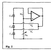
progressively less attenuated. When oscillations are vigorous, and distortion ensues, these harmonics are fed back introducing intermodulation distortion and shifting the frequency of oscillation away from the 180° phase-shift frequency of the network.
