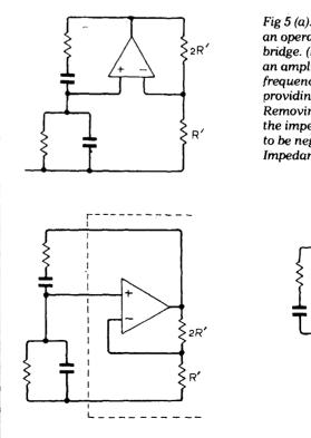
Fig 5 (a). A standard configuration uses an operational amplifier to activate the bridge. (b) Circuit partitioned to show an amplifier of gain +3 with the frequency-dependent network providing positive feedback. (c) Removing one section of the network, the impedance across the port is found to be negative, leading to Negative Impedance Converter interpretations.
