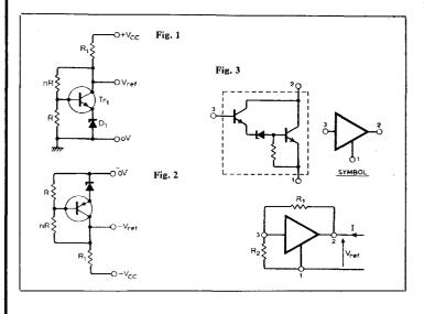
**Typical performance** + $V_{ce}$  +15V  $R_1$  4.7k $\Omega \pm 5\%$ ,  $R_2$  10k $\Omega$ multiturn  $\pm 1\%$ , linearity  $\pm 0.1\%$ Tr<sub>1</sub> BC125 Currents for n=1 condition I<sub>1</sub> 2.91mA, I<sub>C</sub> 2.77mA I<sub>2</sub> 144.6 $\mu$ A, I<sub>B</sub> 16 $\mu$ A (see graph opposite) Voltages for n=1 condition V<sub>BE</sub> 644mV, V<sub>REF</sub> 1.371V (see graph opposite)
