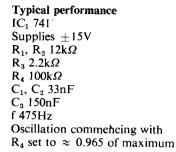
that. Re-drawing in op-amp form then leaves the gain sign to be deduced. Again the loop gain is greater than is needed to sustain oscillation, and the feedback is attenuated to produce minimum distortion. The same constraints on impedance levels apply, and the performance is very similar to the original.
