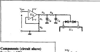
Supply  $\pm 10V$ IC<sub>1</sub> SH74S124N IC<sub>2</sub> LM301 R<sub>1</sub> R<sub>2</sub> 10k $\Omega$ R<sub>3</sub> R<sub>4</sub> 100k $\Omega$ C<sub>2</sub> C<sub>3</sub> 1 $\mu$ F C<sub>4</sub> C<sub>5</sub> MV16408
