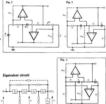
produce sustained oscillation. For  $Z_1 = Z_2 = Z_3 = Z_5 = R$  and  $Z_2 = 1/j\omega C$ ,  $Z_1 = j\omega C R^2$ .
