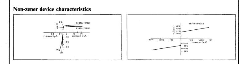
1. Asymmetric voltage dependent resistors—low voltage Non-linear resistors are made of certain polycrystalline materials having a voltagecurrent relationship given by  $V=CI^{\beta}$
