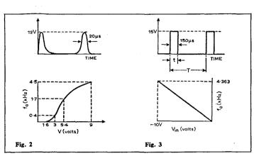
forward path changes, causing changes in  $f_0$ , will be completely cancelled, apart from transient effects. Changes in the shape of  $f_0$ , e.g. impulse height and width, will however have an effect on  $f_0$ , although not linearity.
