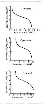
(no. 11) must be grounded for continuous output at the output terminal. Output is disabled if this terminal is taken to logic high or open-circuited. Graphs opposite indicate linearity over a restricted range for each capacitor value, and waveform deteriorates at very low values of  $C_1$ , and thus at high frequencies.
