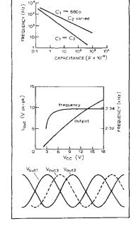
t.h.d. 1.2%. For 470k $\Omega$ , V<sub>out</sub> 4.4V pk-pk, t.h.d. 0.3%. R<sub>2</sub> 7.8M $\Omega$  V<sub>out</sub> 6.8V pk-pk, t.h.d. 0.6%. For 4.7M $\Omega$ , V<sub>out</sub> 4:1V pk-pk, t.h.d. 0.2%. For all above alterations, frequency does not change more than 0.2%. Variation with supply C<sub>1</sub>, C<sub>2</sub> shown on graphs.
