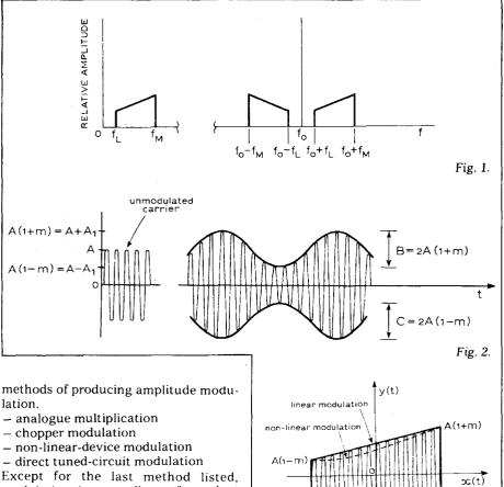
Except for the last method listed, modulation is normally performed at low power levels and the required output power obtained by class-B amplification of the modulated signal.
