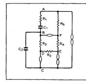
since  $f \propto 1/\sqrt{R_3}$ . Typically R<sub>3</sub> may range from 100 $\Omega$  to  $>1M\Omega$ .
