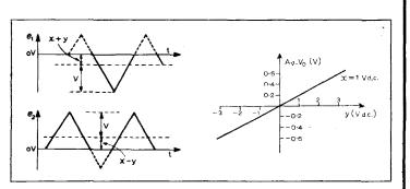
inverted sum of  $e_1$ ,  $e_2$  and y. With x and y both at 1V and varying the frequency of the triangular wave the output accuracy was maintained within 1% up to 6kHz. The device is a 4-quadrant multiplier.
