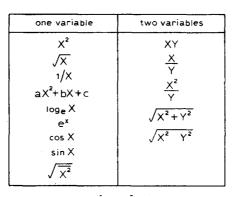
Fig. 1. Common functions that can be obtained by passing X, Y through circuits with corresponding transfer functions.
