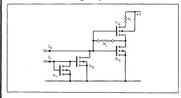
Typical performance IC CD4007 ( $Tr_{1-4}$ ) Supply +15V  $R_1 100k\Omega$   $R_L 1k\Omega$   $I_1, I_2 100\mu A$   $I_L \pm 1\mu A$   $I_L = I_1 - I_2$ Output resistance > 100M $\Omega$ at  $I_L = 10\mu A$ Max.  $R_L \approx 0.5M\Omega$ at  $I_L = 10\mu A$  for good linearity
