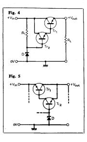
value. The current in the zener diode can be made much larger than the base current of  $Tr_1$  by choice of  $R_1$  and this current, hence  $V_Z$  and  $V_{OUT}$ , will be subject to variation as  $V_{IN}$ changes. The circuit is inherently safe with opencircuit loads but  $Tr_1$  must be chosen to dissipate the maximum power generated under  $V_{IN(max)}$  and  $R_{L(min)}$ conditions.
