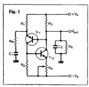
appropriate phase angle to the make the loop phase shift zero. The Fig. 1 circuit is of similar form to Fig. 2 for which an approximate analysis is given. Assume the base-emitter voltages are negligible. Then the signal v<sub>in</sub> will appear as v<sub>out</sub>. The input signal current i<sub>in</sub> comprises  $v_{in}/R_1$  and  $i_{in} - v_{in}/R_1$  up through Tr<sub>1</sub>. The voltage across R<sub>1</sub> is then  $i_{in}R_1 - v_{in}$  which must be that
