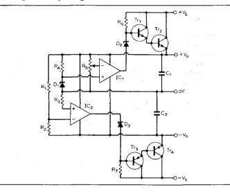
**Typical performance** IC<sub>1-2</sub> 741 Tr<sub>1</sub> BFR41, Tr<sub>2</sub> 2N3055 Tr<sub>3</sub> BFR81, Tr<sub>4</sub> 2N2955  $D_{1-3}$  6.8V zener diodes
