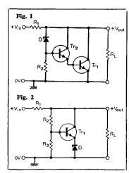
$D_1$  cathode and  $V_{OUT}$ . Note that  $V_{OUT}$  is now adjustable over a wide range, for a given zener voltage by choice of the ratio  $R_2$ :  $R_3$ .
