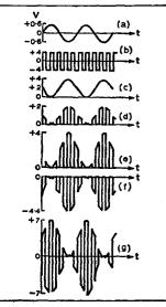
$R_8$  and  $R_{12}$ . The junctions of these pairs of resistors are connected to ground through  $Tr_1$  and  $Tr_2$  when these "chopper" transistors are switched on by the square-wave carrier ( $v_{1n_1}$ ).
