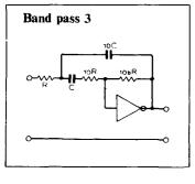
Typical performance IC  $\frac{1}{4} \times CD4001$ (quad NOR gates) Supply +10V C<sub>1</sub> 100pF C<sub>2</sub> 10nF R<sub>1</sub> R<sub>2</sub>, 100k $\Omega$ f<sub>0</sub> 1490Hz Q 2.5 (For an ideal inverter, C<sub>2</sub>/C<sub>1</sub>=4Q<sup>2</sup> but with the very limited gain the theoretical Q of 5 is reduced to 2.5, see Ref. 1.)
