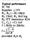
but the need for a twin-gang control which normally requires a good match is avoided. A further advantage of this circuit is that low frequencies are obtained without using large values of capacitance. Provided the thermistor has a long enough thermal time constant, frequencies down to 10Hz are possible with capacitances of 0.1µF.
