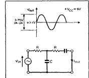
In the above circuit, for example, where R was selected oscillations the amplifier must provide a current-to-voltage gain ( $A_z$ ) of 3R ohms to make the closed-loop gain unity i.e.  $\beta_y.A_z = 1$ .
