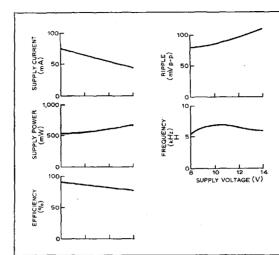
voltages the latter limits the efficiency—between 70 and 90% is common even where the output voltage is  $\langle V_S/2 \rangle$ . As the supply voltage varies the mean current changes in the opposite sense because the mark-space ratio is adjusted automatically via the astable action. Hence the mean power drawn from the supply depends mainly on the power required by the load.
