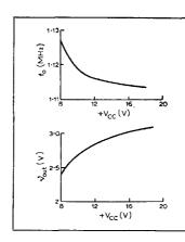
output waveform. The more the gain exceeds the critical value the more distorted will the output waveform become and the lower will be the frequency of oscillation. (See graphs for effect of increasing supply voltage, for example, after setting the critical condition at a lower value of +Vcc.)
