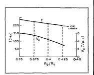
open-circuit voltage gain falls; at low voltages the output impedance becomes too high. Best range 5 to 10V.  $R_1$ : Circuit requires relatively high resistance values to reduce loading on output—typically 10k to 10M $\Omega$ .  $R_2$ :  $R_1/2$
