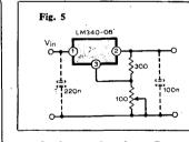
on the internal resistor  $R_1$ . LM109/309 are earlier versions on the same principle, but designed specifically for +5Vlogic levels. Fig. 5 is an adjustable output circuit. Capacitors are optional depending on transient response requirement and distance from supply. Another advantage of this i.c. is the internal circuitry which provides shutdown of the regulator if the die temperature reaches 175°C, thus providing virtually absolute protection.
