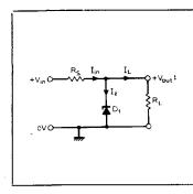
Typical performance  $I_{Lconstant}$ ,  $V_{IN}$  variable  $D_1$  BZY96C9V,  $I_L$  50mA  $V_{IN(min)}$  12V,  $V_{IN(max)}$  18V  $R_S$  54 $\Omega$  (39 $\Omega$ +15 $\Omega$ )  $R_L$  195 $\Omega$  (3×56 $\Omega$ +27 $\Omega$ ) to set  $I_L$  at 50mA
