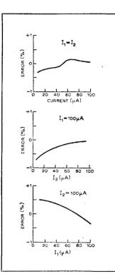
**Typical data**   $Tr_1$ - $Tr_3$  3/5 of CA3086  $Tr_4$ - $Tr_7$  4/5 of CA3086  $V_8 \pm 5V R_1$  33k $\Omega$ For graphs, currents  $I_1$  and  $I_2$ are derived from calibrated current sources.  $I_0 = \sqrt{I_1^2 + I_2^2}$ . Percentage error shown in graphs.
