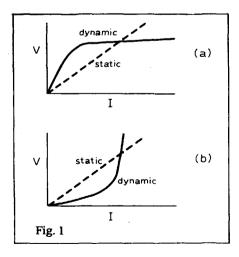
Zener breakdown is a field effect which dominates for heavily-doped narrow junctions, where even small p.ds of three or four volts can provide a sufficiently intense field for the direct production of hole-electron pairs. The observed characteristics are that the current increases steadily as the operating region is approached, with a rounded knee, and with a temperature drift of about  $-2mVK^{-1}$ . To a first order the slope resistance of such diodes is inverse to the quiescent current.
