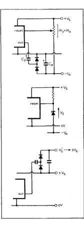
Typical performance IC<sub>1</sub> 555 timer D<sub>1-7</sub> 1N4148 C<sub>2-5</sub>  $47\mu$ F, C<sub>1</sub> 0.015 $\mu$ F R<sub>1</sub> 1.2k $\Omega$ , R<sub>2</sub> 10k $\Omega$ , R<sub>3,4</sub> 22k $\Omega$ +V<sub>8</sub> +10V V<sub>0</sub> -10V I<sub>0</sub> 0 to -20mA  $V_0/V_8 \pm 0.5\%$  for V<sub>8</sub> 7 to 14V
