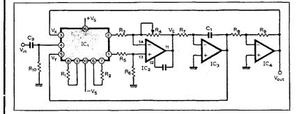
Typical data IC<sub>1</sub> XR2308 V<sub>8</sub>  $\pm 10V$ IC<sub>2</sub> (included in IC<sub>1</sub>) IC<sub>3</sub>, IC<sub>4</sub> SN741, R<sub>10</sub>, R<sub>7</sub> 47k $\Omega$ R<sub>1</sub>, R<sub>2</sub>22k $\Omega$ , R<sub>8</sub>, R<sub>9</sub>10k $\Omega \pm 0.1\%$ R<sub>3</sub>, R<sub>5</sub> 56k $\Omega$ , R<sub>6</sub> 100k $\Omega$ R<sub>4</sub> 100k $\Omega$  potentiometer V<sub>in</sub> 1-5V r.m.s. C<sub>1</sub>, C<sub>2</sub> 1 $\mu$ F frequency 1kHz V<sub>out</sub>1-5V d.c.
