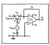
**Typical data** IC<sub>1</sub> 741, Tr<sub>1</sub> 2N5457 Supply  $\pm 15V$ R<sub>1</sub> 10k $\Omega$   $\nu_{mod}$  1V pk-pk  $f_{mod}$  1kHz  $\nu_{carrier}$  100mV pk-pk  $f_{carrier}$  10kHz  $\nu_{B} \approx 0.75V$ Output at  $\nu_{0}$  as shown top. D.C. transfer function between input carrier and  $\nu_{0}$ , for varying  $V_{GS}$  of f.e.t., provides information on linear regions.
