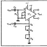
$v_{out}$  (pin 1 or 7) 800mV pk-pk unmodulated, see waveform opposite. Balanced modulator Vg 2.5V d.c. to balance out carrier  $v_{in1}$  (carrier) 130mV pk-pk  $f_c$  1MHz  $v_{in2}$  (modulation) 2.4V pk-pk (max)  $f_m$  10kHz  $v_{out}$  (pin 1 or 7) see waveform opposite.
