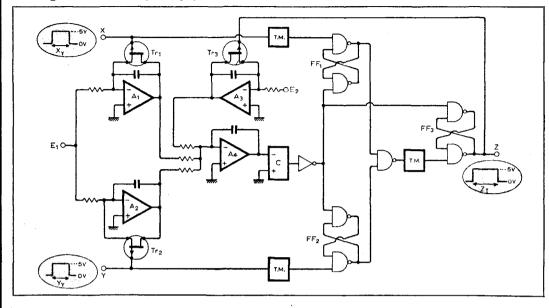
Analogue information x and y is contained in the input pulse widths  $x_T$  and  $y_T$  respectively.
