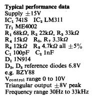
Vary mark/space ratio of output at  $V_{02}$  by  $R_2/R_1$  ratio change; this also modifies frequency. Range of  $R_2$ ,  $R_1$  22 to  $68k\Omega$ Range of mark/space 1:1 to 1:3.
