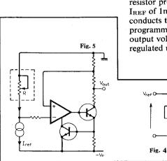
resistor provides a current  $I_{REF}$  of 1mA. When this conducts through an external programming resistor R, the output voltage available is regulated up to zero volts.
