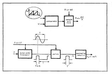
input voltage. This produces a ramp output voltage which has to be reduced to zero every  $2\pi$  radians. This can be done by inserting a f.e.t. in parallel with the feedback capacitor and triggering the f.e.t. from a monostable fed from  $R\sin \omega t$  via a comparator.
