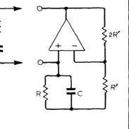
passive network in some way, and in addition there is an effective loss in Q of the system that results in increased distortion. One example out of many that have been designed is shown in Fig. 6. Frequency ranges of up to three decades have been reported, while the amplitude control mechanisms are similar to those above.
