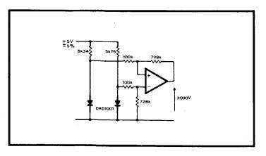
One special device that has been reported, contains a pair of silicon p-n junctions. One is so heavily doped that its band-gap voltage is reduced to that of germanium. The voltage difference is then temperature stable at around 0.41V, the difference between silicon and germanium band-gap voltages. The configuration of the circuit is not particularly novel, but the temperature coefficient is < 10p.p.m.  $K^{-1}$ , over the full military temperature range.
