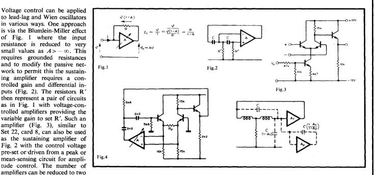
effect can be applied to LC oscillators to replace a capacitor that normally appears in a feedback path by either a grounded capacitor or one connected across a separate amplifier. If  $A_1$  is fixed to sustain oscillations, then  $A_2$  varies the effective
