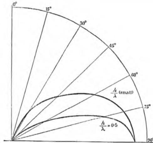
FIG. 5.—Vertical polar diagram of radiation for  $\frac{1}{2}\lambda$  and  $\frac{1}{4}\lambda$  (or less) aerials. Drawn for the same maximum radiation intensity in the horizontal plane.
