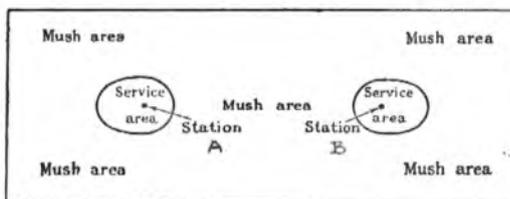
FIG. 13.—Showing small service area and large 'mush' area (where quality of transmission is bad) around two stations sharing the same wavelength.
