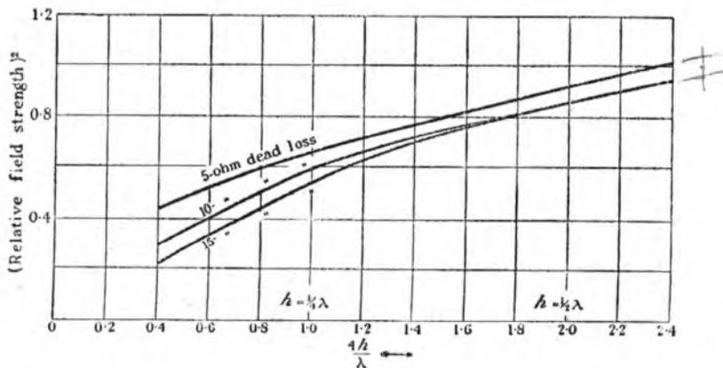
FIG. 10.—Relative field strength for a given power for various values of  $h/\lambda$ .
