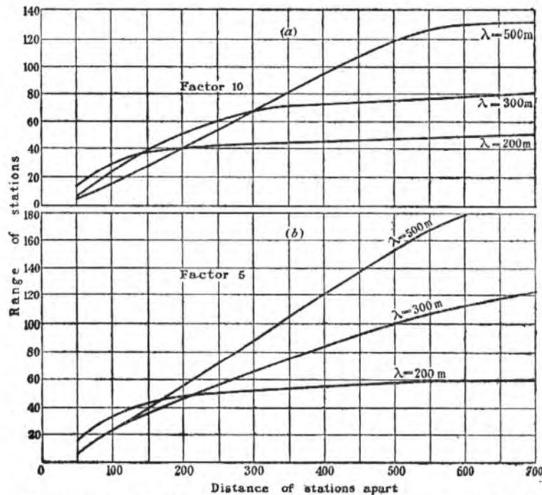
FIG. 14.—Range of two equal power stations sharing same wavelength, at different distances apart and different factors.
