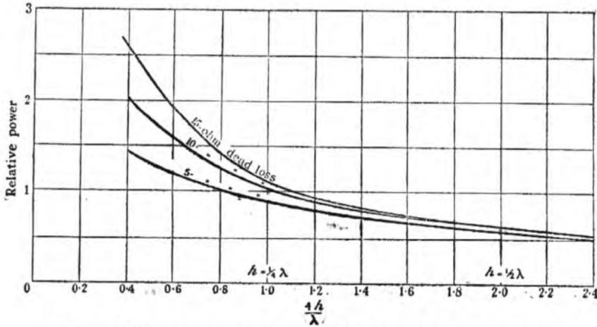
FIG. 9.—Relative power required to produce a given value of metre-amperes.
