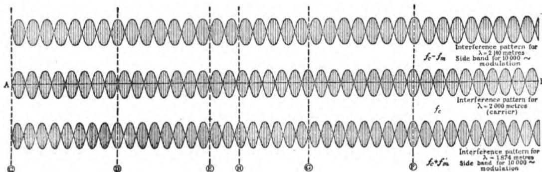
FIG. 12.—Interference pattern produced by two broadcasting stations using the same wavelength of 2,000 m. and having the same modulation of 10,000 cycles per sec.
