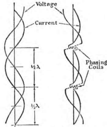
FIG. 7.—Current and voltage in a long uniform aerial.
