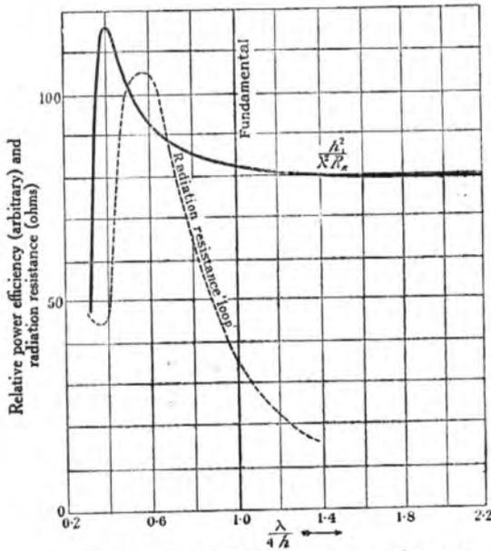
FIG. 6.—Ordinate (thick curve) represents  $h_1^2/(\lambda^2 R_R)$ .
