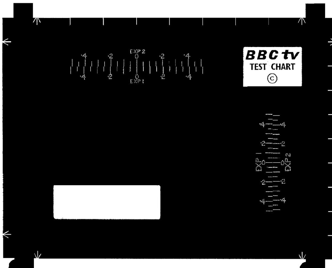
Fig. 11 — Hop and weave tests
